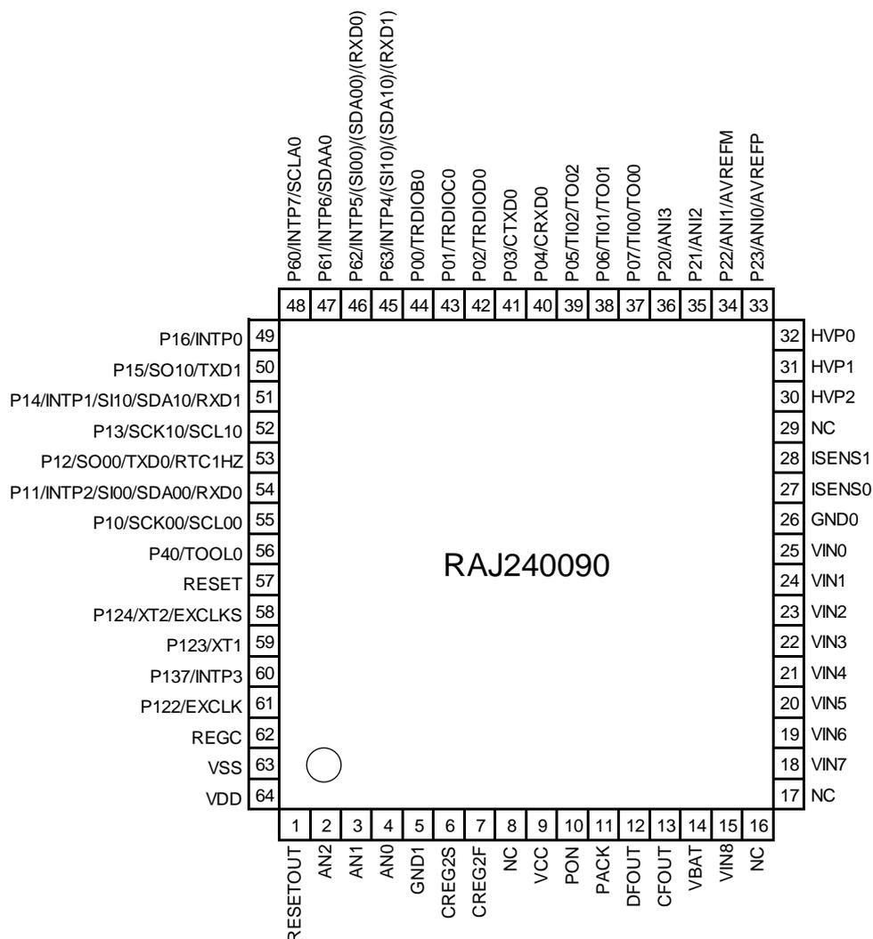
**Caution 1.** REGC pin connects to VSS pin through a capacitor (0.47 to 1 μF)
