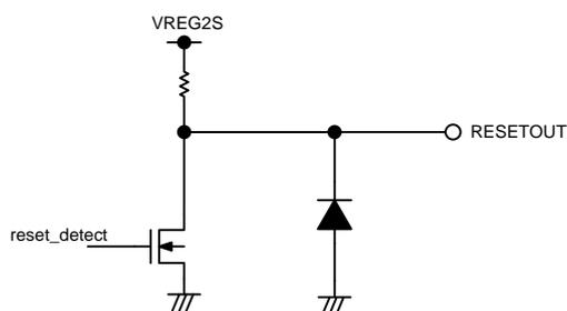
Figure 3-21 Pin Block Diagram for RESETOUT Pin
