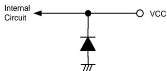
**Figure 3-12 Pin Block Diagram for VCC Pin**
