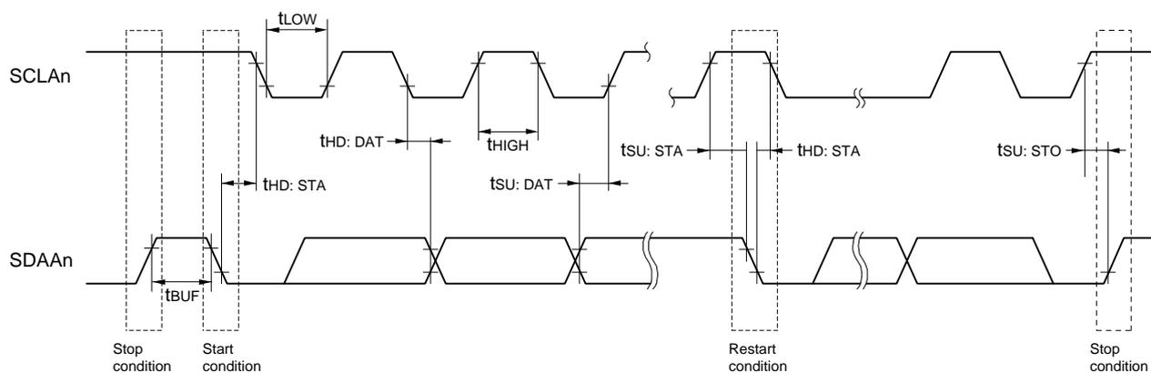
I<sup>2</sup>C serial transfer timing
