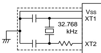
**Figure 3-1 Example of External Circuit for XT1 Oscillator**
