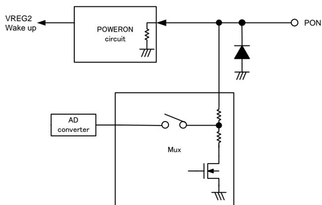
Figure 3-15 Pin Block Diagram for PON Pin
