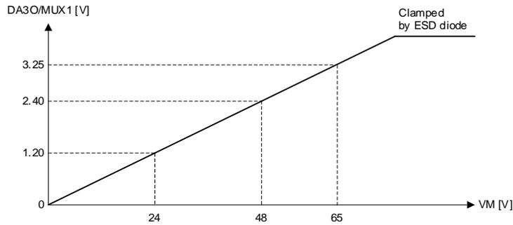
Figure 6.5-6 The Relation Between DA30/MUX1 and VM Voltage
