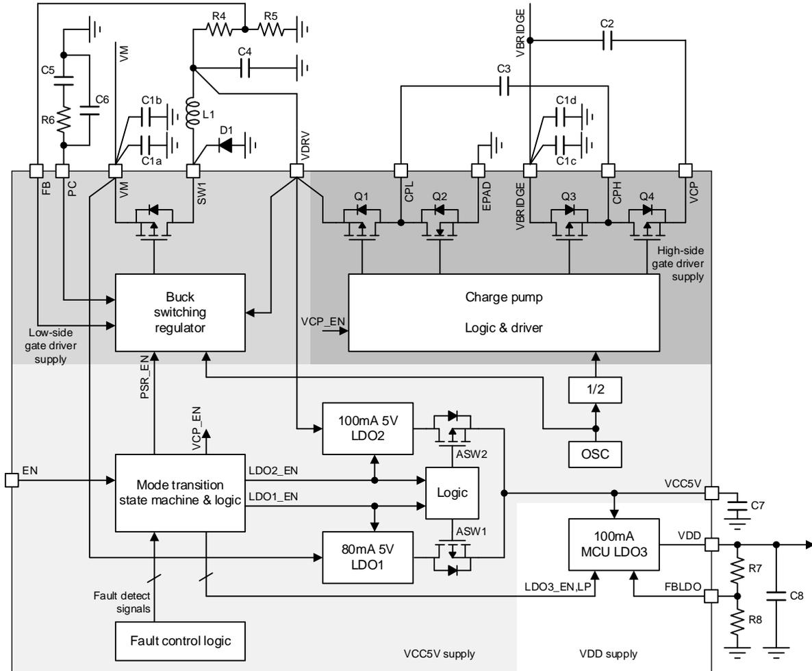
Figure 6.3-1 Block Diagram of Power Supply Blocks
