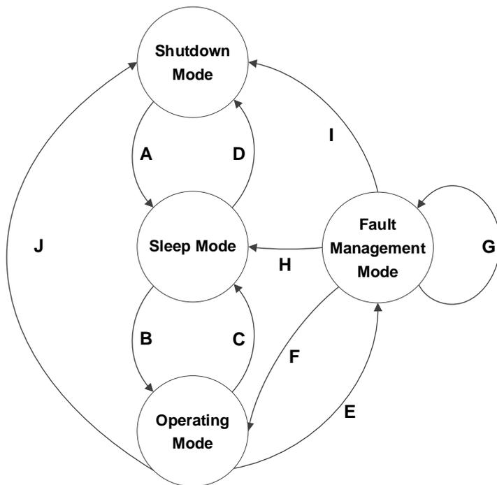
Figure 6.1-2 Mode Transition State Machine
