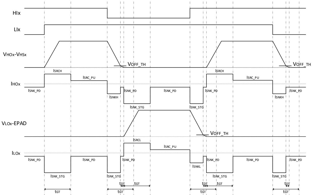
Figure 6.4-6 Gate Drive Timing Diagram in 3-Phase PWM Mode
