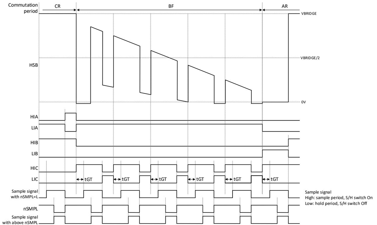
Figure 6.5-4 S/H Timing During Commutation Period BF
