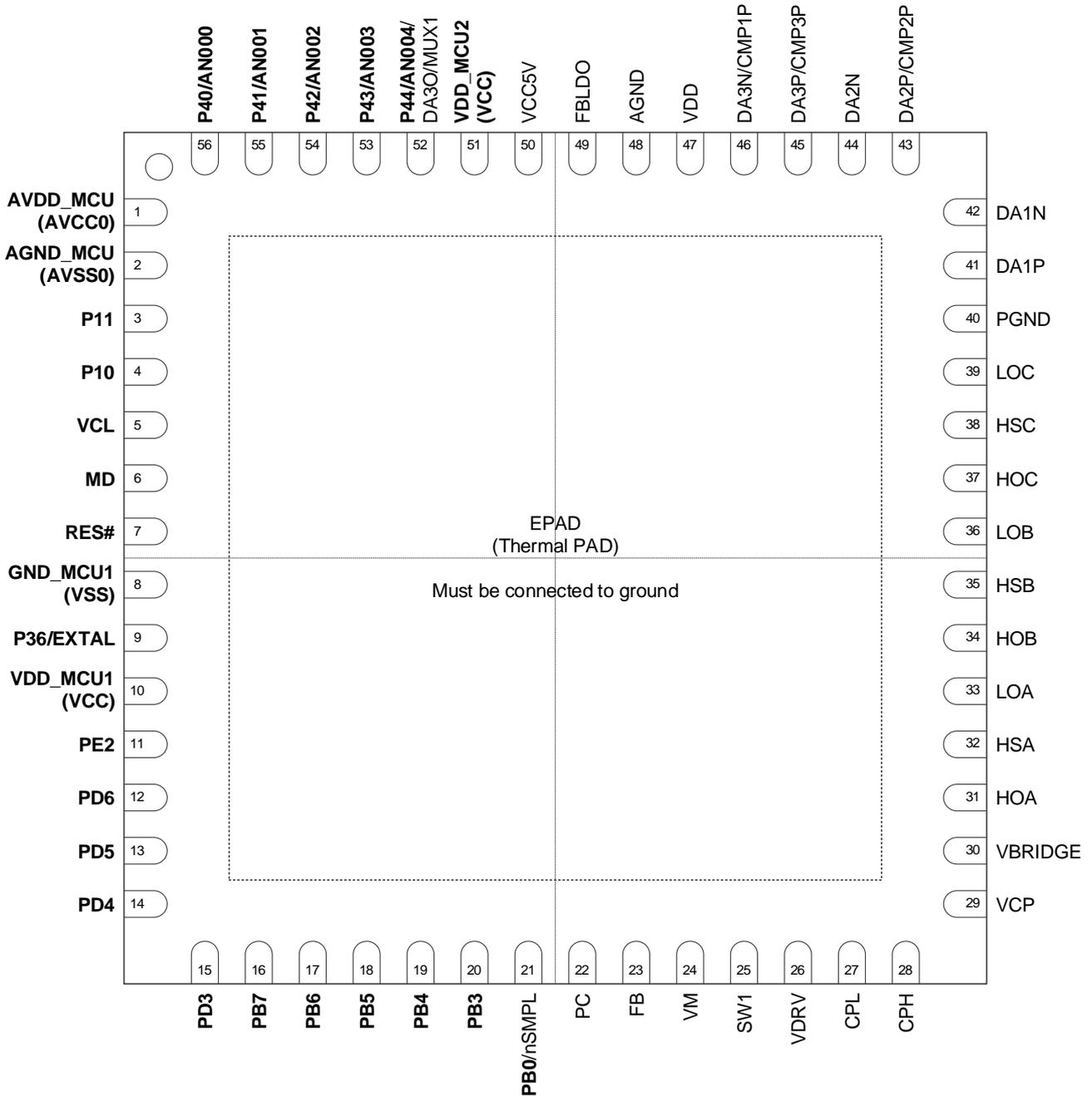
Figure 4.2-1 Pin Configuration Diagram (Top View)
