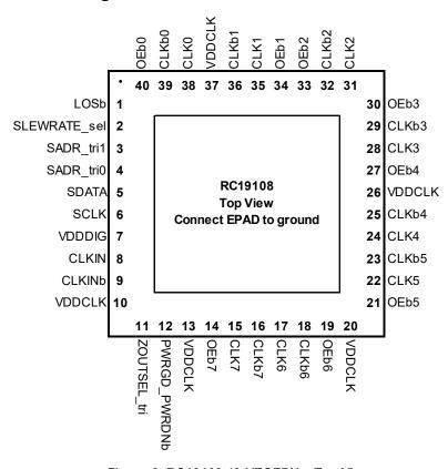
Figure 2. RC19108 40-VFQFPN - Top View
