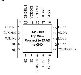
Figure 6. RC19102 20-VFQFPN - Top View
