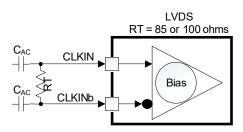
Figure 13. LVDS Input Levels
