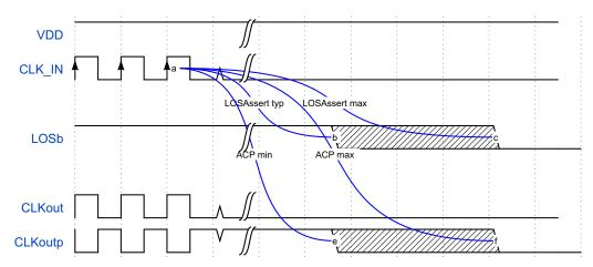
Figure 21. LOSb Assert Timing
