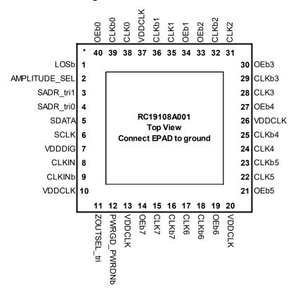
Figure 3. RC19108 40-VFQFPN - Top View
