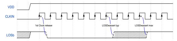
Figure 20. LOSb De-assert Timing RC191xx Devices
