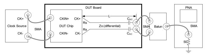
Figure 11. Test Load for PCle Phase Jitter Measurements
