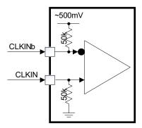
Figure 7. Clock Input Bias Network
