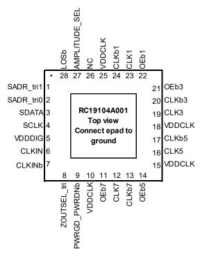
Figure 5. RC19104A100 28-VFQFPN - Top View
