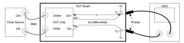
Figure 9. AC/DC Test Load for Differential Outputs (Standard PCle Source-Terminated)
