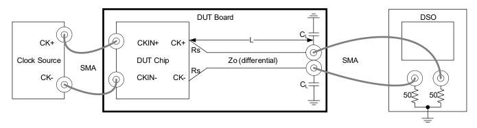
Figure 10. AC/DC Test Load for Differential Outputs (Double-Terminated or Receiver-Terminated)
