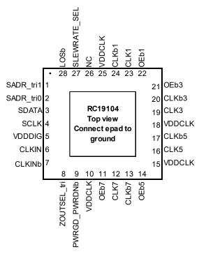
Figure 4. RC19104 28-VFQFPN - Top View
