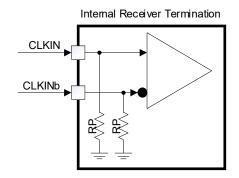
Figure 15. Receiver Termination
