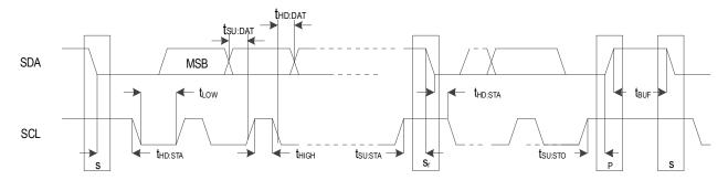
Figure 8. SMBus Target Timing Diagram
