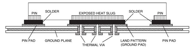
Figure 14. P.C. Assembly for Exposed Pad Thermal Release Path - Side View
