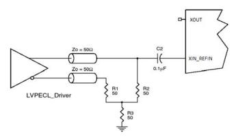
Figure 8. LVPECL Driver to XTAL Input Interface
