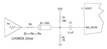
Figure 7. LVCMOS Driver to XTAL Input Interface
