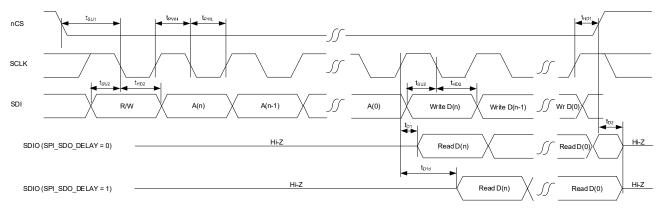
Figure 3. SPI Bus Timing
