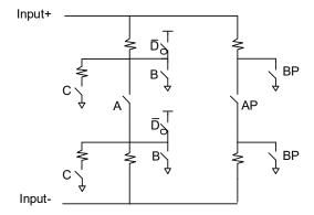
Figure 4. Programmable Input Buffer Logical Diagram
