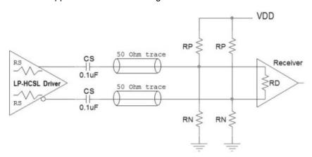
Figure 11. AC-Coupling Termination
