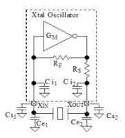
Figure 12. Crystal Load Capacity
