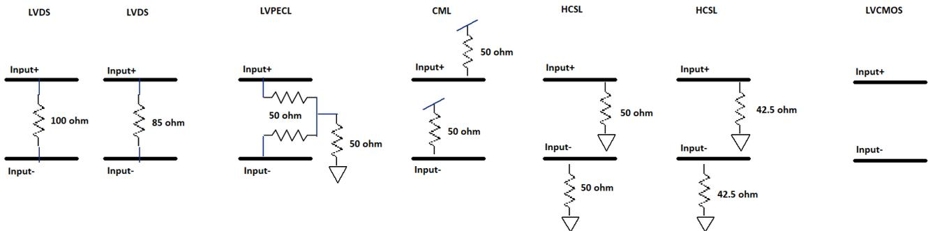
Figure 6. Input Buffer Behavior by Protocol
