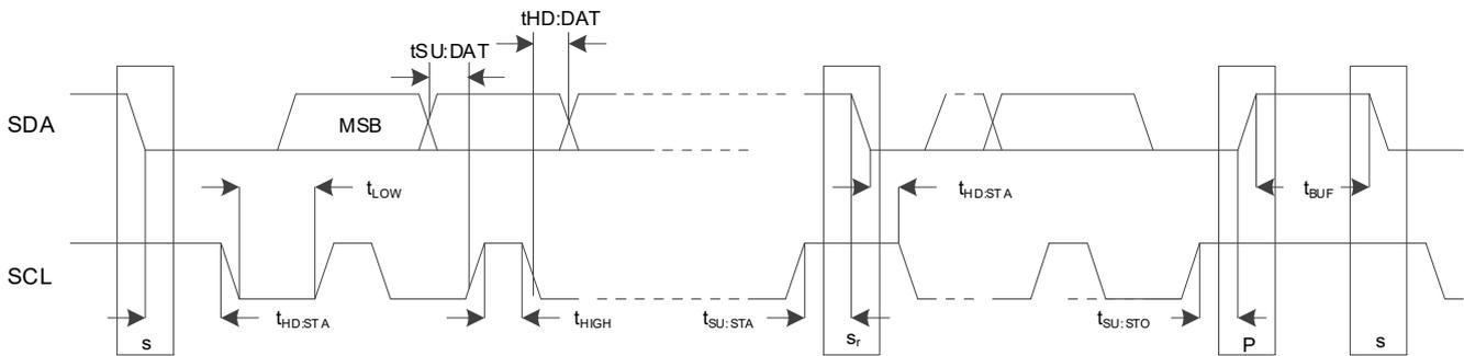
Figure 3. I<sup>2</sup>C/SMBus Target Timing Diagram
