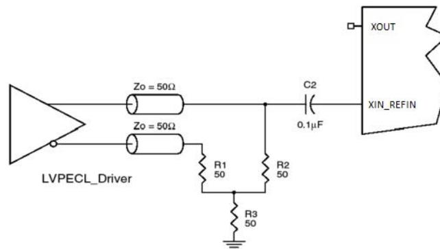
Figure 9. LVPECL Driver to XTAL Input Interface
