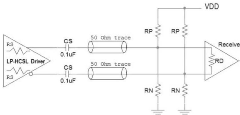
Figure 12. AC-Coupling Termination
