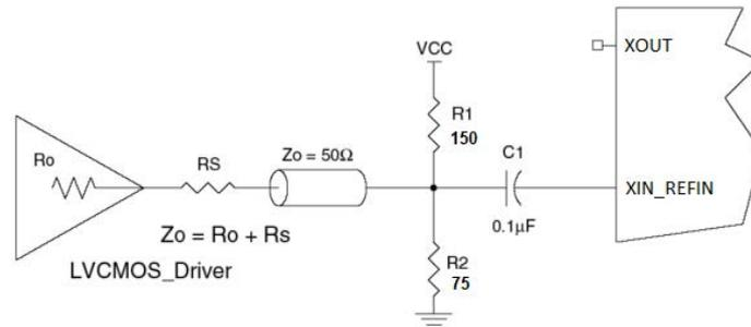
Figure 8. LVCMOS Driver to XTAL Input Interface
