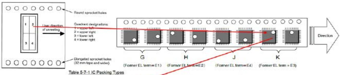
Figure 16. Pin 1 Orientation in Tape and Reel Packaging
