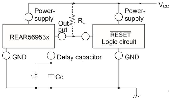
(b) Reset at transistor ON
