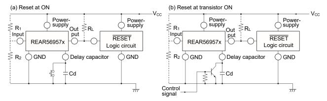
Case of Using Reset Signal except Supply Voltage in the REAR56957
