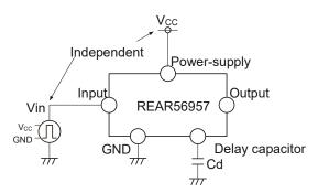
Example 2. Logic pulse input (not recommended)
