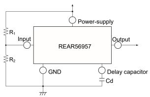
Delay Waveform Generating Circuit
