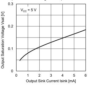
Output Load Current vs. Output Voltage (REAR56957A)
