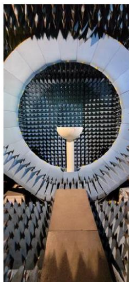
Figure 19. Satimo SG-23 6 GHz Stargate Antenna Test Chamber
