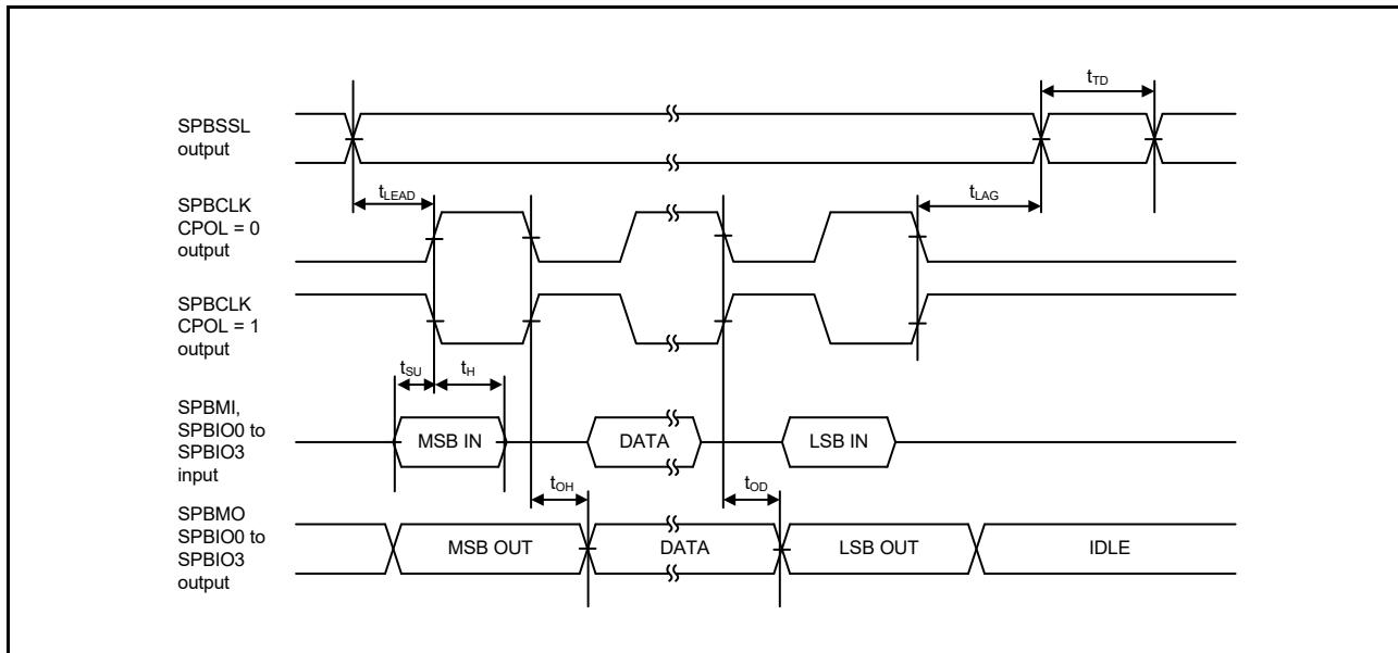
Figure 2.58 SPIBSC Transmit/Receive Timing (CPHAT = 0, CPHAR = 0)
