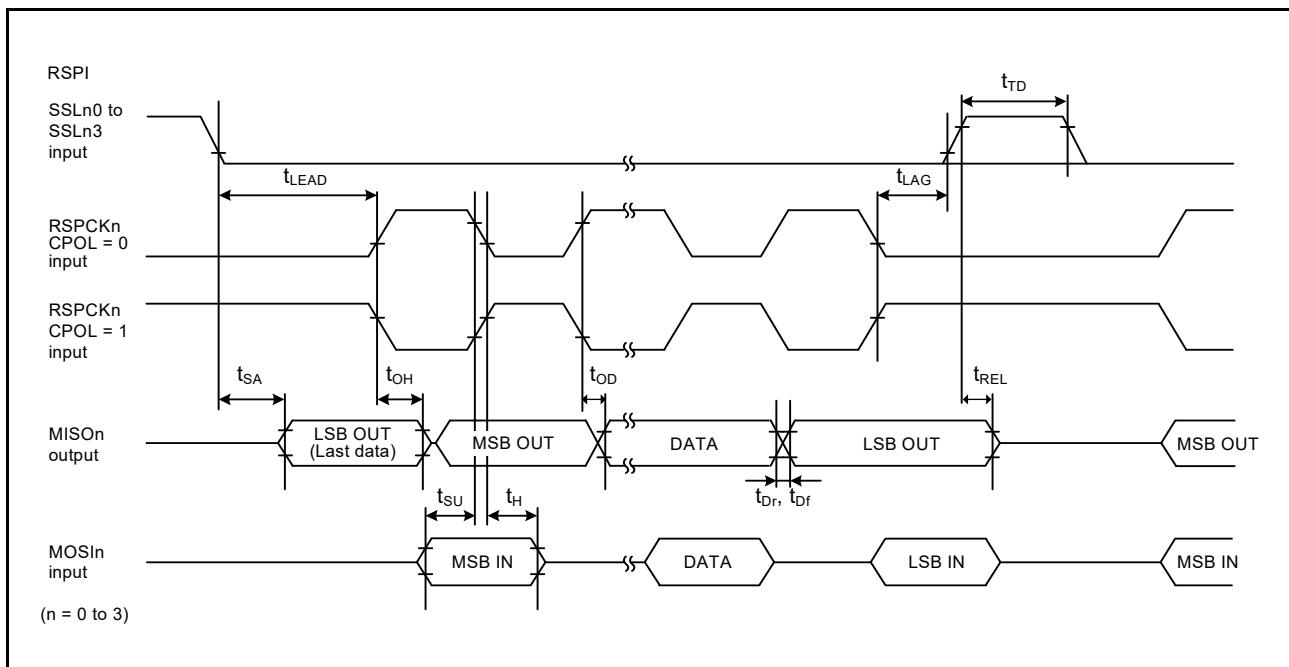
Figure 2.56 RSPI Timing (Slave, CPHA = 1)
