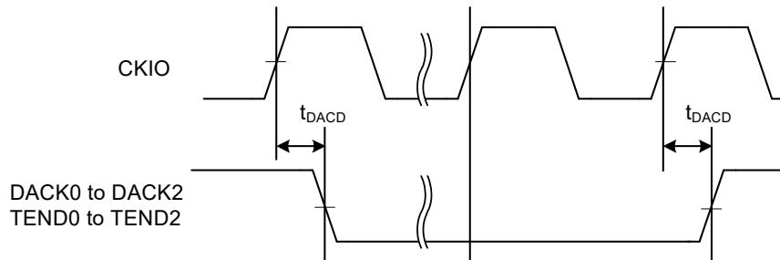
**Figure 2.38 DACK and TEND Output Timing**
