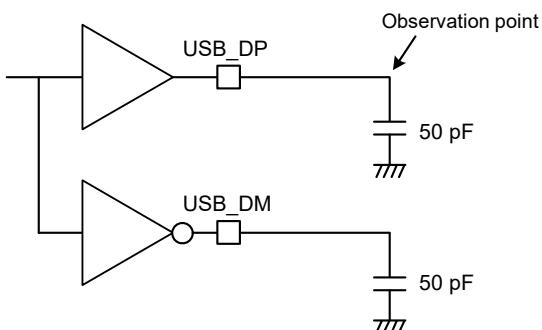
**Figure 2.83 Measurement Circuit (Full Speed)**
