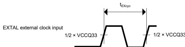
**Figure 2.5 EXTAL External Clock Input Timing****Table 2.14 XTAL Clock Timing**
