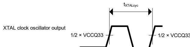
**Figure 2.6 XTAL Clock Oscillator Output Timing****Table 2.15 LOCO Clock Timing**
