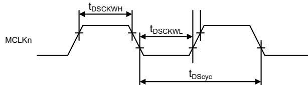
**Figure 2.79 Clock Input/Output Timing**
