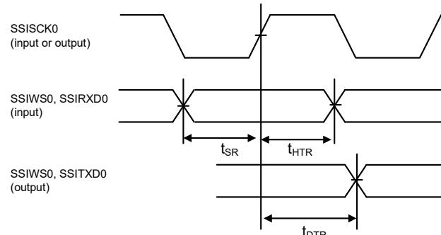
Figure 2.66 Transmit/Receive Timing (SSISCK0 Rising Synchronous)
