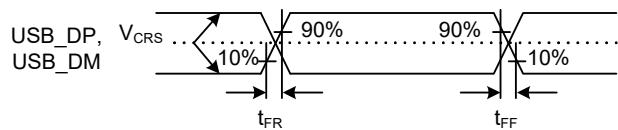
**Figure 2.82 USB\_DP, USB\_DM Output Timing (Full Speed)**
