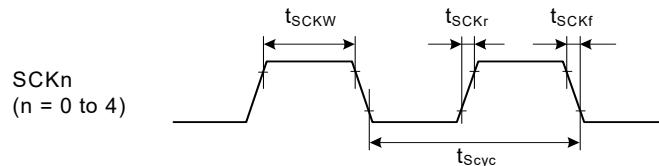
**Figure 2.50 SCK Clock Input Timing**
