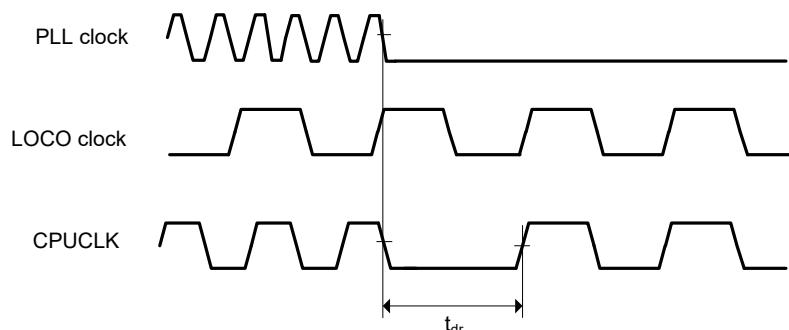
**Figure 2.86 Oscillation Stop Detection Timing**
