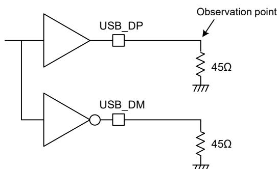
**Figure 2.85 Measurement Circuit (High Speed)**
