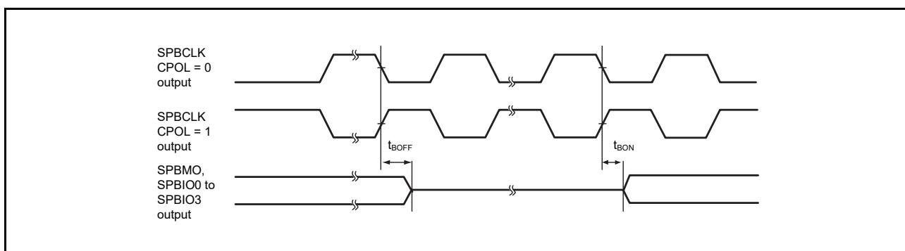
Figure 2.61 SPIBSC Buffer On/Off Timing (CPHAT = 0, CPHAR = 0)
