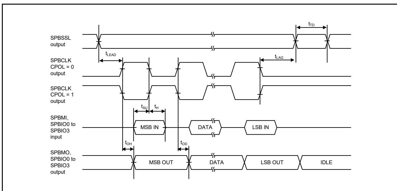
Figure 2.59 SPIBSC Transmit/Receive Timing (CPHAT = 1, CPHAR = 1)
