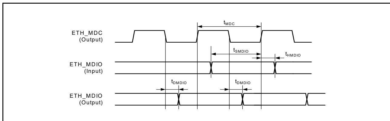
**Figure 2.78 Serial Management Access Timing**
