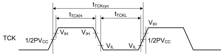
**Figure 2.87 TCK Input Timing**
