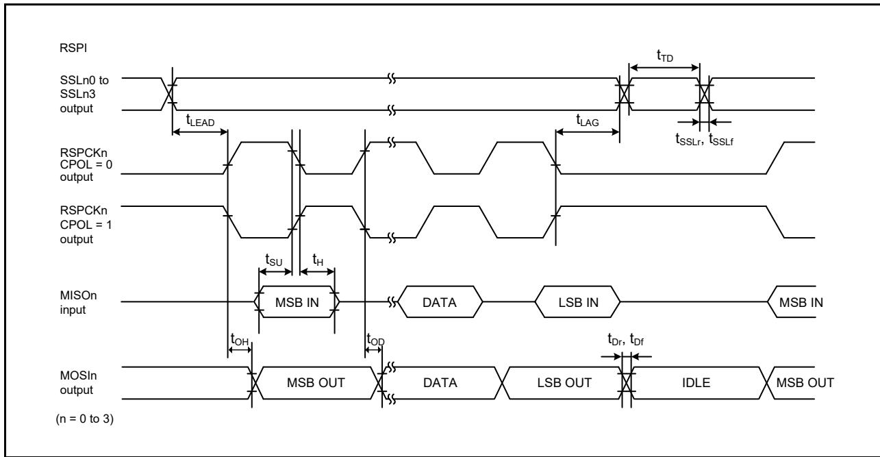
Figure 2.54 RSPIa Timing (Master, CPHA = 1)
