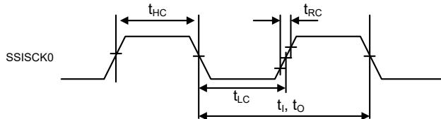
Figure 2.65 Clock Input/Output Timing
