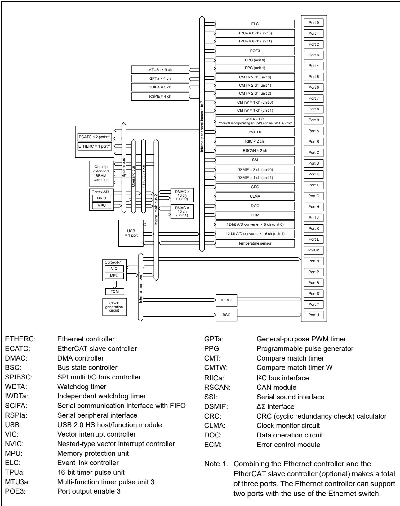
Figure 1.1 Block Diagram
