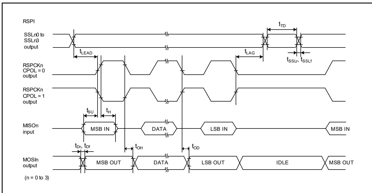
Figure 2.53 RSPIa Timing (Master, CPHA = 0)
