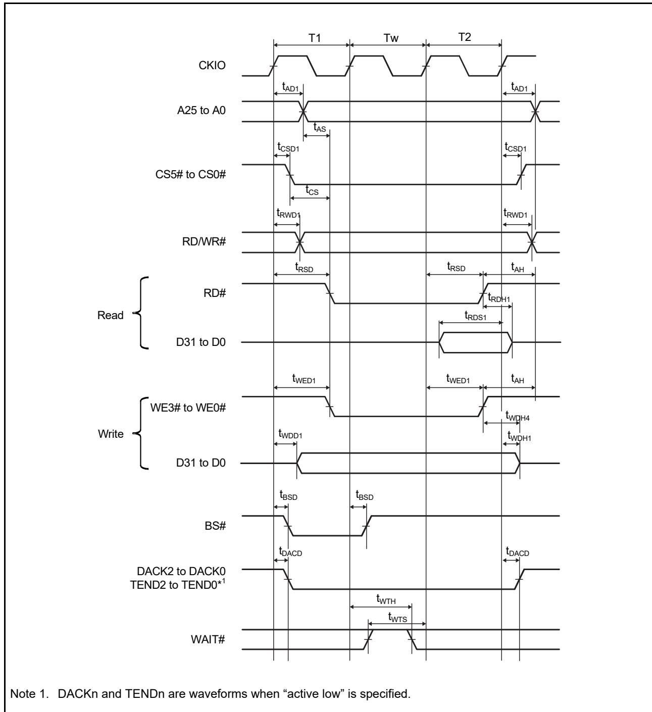
Figure 2.13 SRAM Interface Basic Bus Cycle (Software Wait 1)
