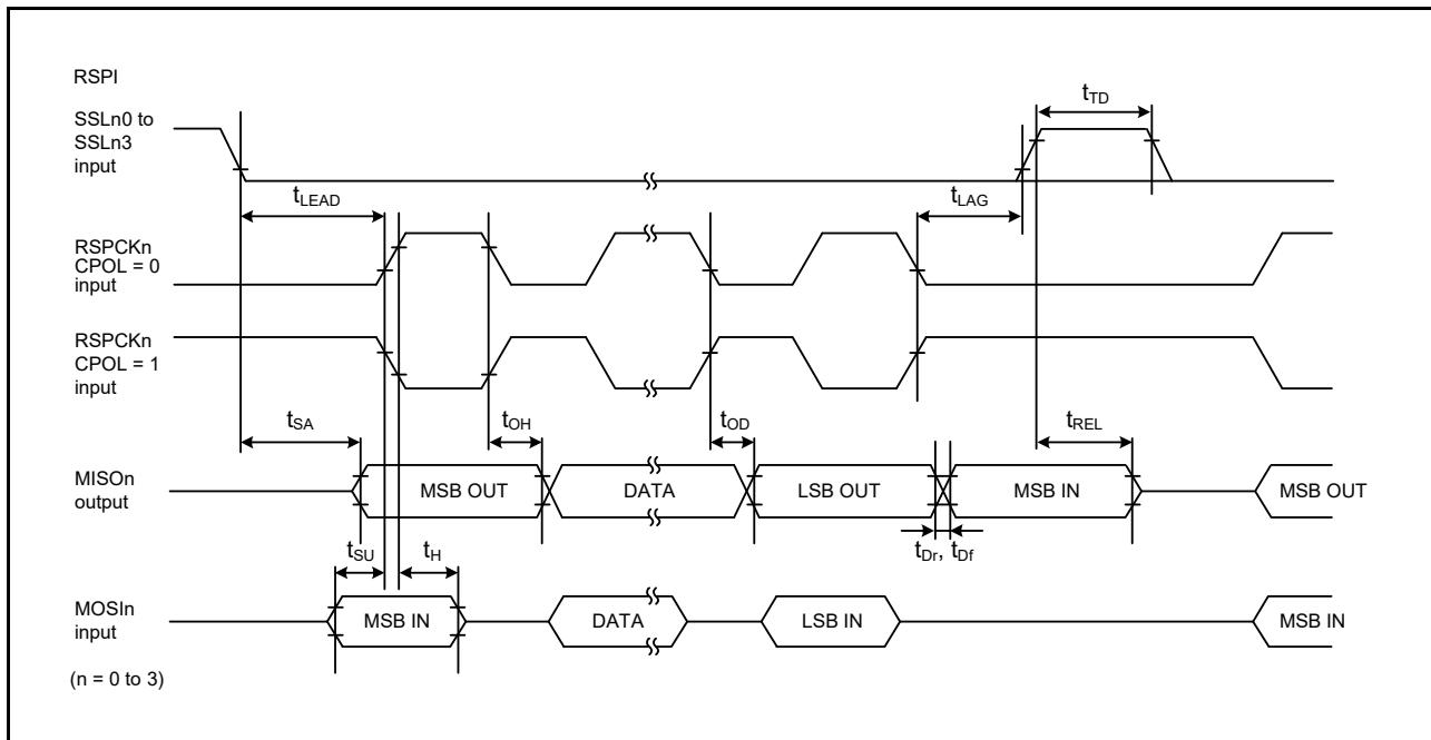
Figure 2.55 RSPI Timing (Slave, CPHA = 0)
