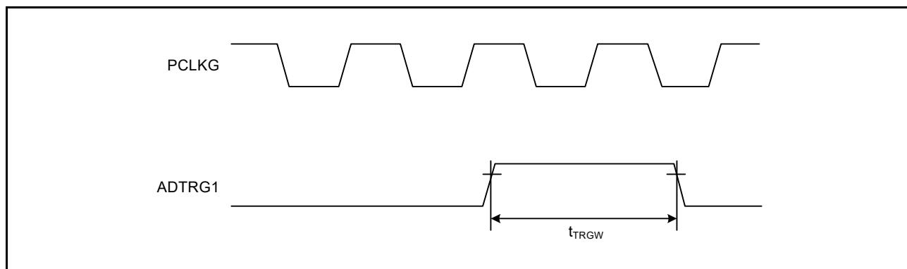
**Figure 2.49 A/D Converter Trigger Input Timing (ADTRG1)**
