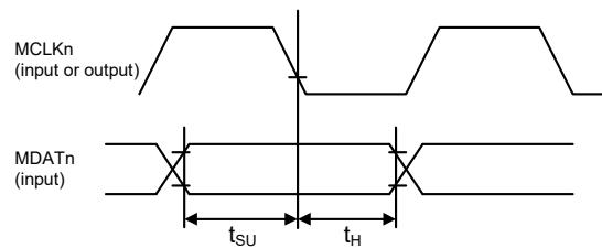
Figure 2.81 Reception Timing (MCLKn Falling Synchronous)
