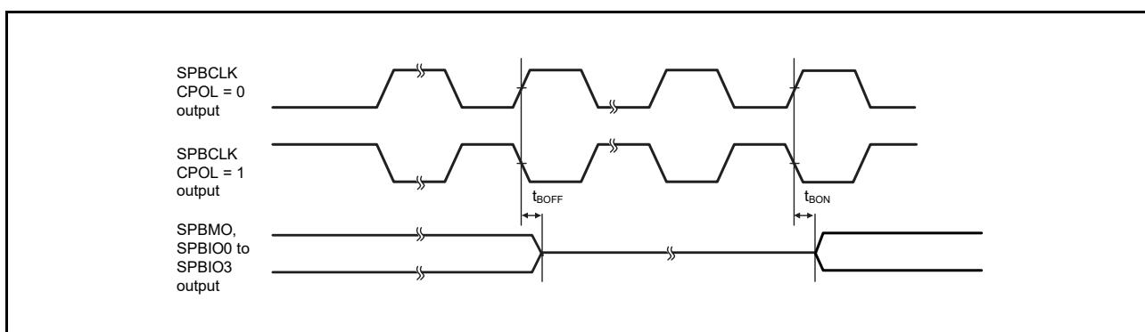
Figure 2.62 SPIBSC Buffer On/Off Timing (CPHAT = 1, CPHAR = 1)
