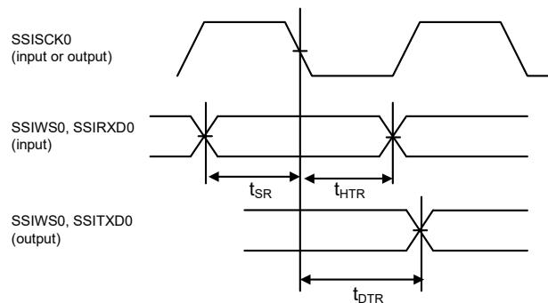
Figure 2.67 Transmit/Receive Timing (SSISCK0 Falling Synchronous)
