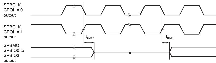
Figure 2.63 SPIBSC Buffer On/Off Timing (CPHAT = 0, CPHAR = 1)
