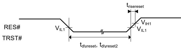
**Figure 2.8 Reset Input Timing**
