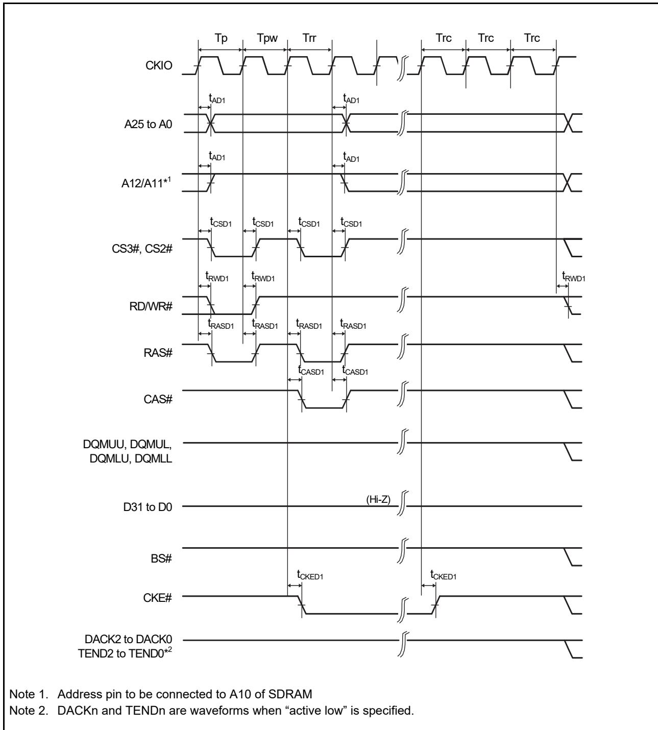
Figure 2.35 Synchronous DRAM Self-Refresh Timing (WTRP = 1 Cycle)
