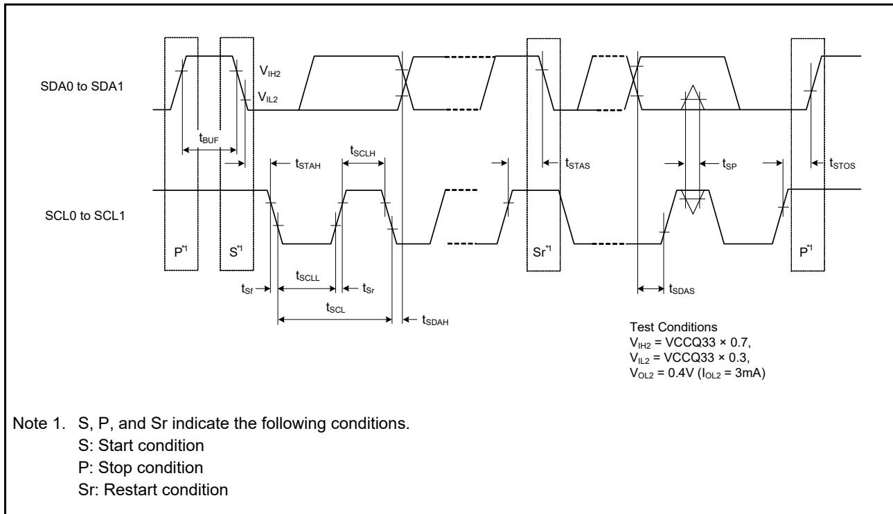
Figure 2.64 RII Ca Bus Interface Input/Output Timing
