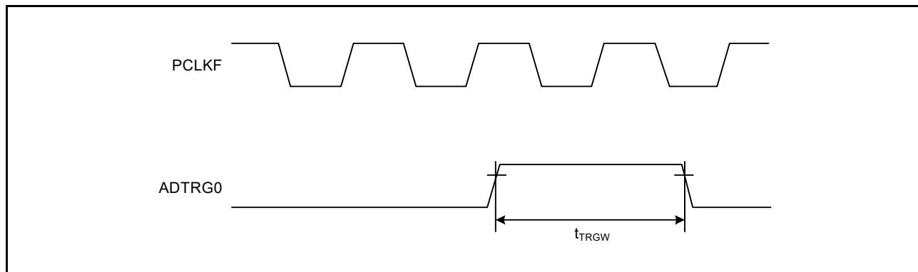
**Figure 2.48 A/D Converter Trigger Input Timing (ADTRG0)**
