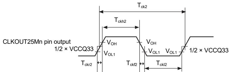
**Figure 2.4 CLKOUT25Mn Pin Output Timing 2**
