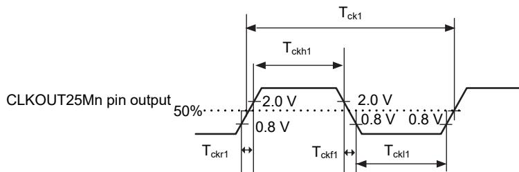
**Figure 2.3 CLKOUT25Mn Pin Output Timing 1**
