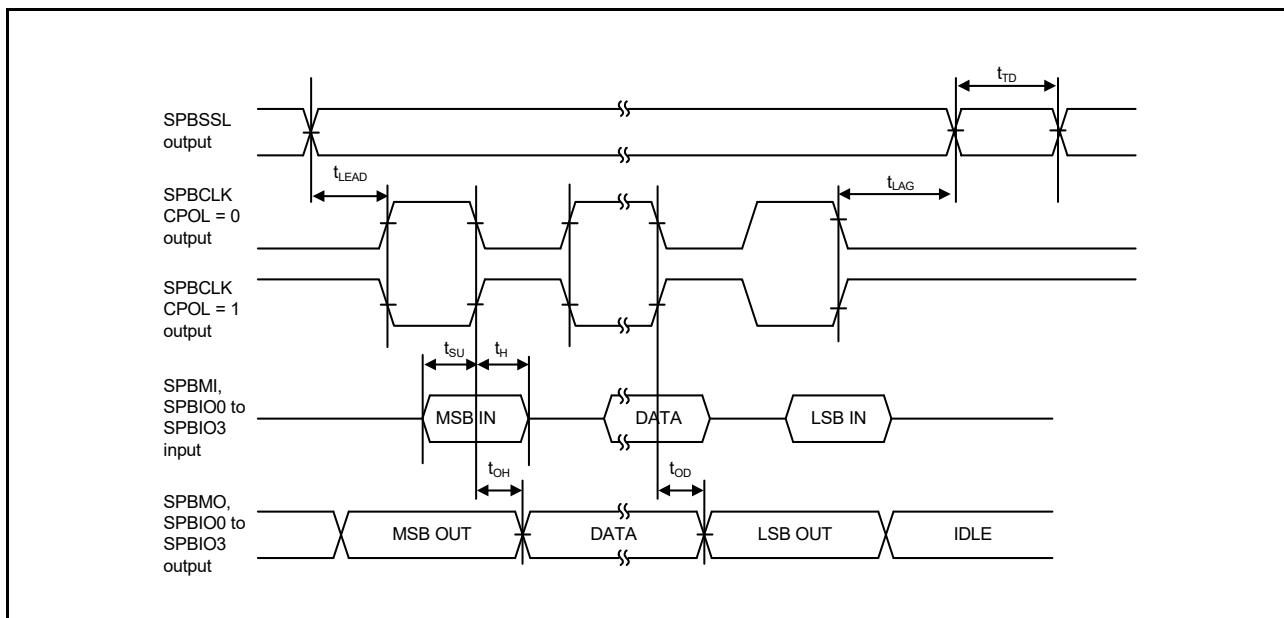
Figure 2.60 SPIBSC Transmit/Receive Timing (CPHAT = 0, CPHAR = 1)
