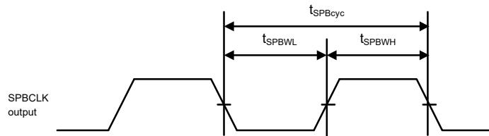
**Figure 2.57 SPIBSC Clock Timing**
