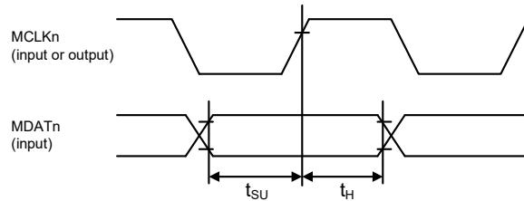
**Figure 2.80 Reception Timing (MCLKn Rising Synchronous)**
