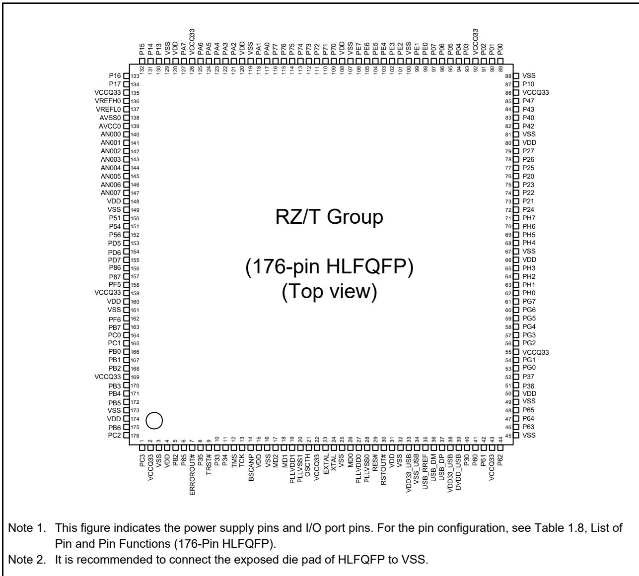
Note 1. This figure indicates the power supply pins and I/O port pins. For the pin configuration, see Table 1.8, List of Pin and Pin Functions (176-Pin HLFQFP).
