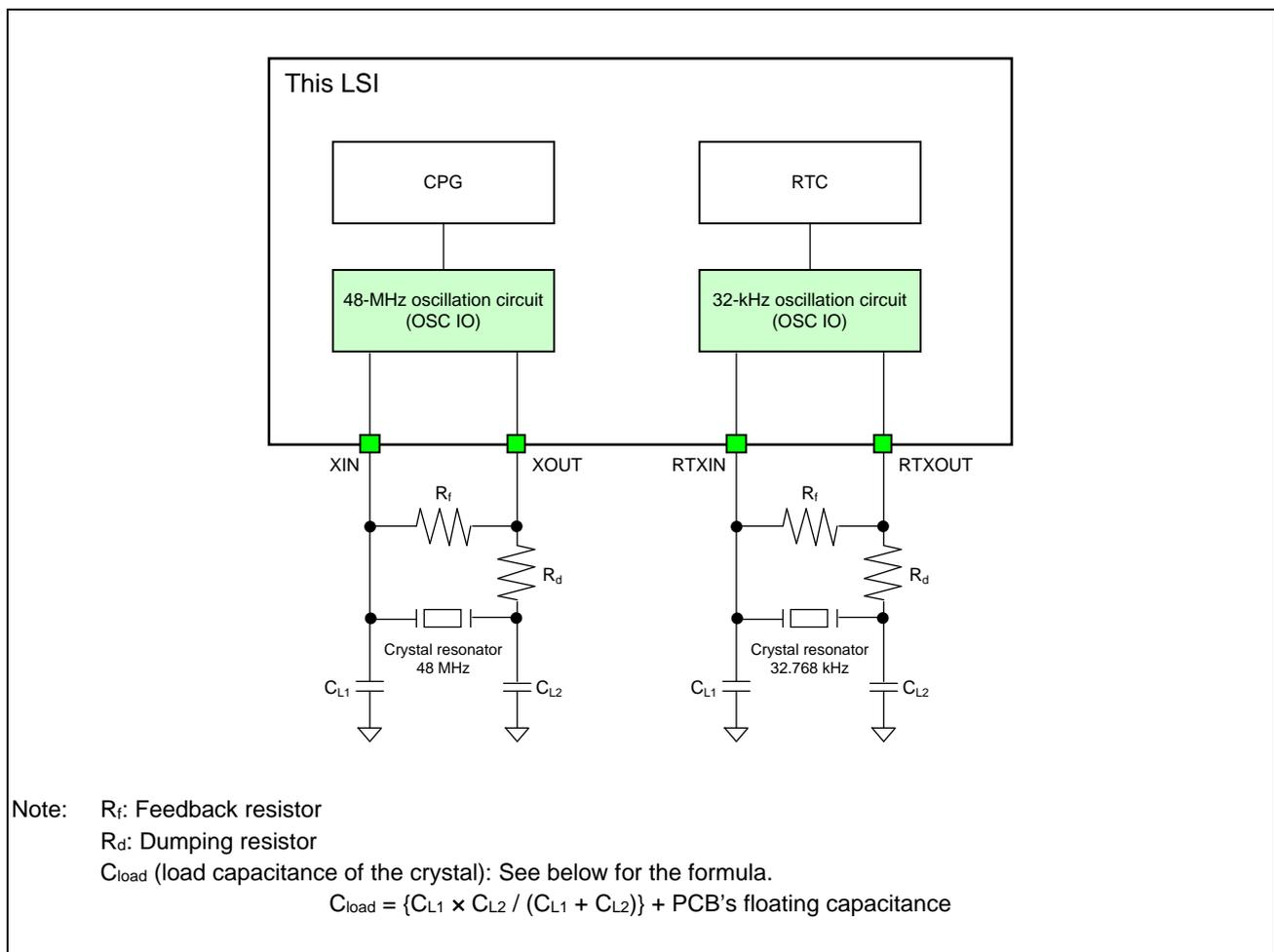
Figure 3.7-1 Example of Connections with Crystal Resonators
