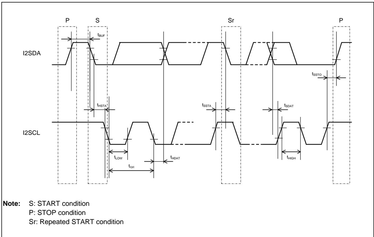
Figure 3.5-1 IIC Timing
