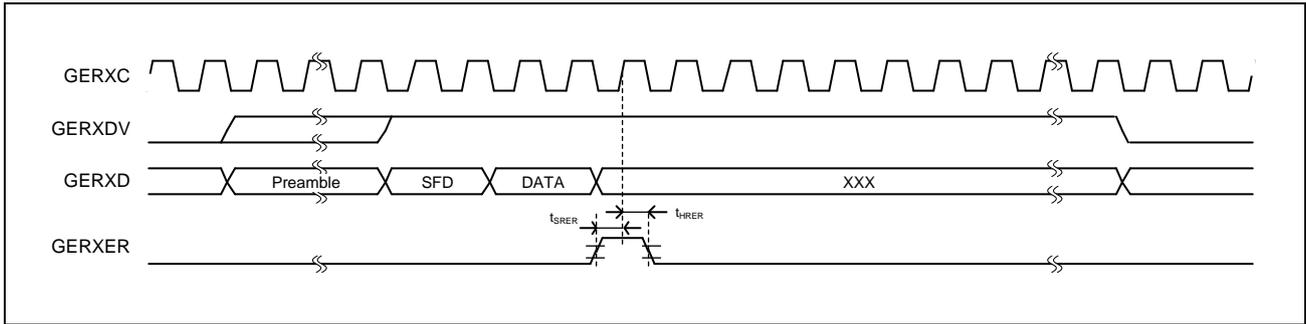
Figure 3.5-6 Reception Timing (in Cases of Error)
