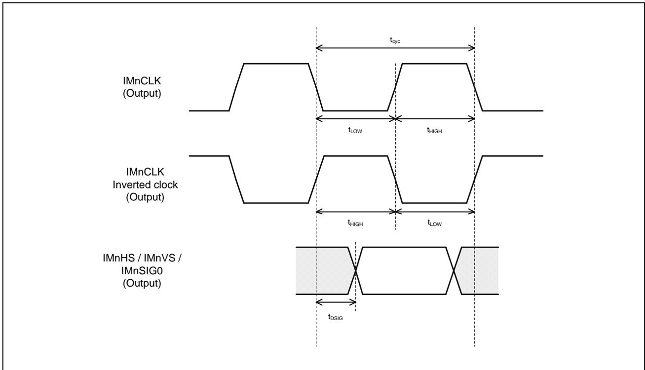
Figure 3.5-12 Clock Synchronous HS/VS/SIG0 Signal Output Timing
