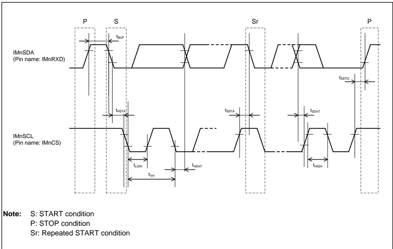
Figure 3.5-13 IIC Timing
