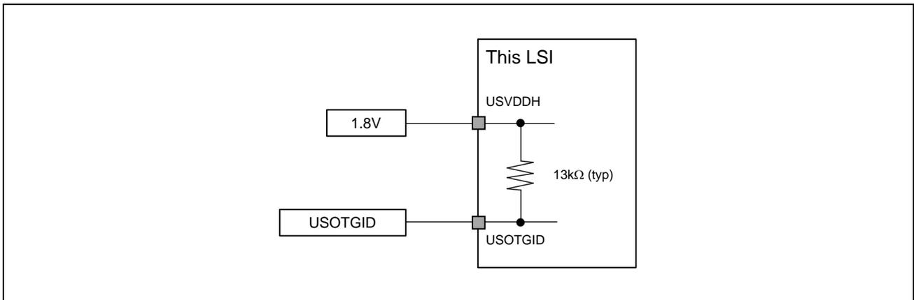
Note 5. When the power of this LSI is turned off, applying the 3.3-V pull-up voltage in the opposite direction to these pins does not cause any problem.
