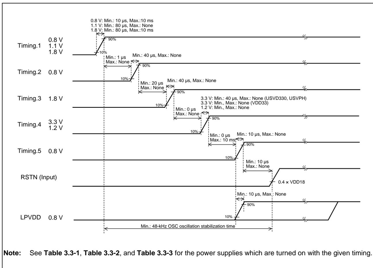
Figure 3.3-2 Power-On Sequence (other than for RTC/PWC)
