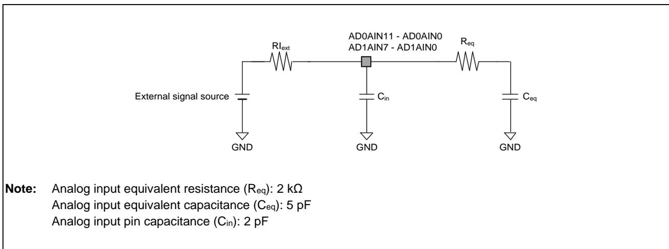
Figure 3.6-1 ADC Input Equivalent Circuit
