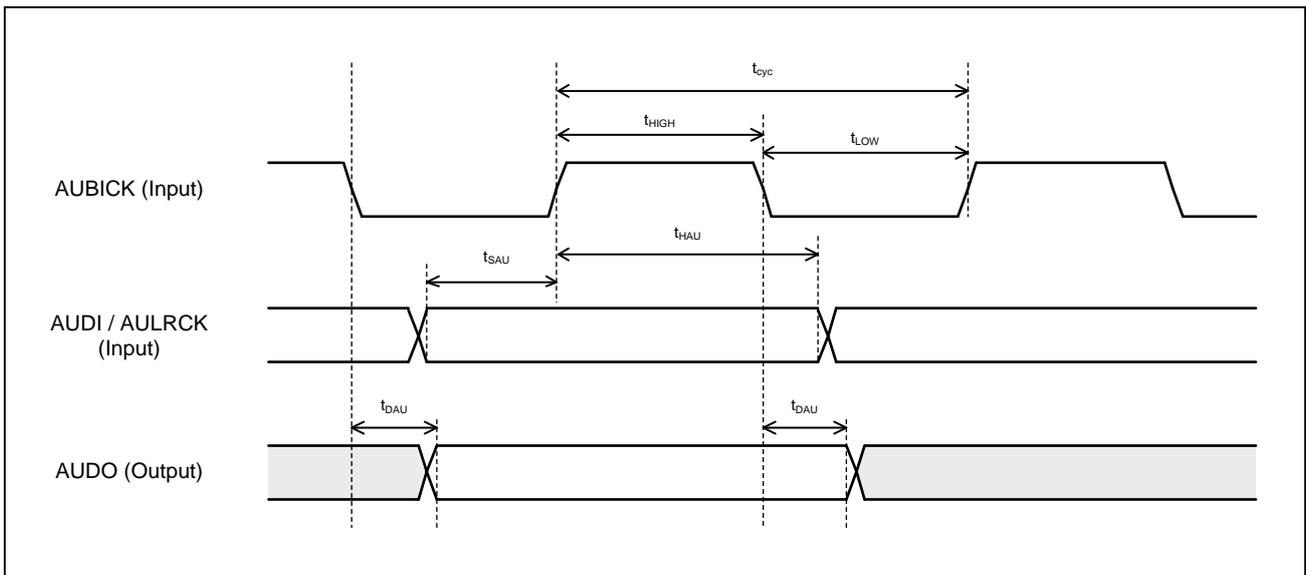
Figure 3.5-14 Audio Interface Timing
