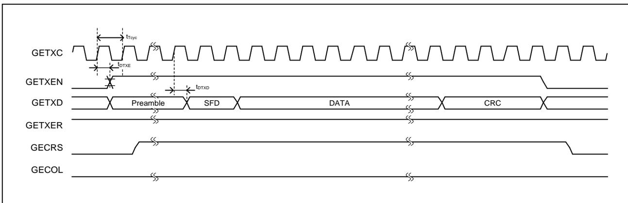
Figure 3.5-4 Transmission Timing
