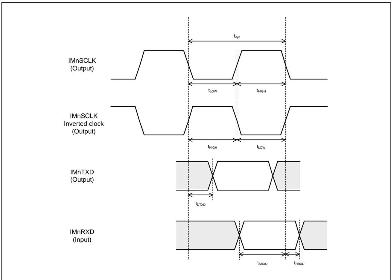
Figure 3.5-11 Clock Synchronous Serial Data I/O Timing
