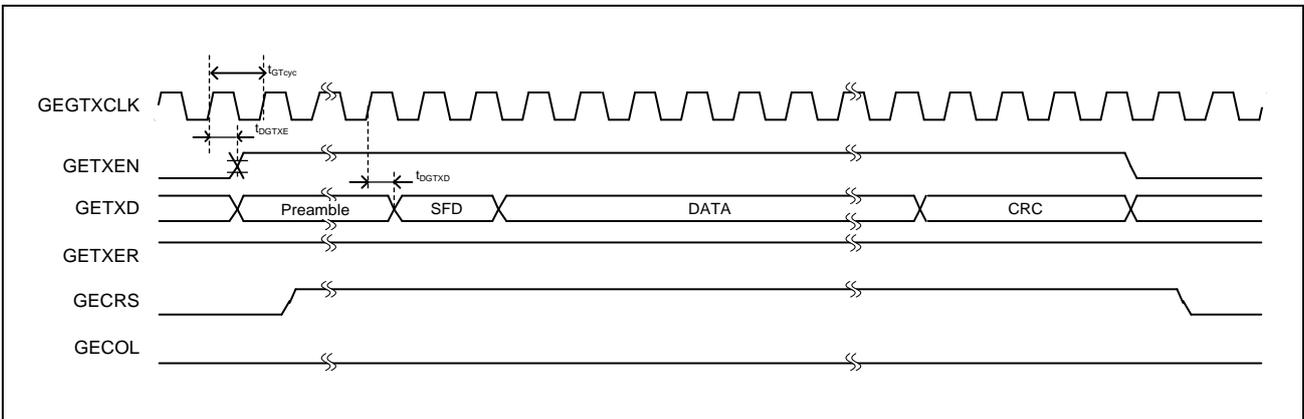
Figure 3.5-7 Transmission Timing
