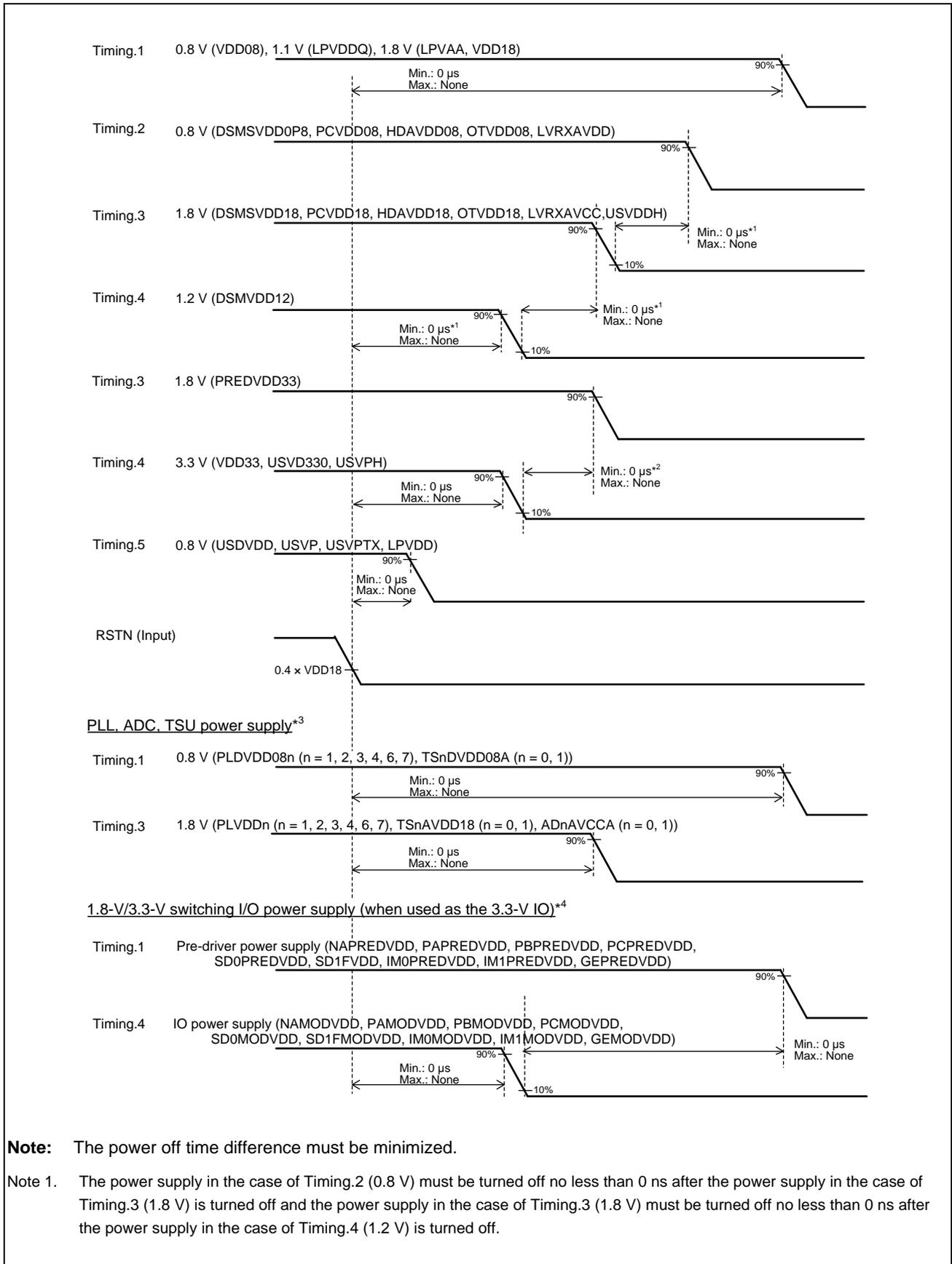
**Note:** The power off time difference must be minimized.
