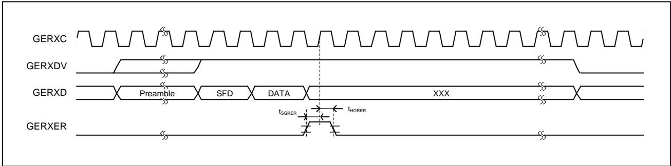
Figure 3.5-9 Reception Timing (in Cases of Error)
