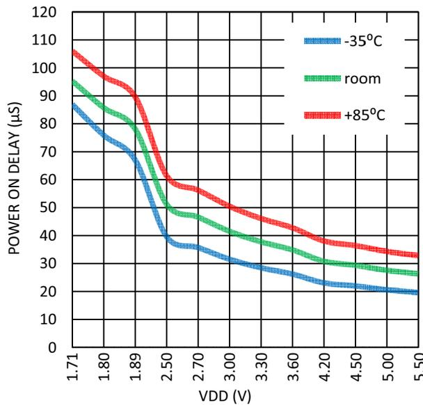
**Figure 24. Maximum Power On Delay vs. V<sub>DD</sub>.**
