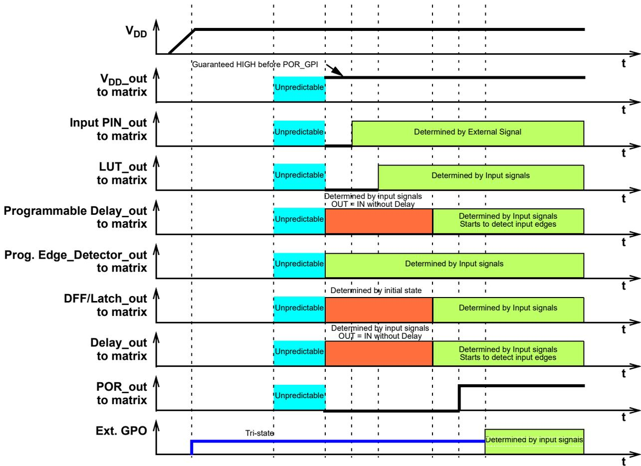
Figure 48. Internal Macrocell States during POR sequence
