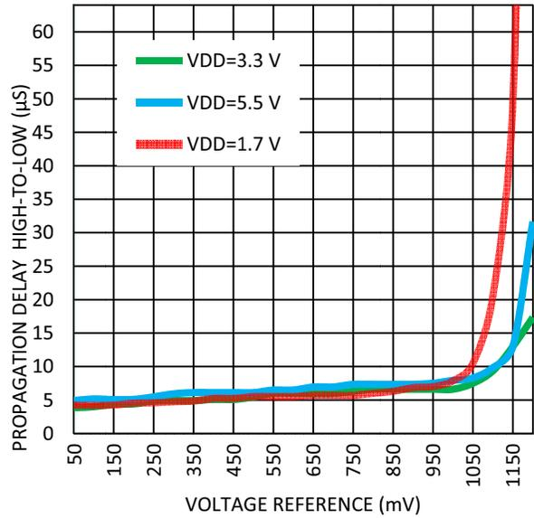
Figure 35. Maximum Propagation Delay High-to-Low vs. Voltage Reference at Room Temperature,  $V_{od} = 2 \text{ mV}$ .
