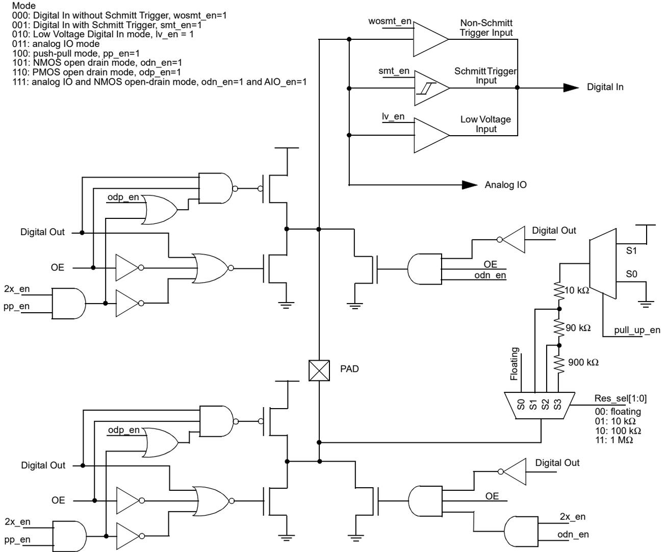
Figure 4. Register OE IO Structure Diagram
