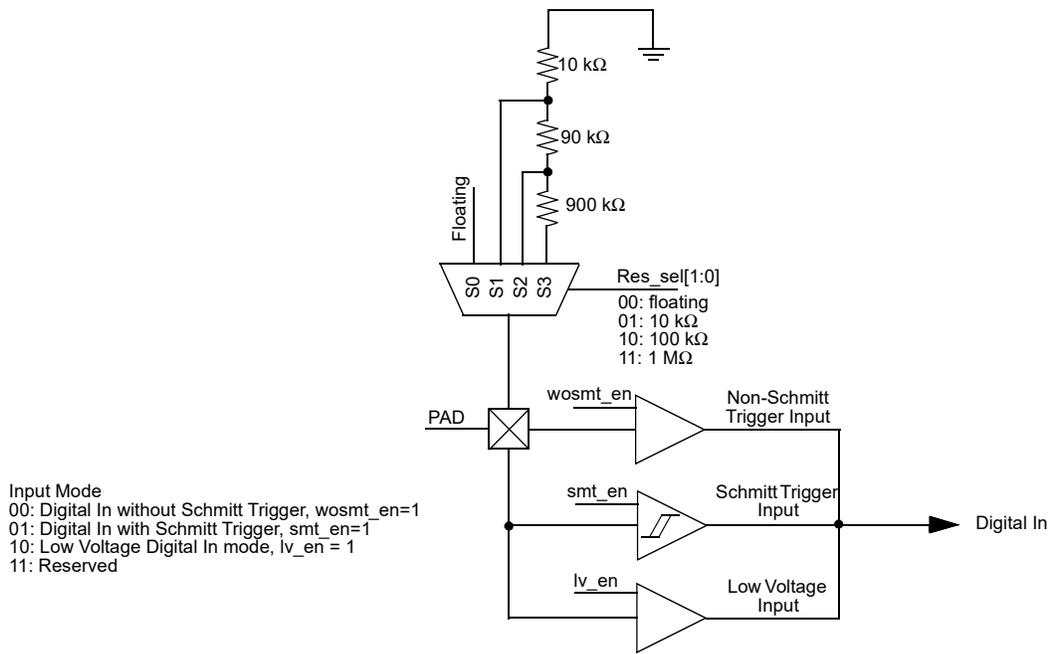
Figure 2. PIN 2 GPI IO Structure Diagram
