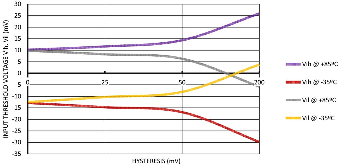
Figure 31. Input Threshold Voltage Vih, Vil vs. Hysteresis at V<sub>DD</sub> = 5.5 V, V<sub>ref</sub> = 1000 mV. Gain = 1
