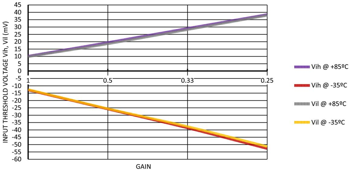
Figure 32. Input Threshold Voltage Vih, Vil vs. Gain at Hysteresis = 0, V<sub>DD</sub> = 5.5 V, V<sub>ref</sub> = 1000 mV
