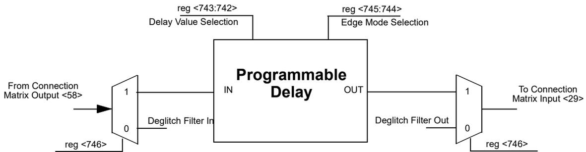
Figure 20. Programmable Delay
