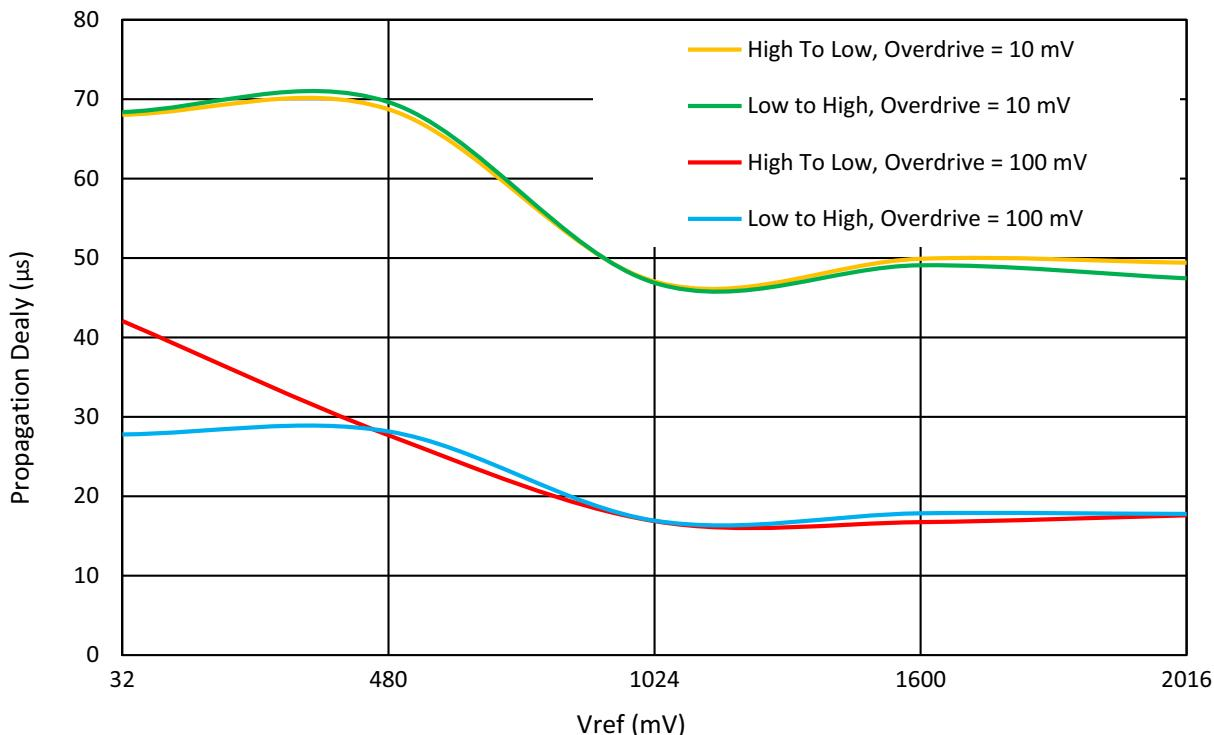
Figure 57: Typical Propagation Delay vs. Vref for ACMPxL at  $T = 25^\circ\text{C}$ ,  $V_{\text{DD}} = 2.3\text{ V to }5.5\text{ V}$ , Gain = 1, Hysteresis = 0
