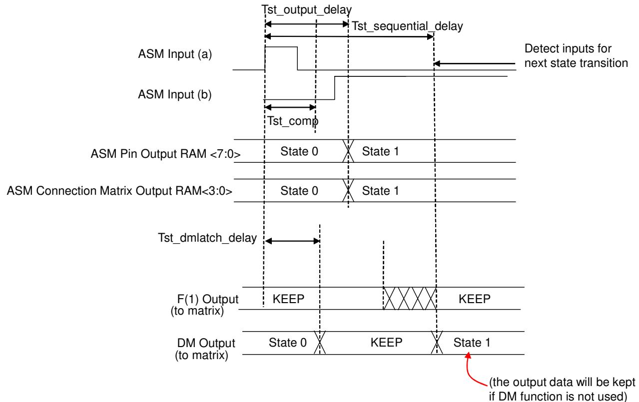
Figure 102: State Transition Timing - Competing Inputs Determinable
