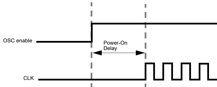
**Figure 77: Oscillator Startup Diagram**
