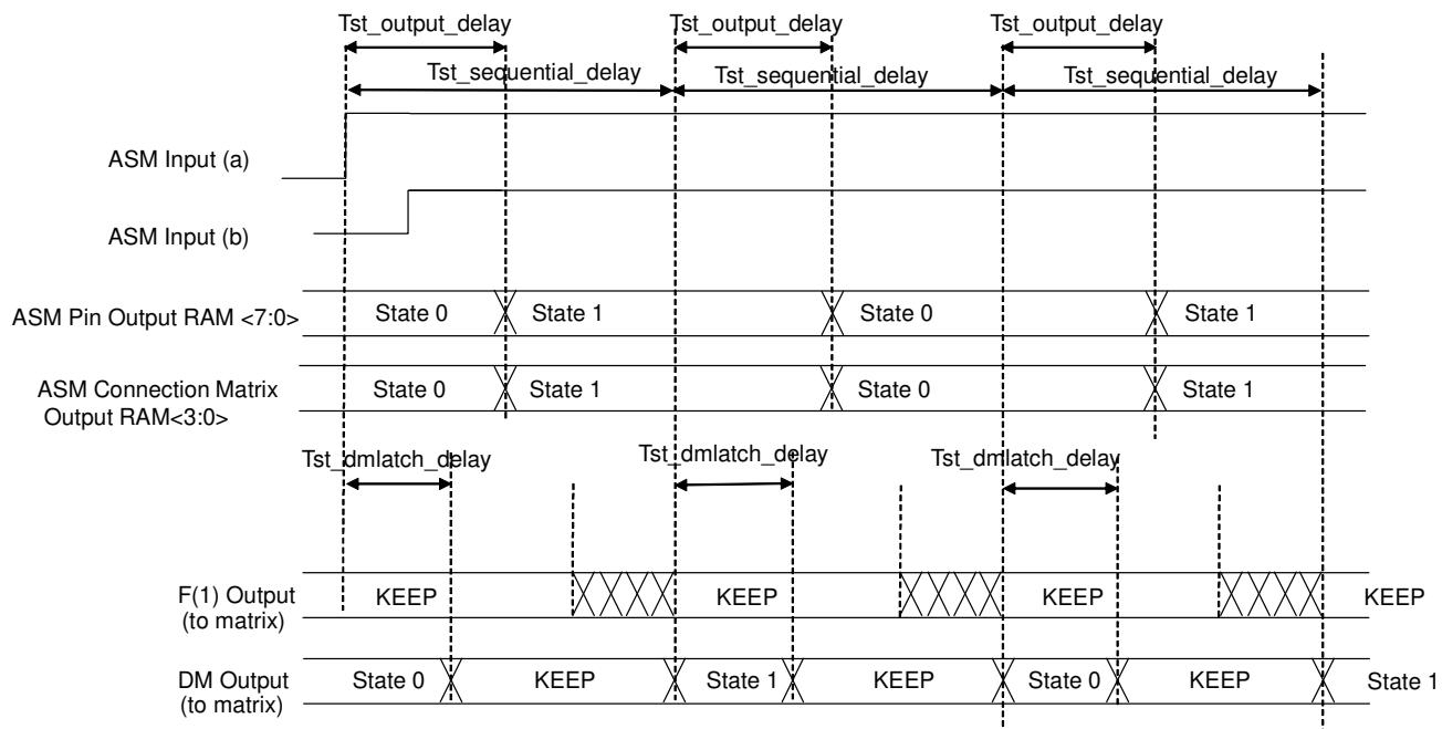
Figure 106: State Transition - Closed Cycling Timing
