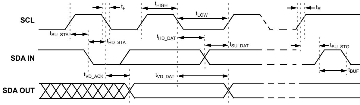
Figure 126: I<sup>2</sup>C General Timing Characteristics
