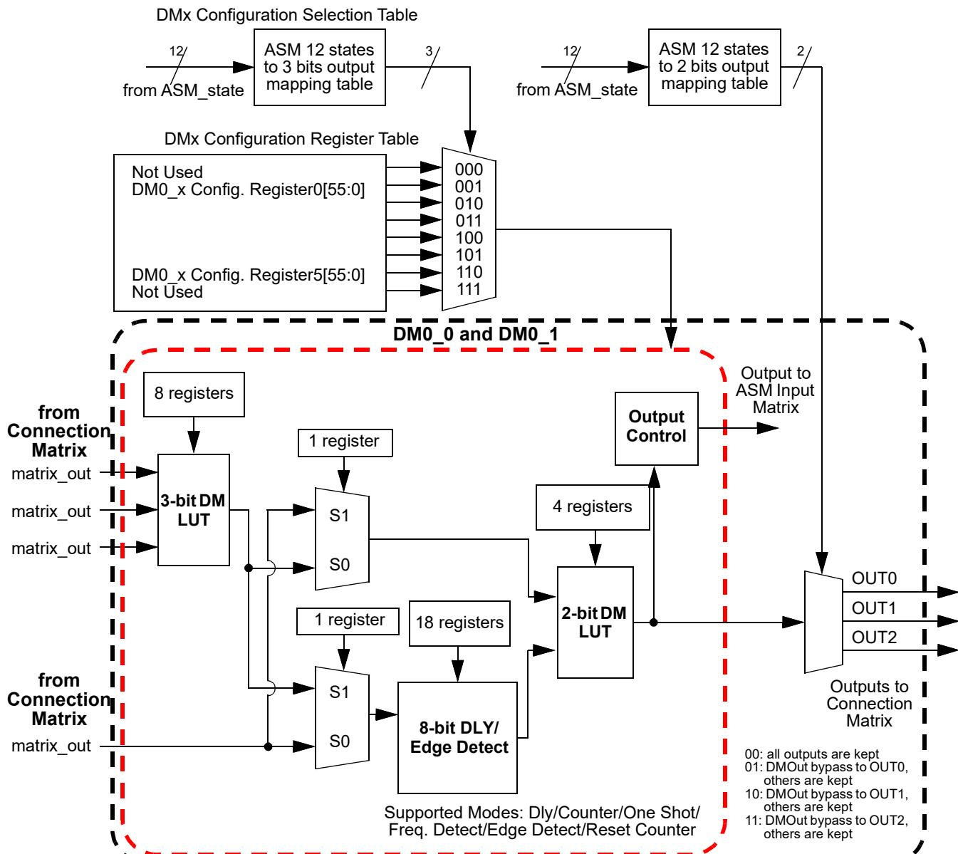
Figure 111: DM0\_0/DM0\_1
