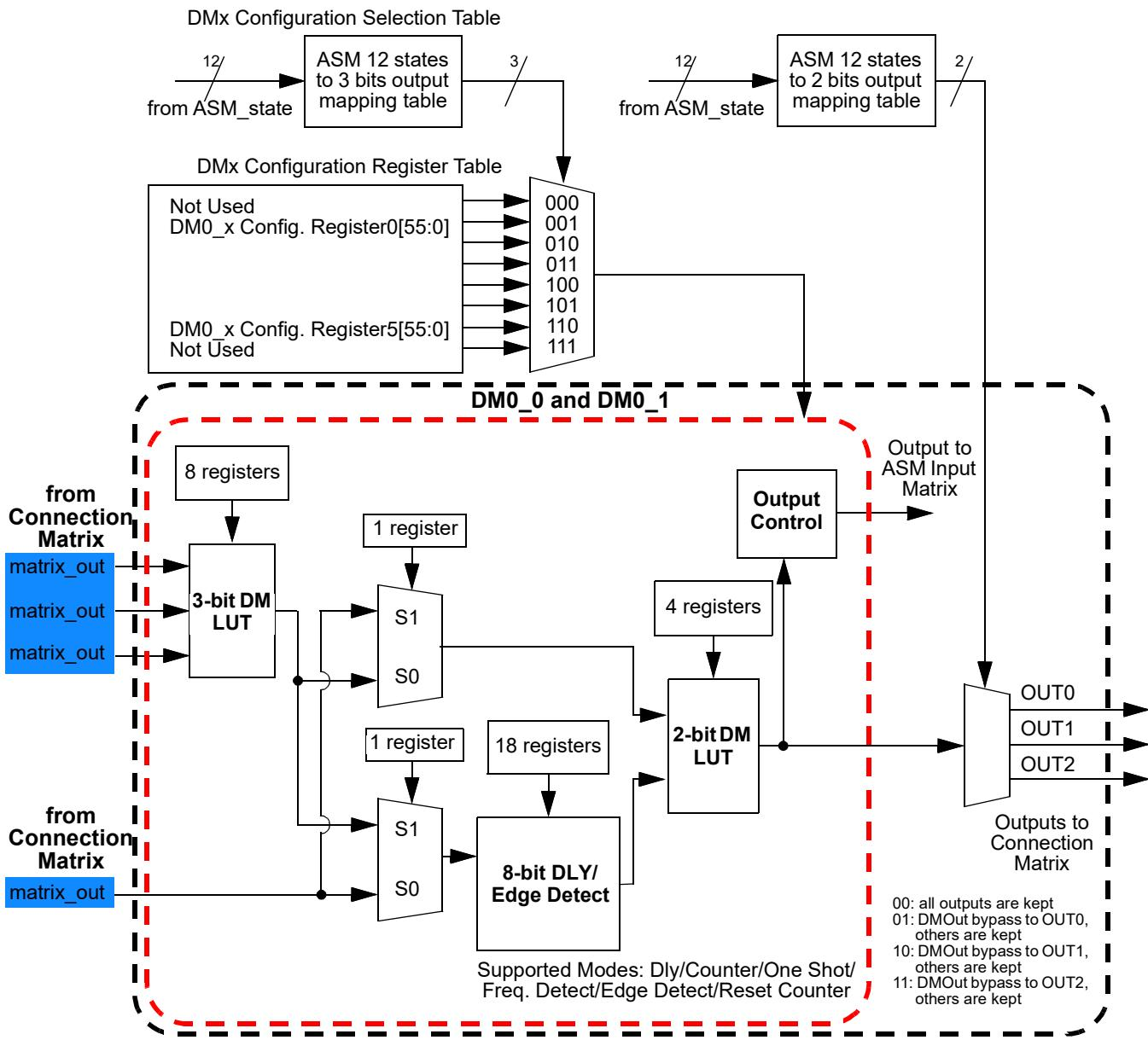
Figure 113: DM0\_0/DM0\_1 Inputs
