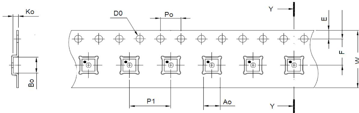
**Note:** 1. Orientation in carrier: Pin1 is at upper left corner (Quadrant1).
