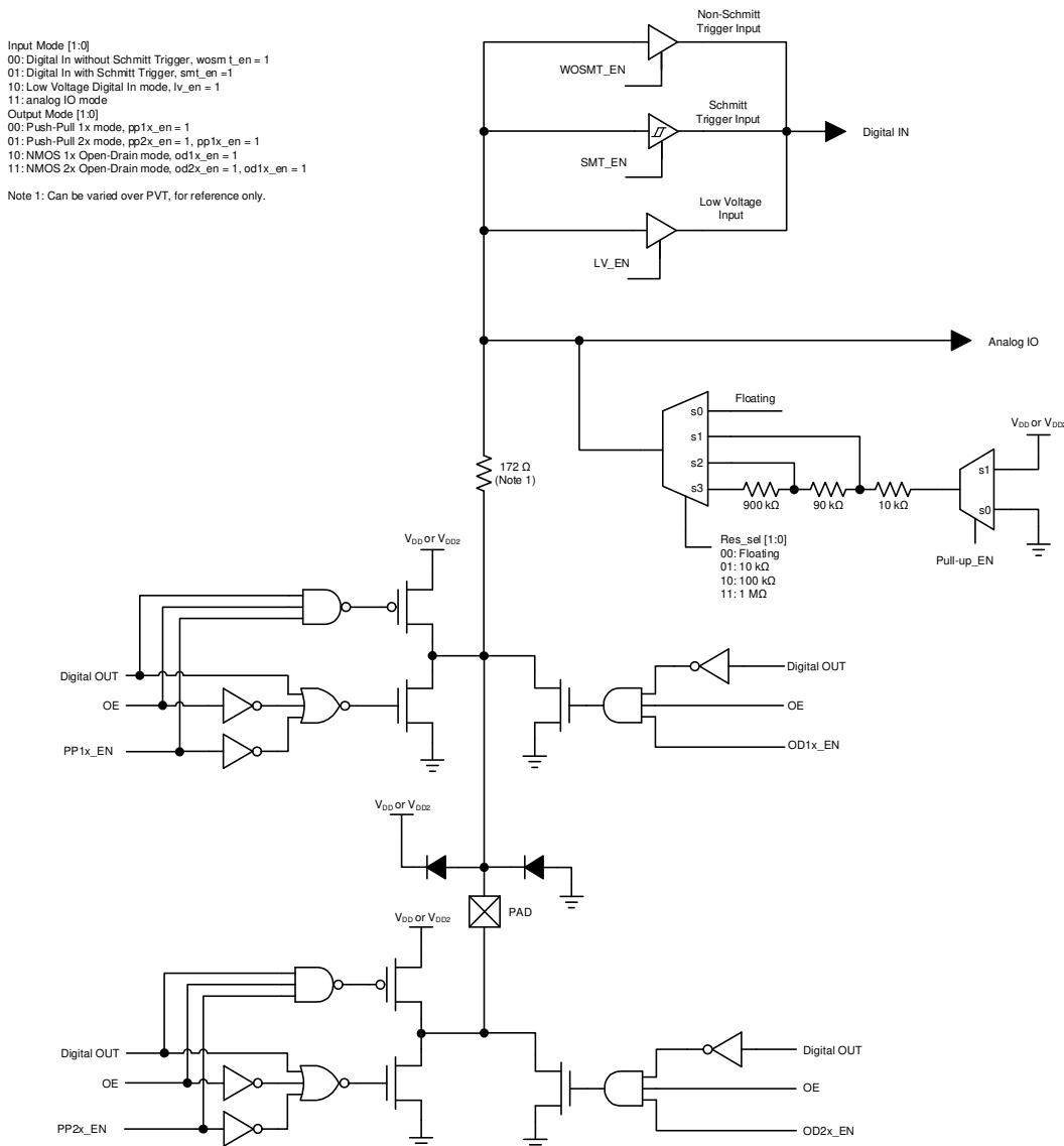
Figure 8: GPIO with Matrix OE IO Structure Diagram
