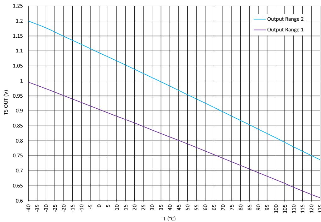
Figure 135: TS Output vs. Temperature,  $V_{DD}$  = 2.3 V to 5.5 V
