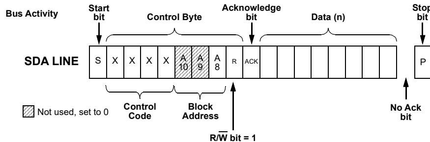
Figure 129: Current Address Read Command, R/W = 1
