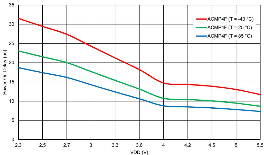
Figure 122: ACMP4F Power-On Delay vs. V<sub>DD</sub>
