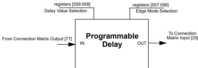
**Figure 63: Programmable Delay**
