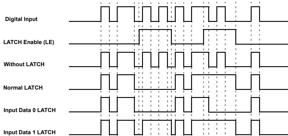
Figure 3: Digital Input Latch Timing Diagram
