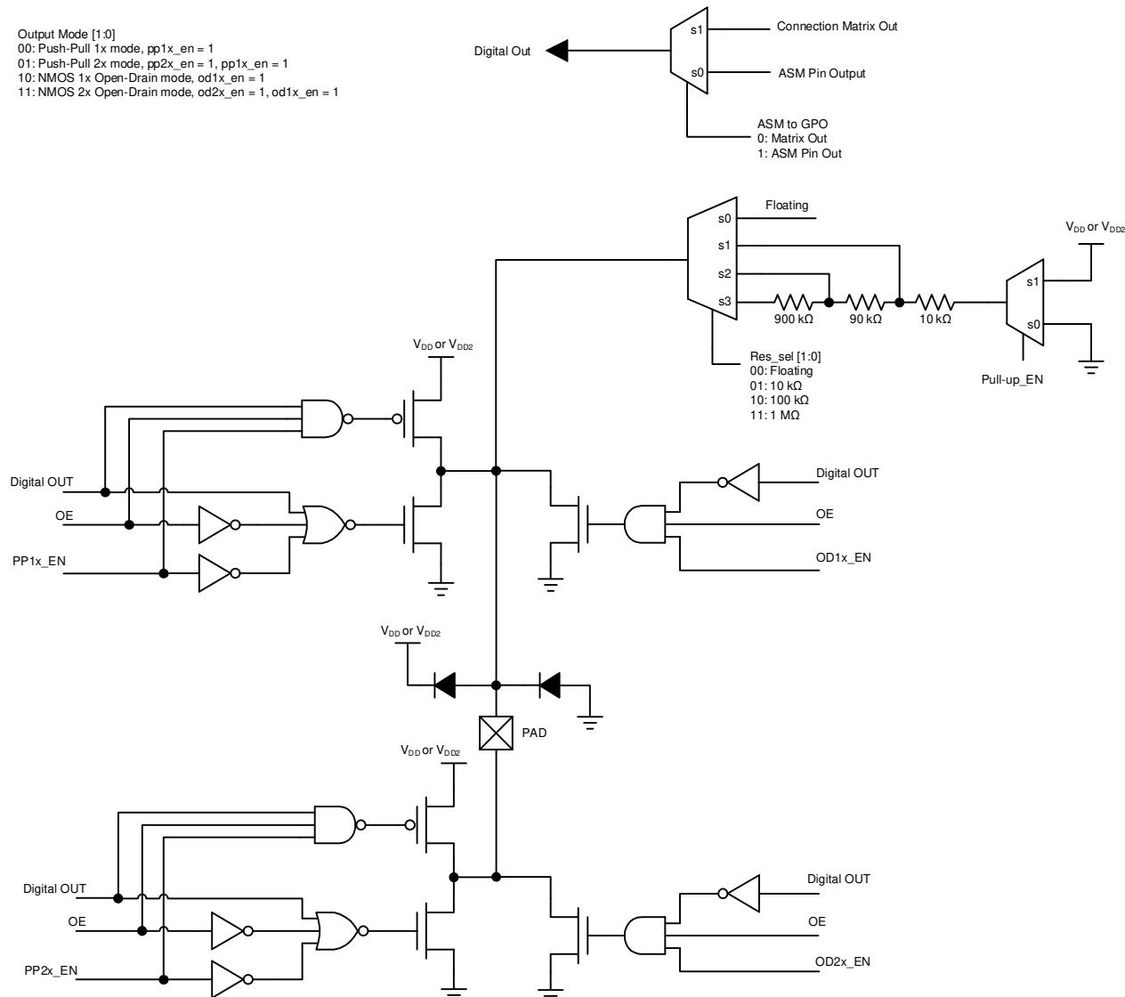
Figure 11: GPO Register OE IO Structure Diagram
