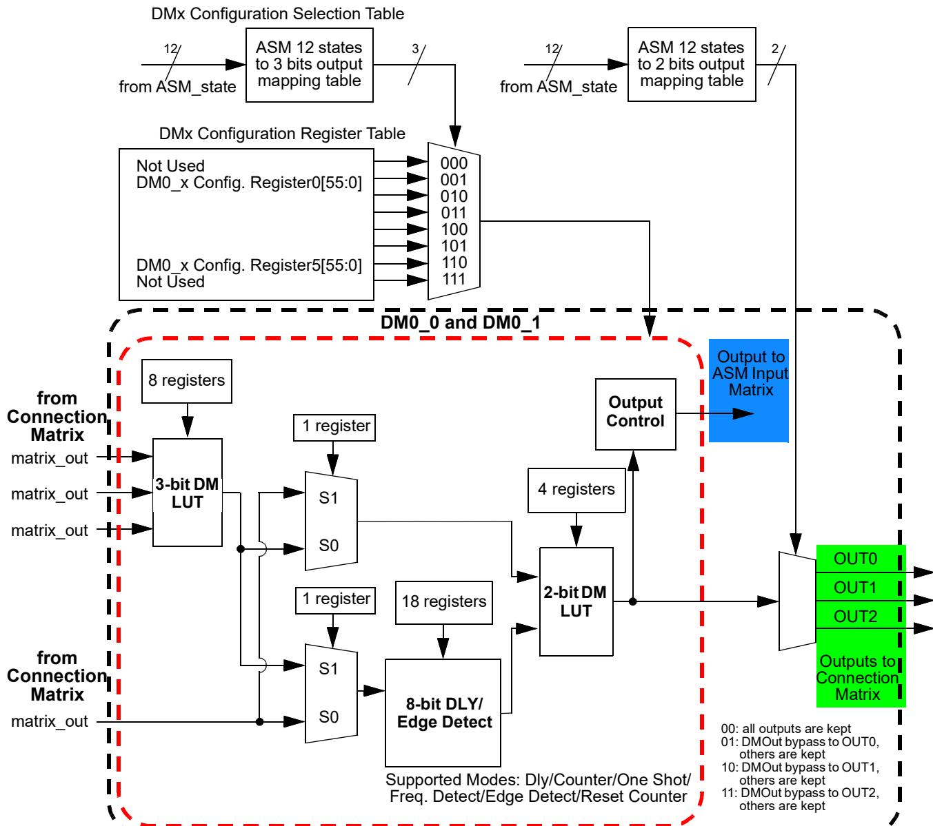
Figure 115: DM0\_0/DM0\_1 Outputs
