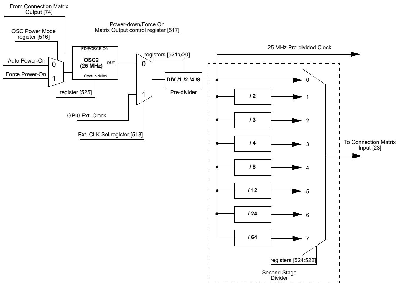
Figure 73: Oscillator2 Block Diagram
