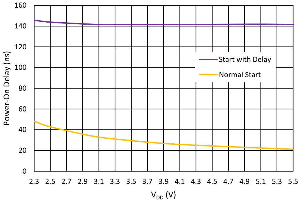
Figure 80: Oscillator2 Maximum Power-On Delay vs. V<sub>DD</sub> at T = 25 °C, OSC2 = 25 MHz
