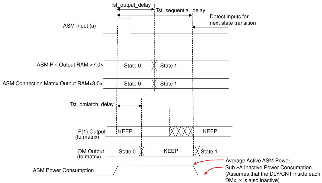
Figure 97: State Transition Timing and Power Consumption
