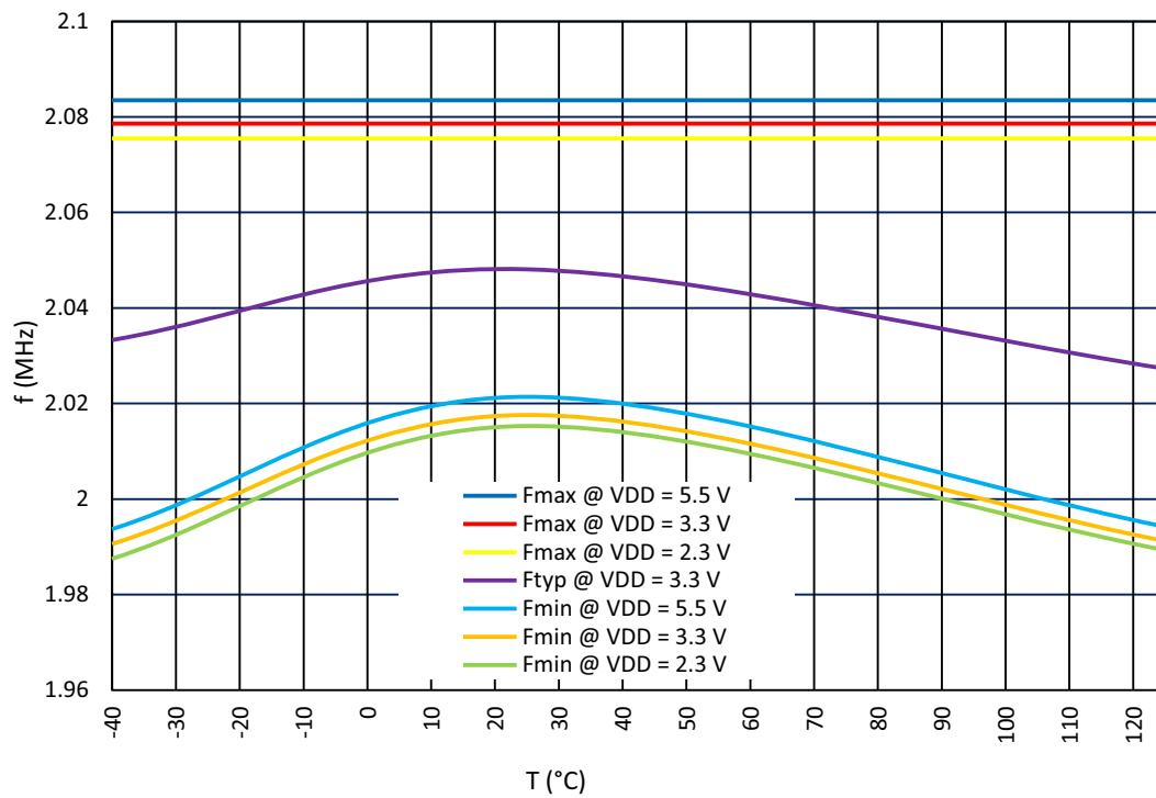
Figure 82: Oscillator1 Frequency vs. Temperature, OSC1 = 2.048 MHz
