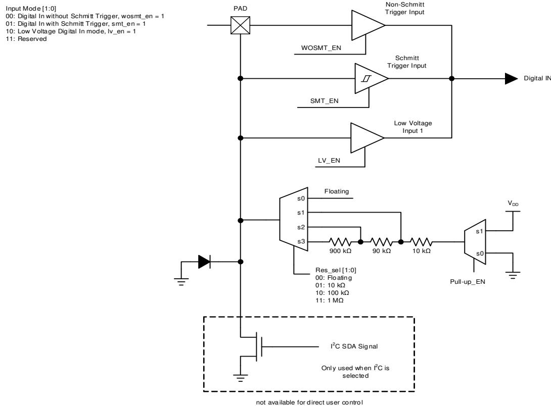
Figure 7: SLG46880 GPI with I<sup>2</sup>C Mode IO Structure Diagram
