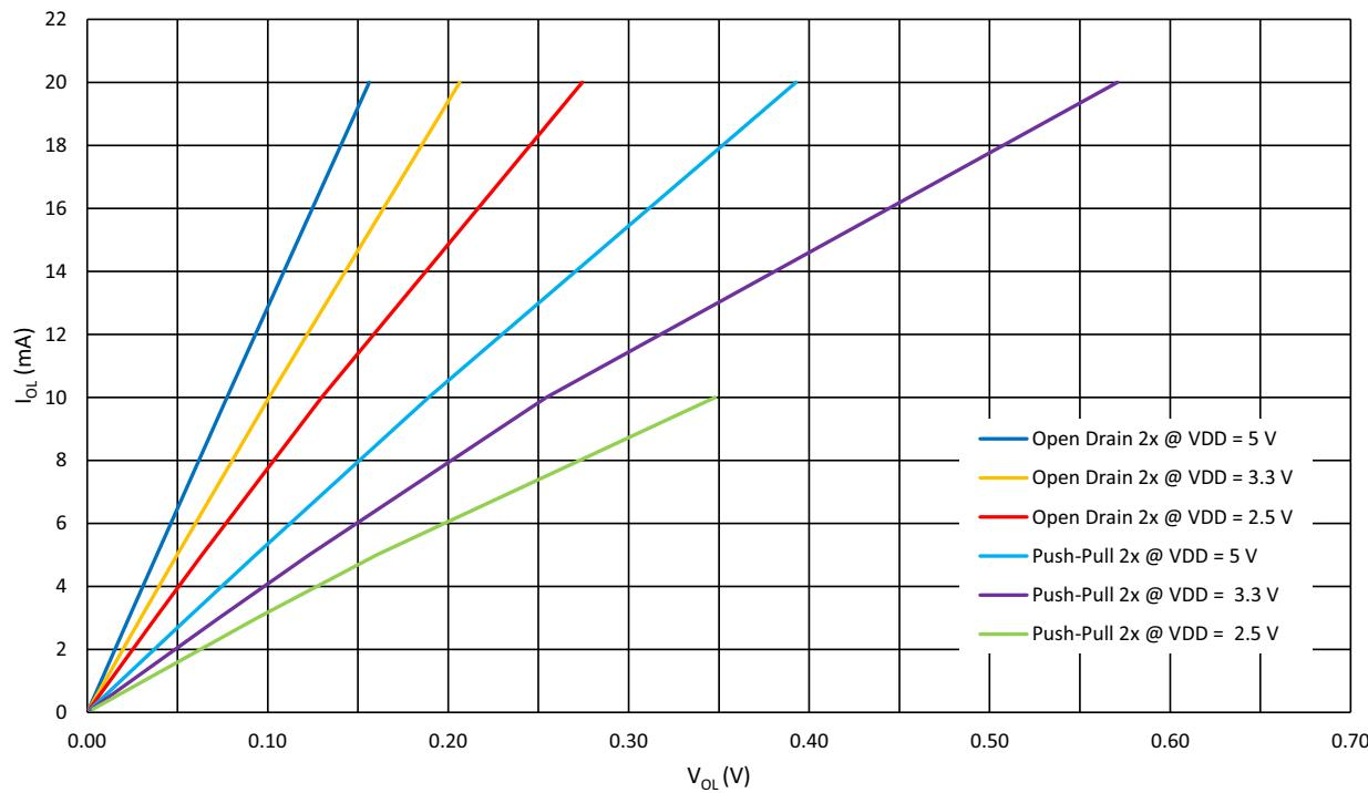
Figure 14: Typical Low Level Output Current vs. Low Level Output Voltage, 2x Drive at  $T = 25^\circ\text{C}$
