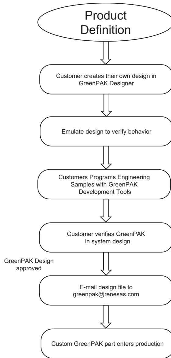
Figure 2: Steps to Create a Custom GreenPAK Device
