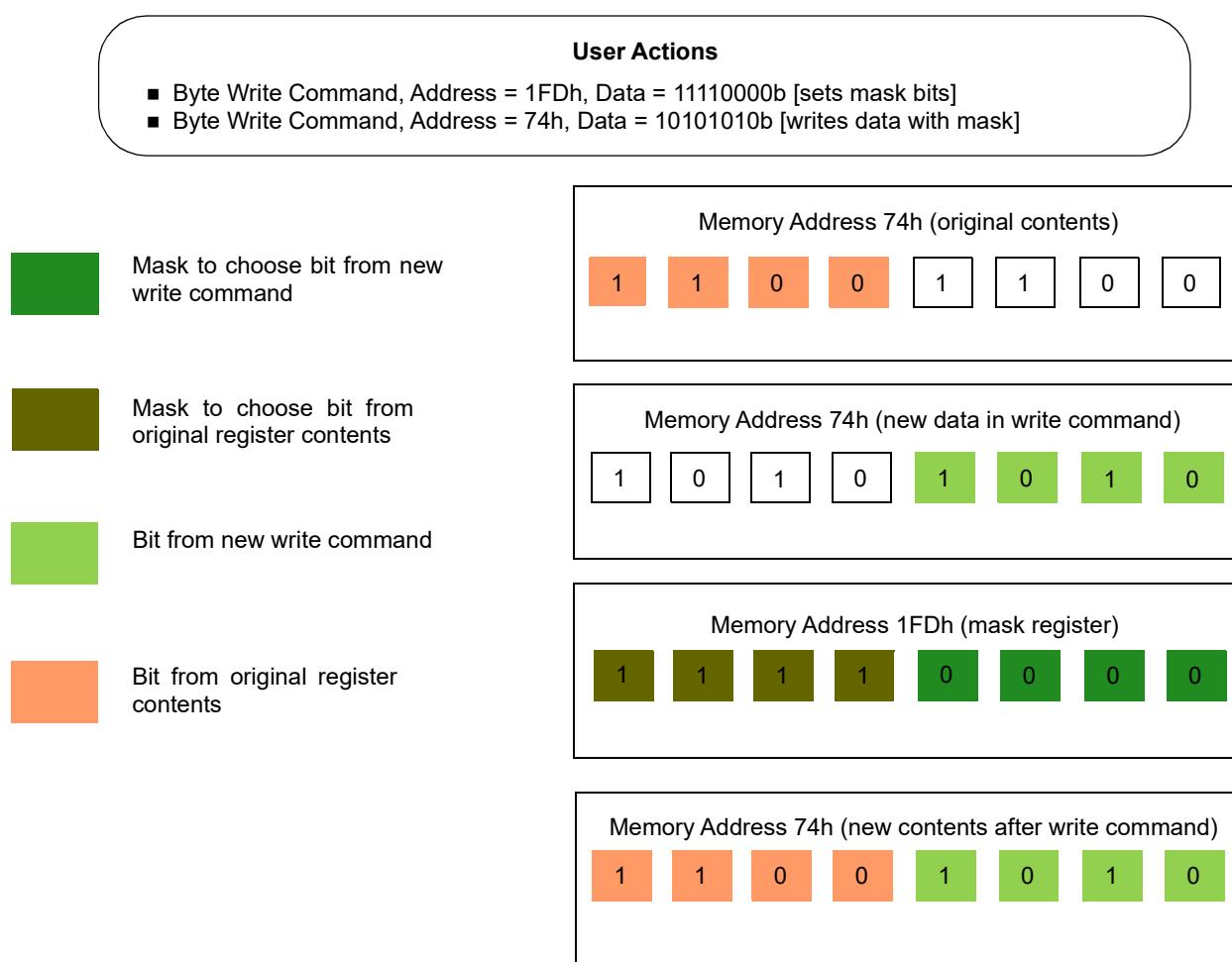
Figure 133: Example of I<sup>2</sup>C Byte Write Bit Masking
