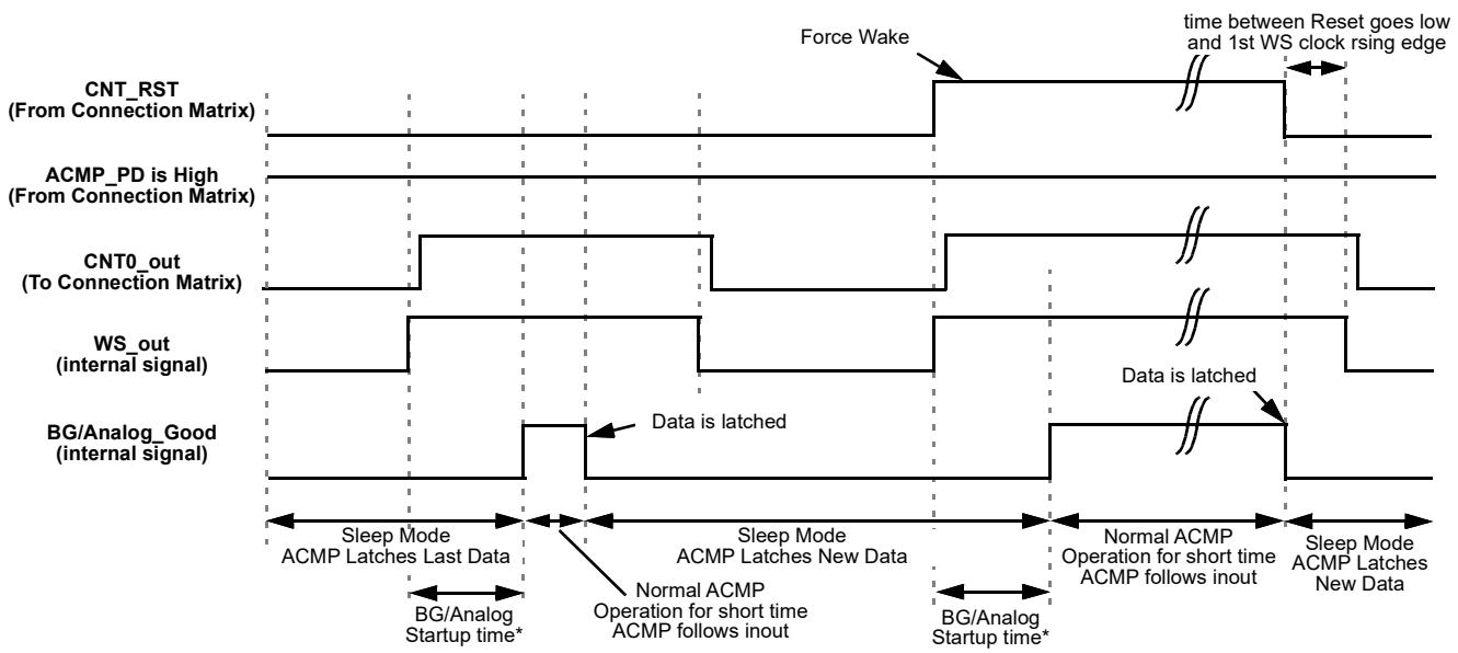
Figure 49: Wake/Sleep Timing Diagram, Short Wake Mode, Counter Reset is Used
