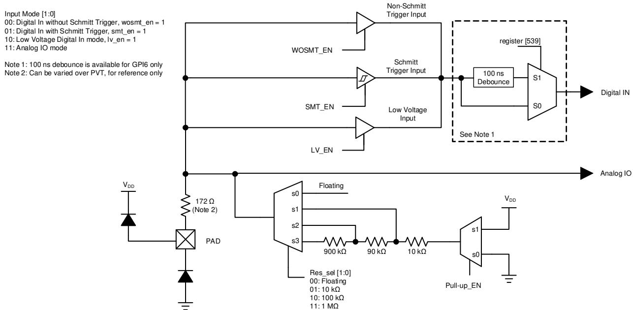
Figure 5: GPIO IO Structure Diagram
