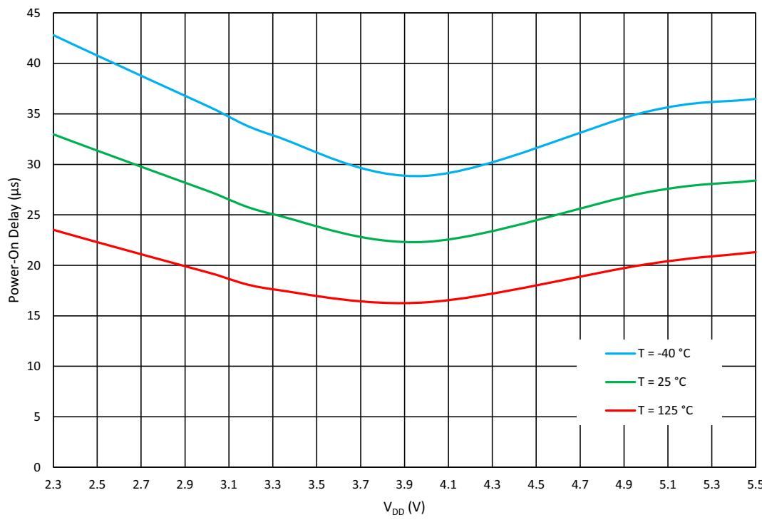
Figure 58: ACMPxH Power-On Delay vs.  $V_{DD}$
