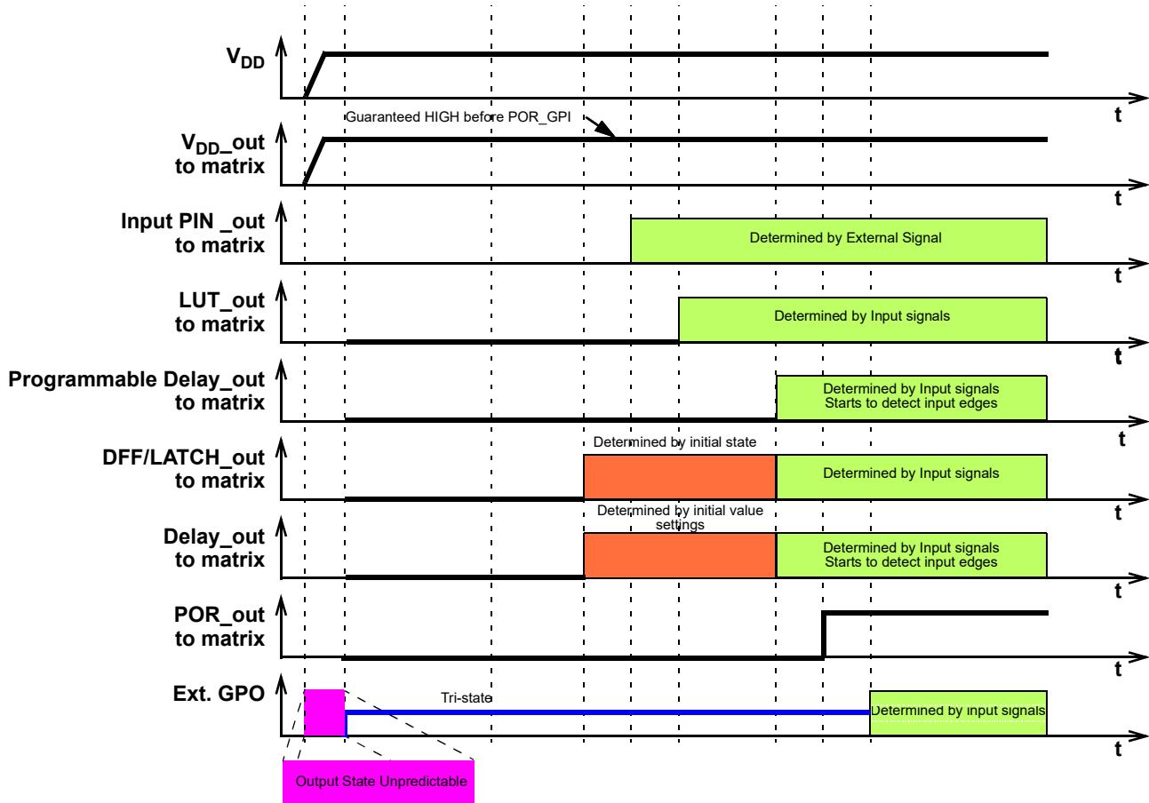
Figure 86: Internal Macrocell States during POR Sequence
