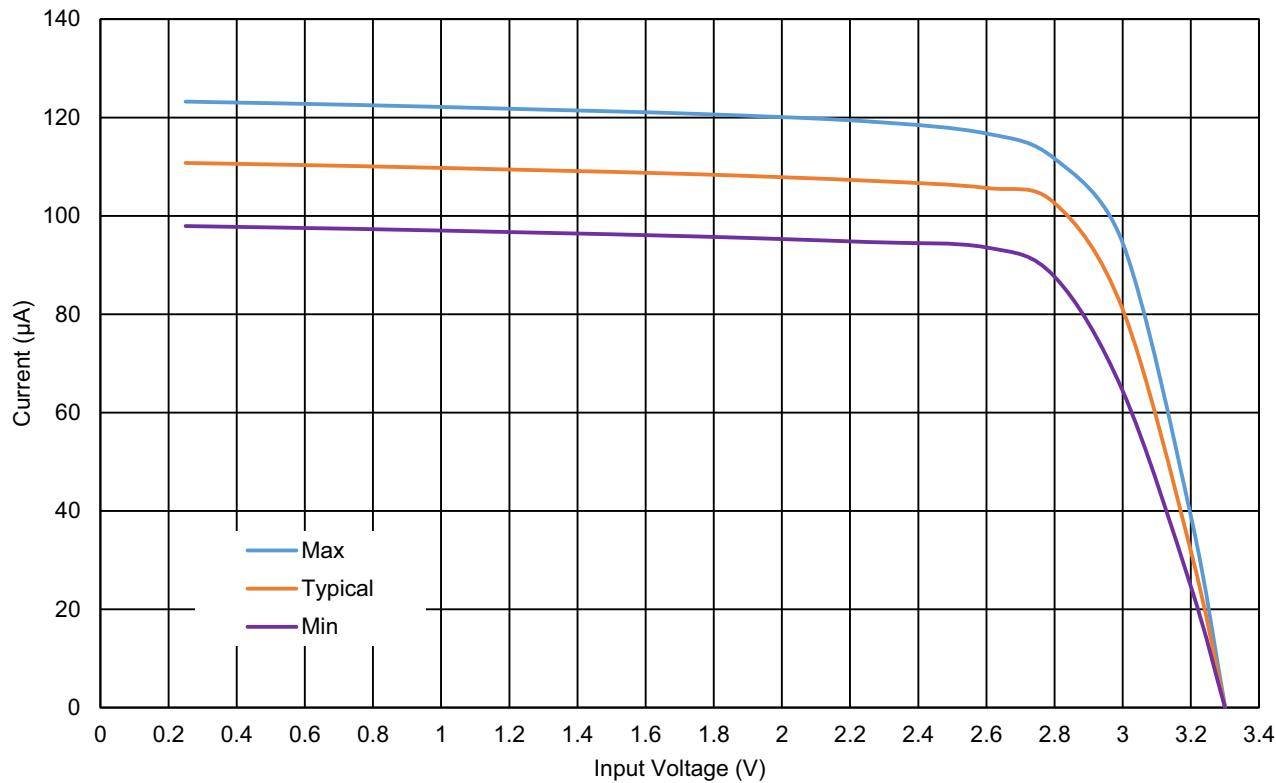
Figure 62: ACMP Input Current Source vs. Input Voltage at  $T = -40\text{ }^{\circ}\text{C}$  to  $125\text{ }^{\circ}\text{C}$ ,  $V_{DD} = 3.3\text{ V}$
