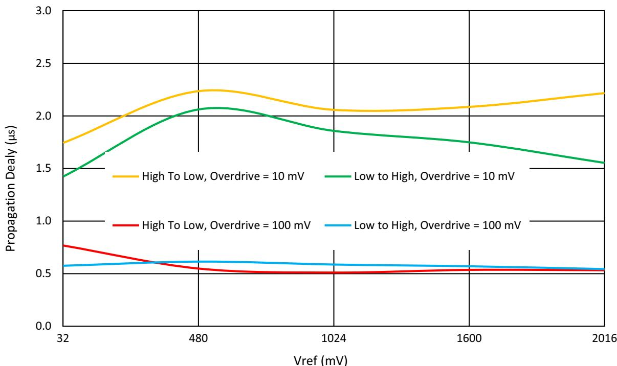
Figure 56: Typical Propagation Delay vs. Vref for ACMPxH at  $T = 25^\circ\text{C}$ ,  $V_{\text{DD}} = 2.3\text{ V to }5.5\text{ V}$ , Gain = 1, Hysteresis = 0
