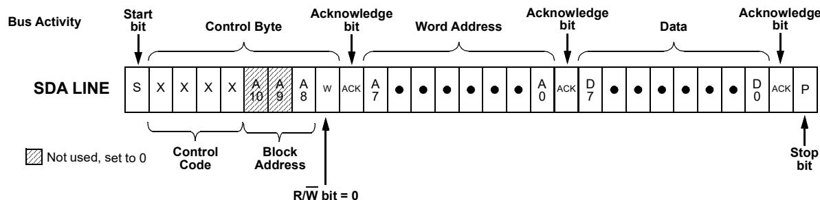
Figure 127: Byte Write Command,  $\overline{R/W} = 0$
