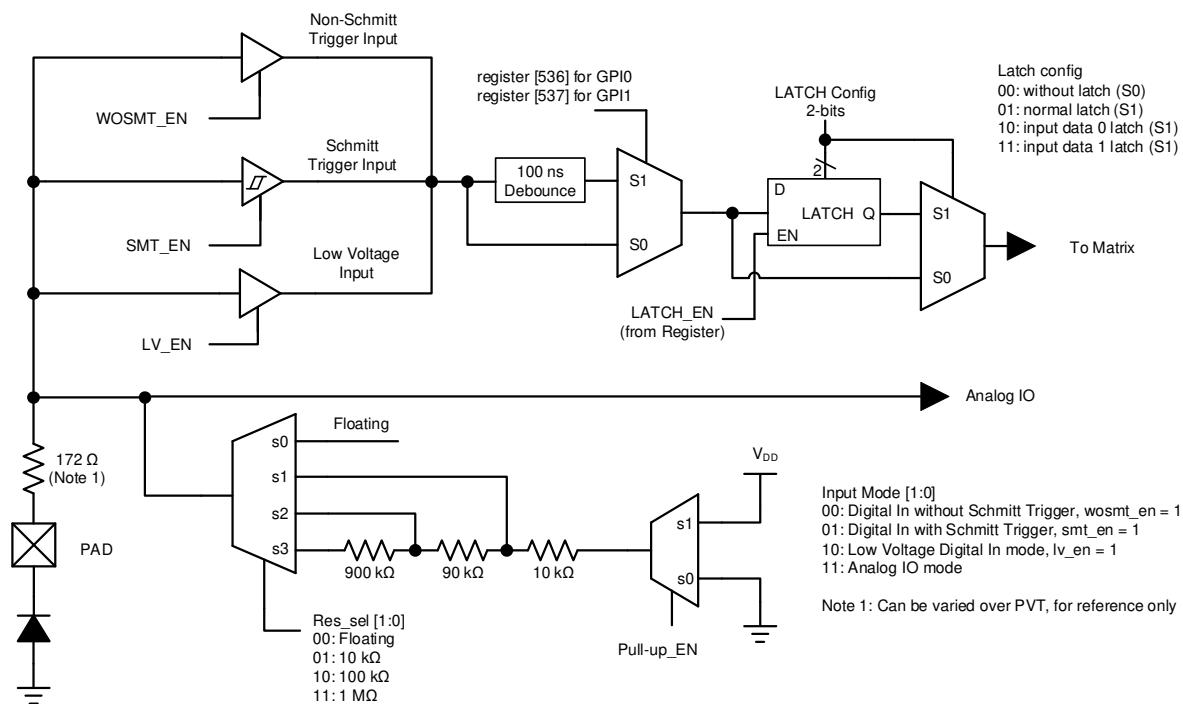
Figure 6: GPI with Input LATCH Structure Diagram
