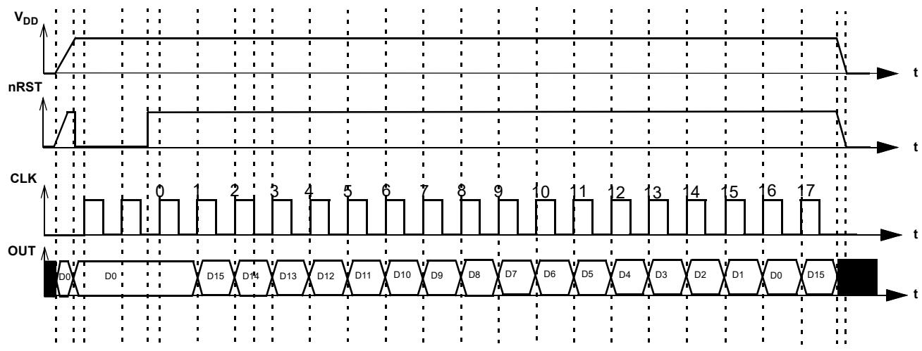
Figure 20: PGen Timing Diagram
