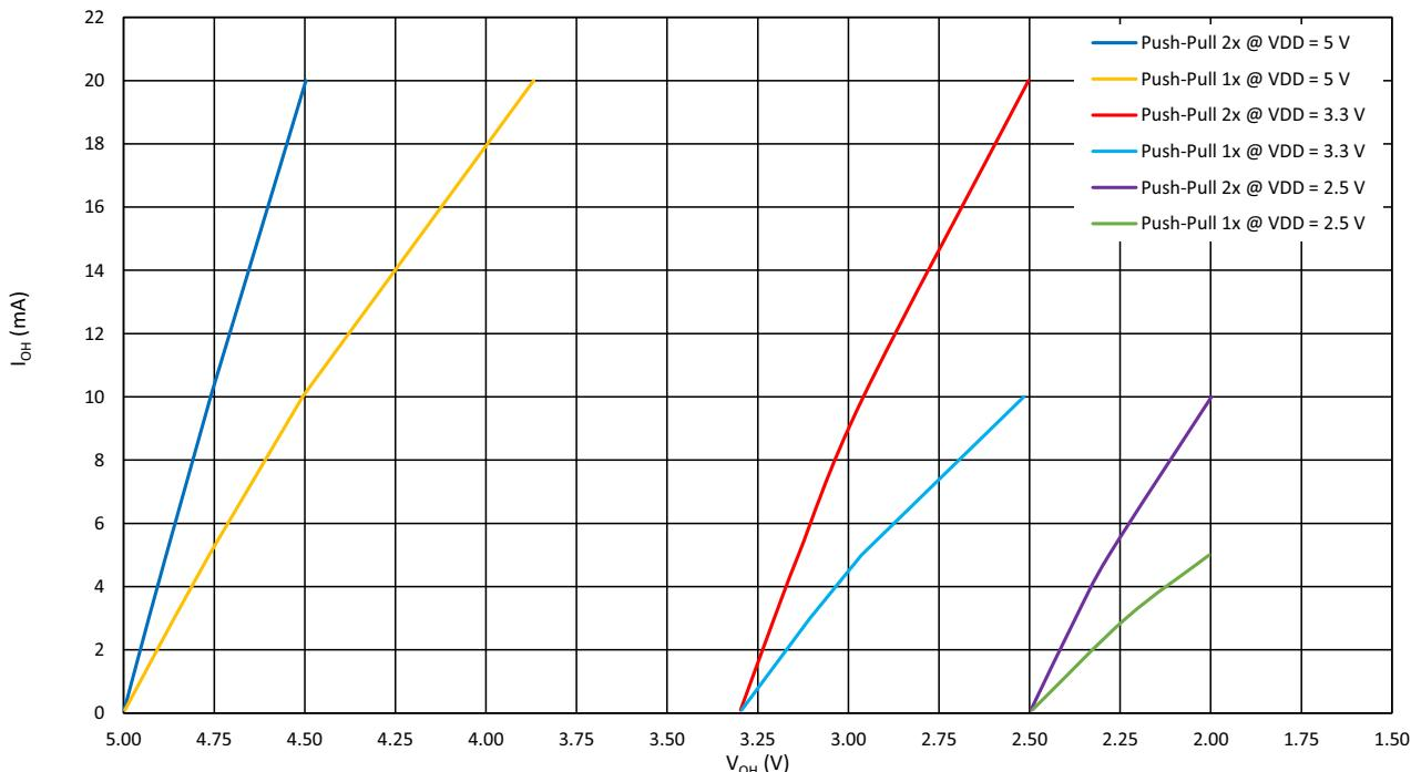
Figure 12: Typical High Level Output Current vs. High Level Output Voltage at  $T = 25^\circ\text{C}$
