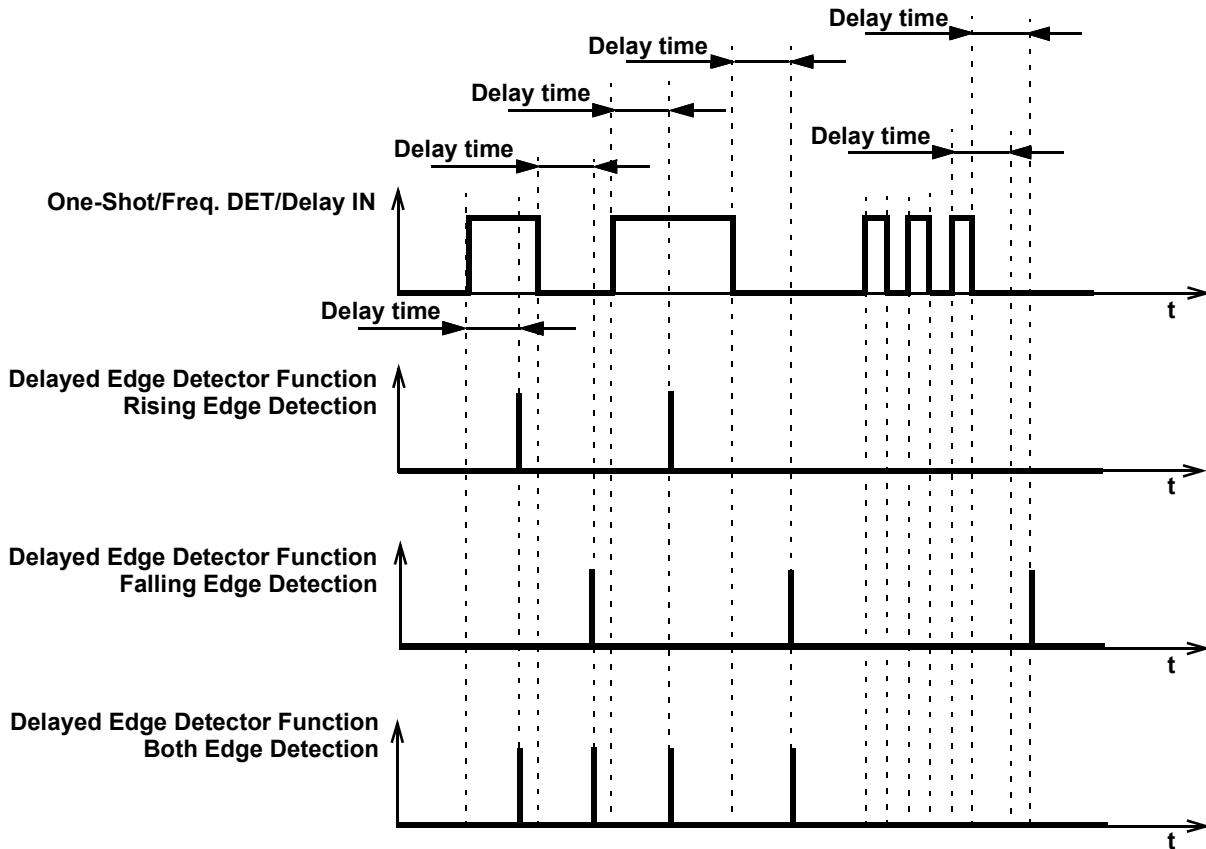
Figure 40: Delayed Edge Detection Mode Timing Diagram
