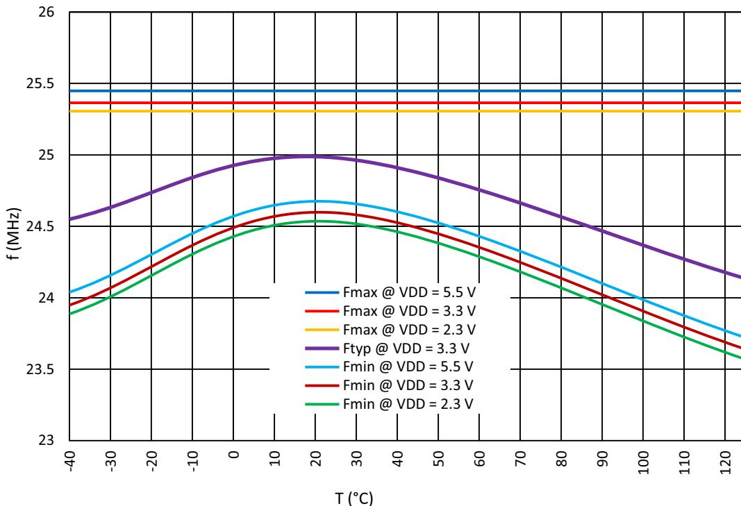
Figure 83: Oscillator2 Frequency vs. Temperature, OSC2 = 25 MHz
