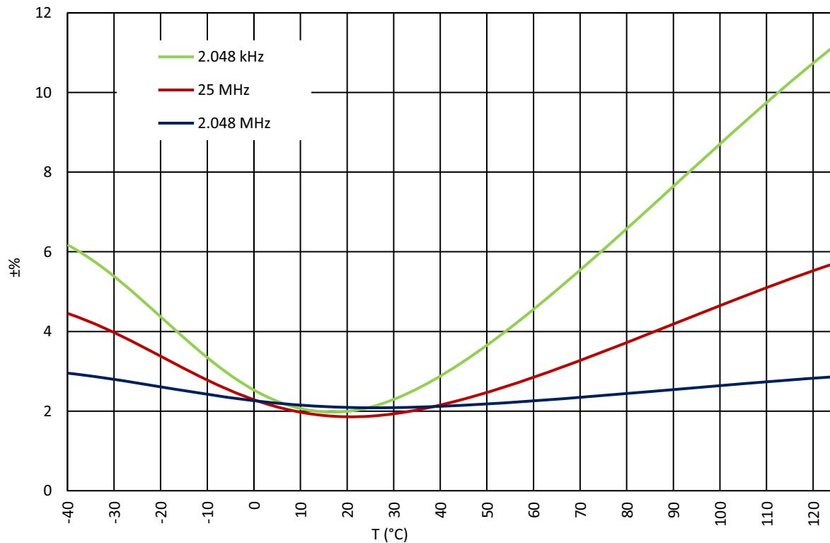
Figure 84: Oscillators Total Error vs. Temperature at  $V_{DD}$  = 2.3 V to 5.5 V
