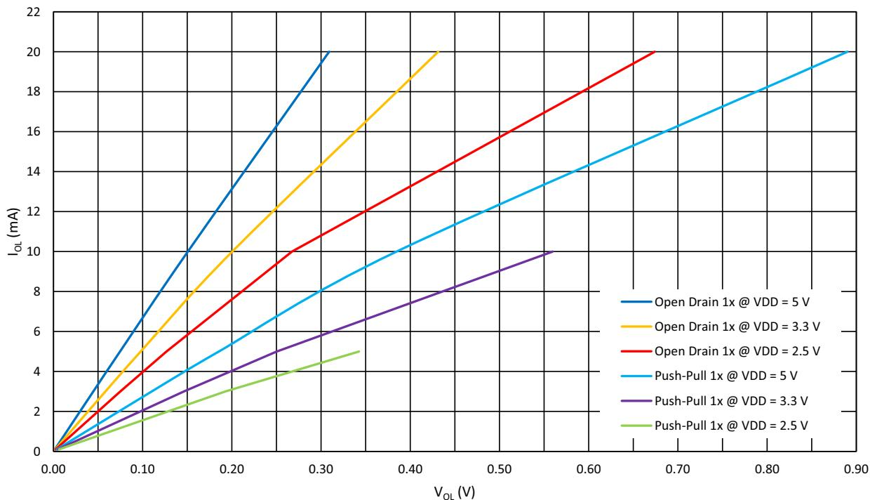
Figure 13: Typical Low Level Output Current vs. Low Level Output Voltage, 1x Drive at  $T = 25^\circ\text{C}$
