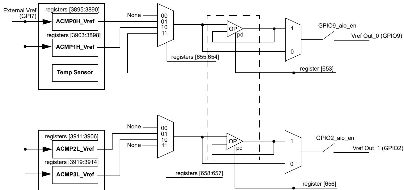
Figure 66: Voltage Reference Block Diagram
