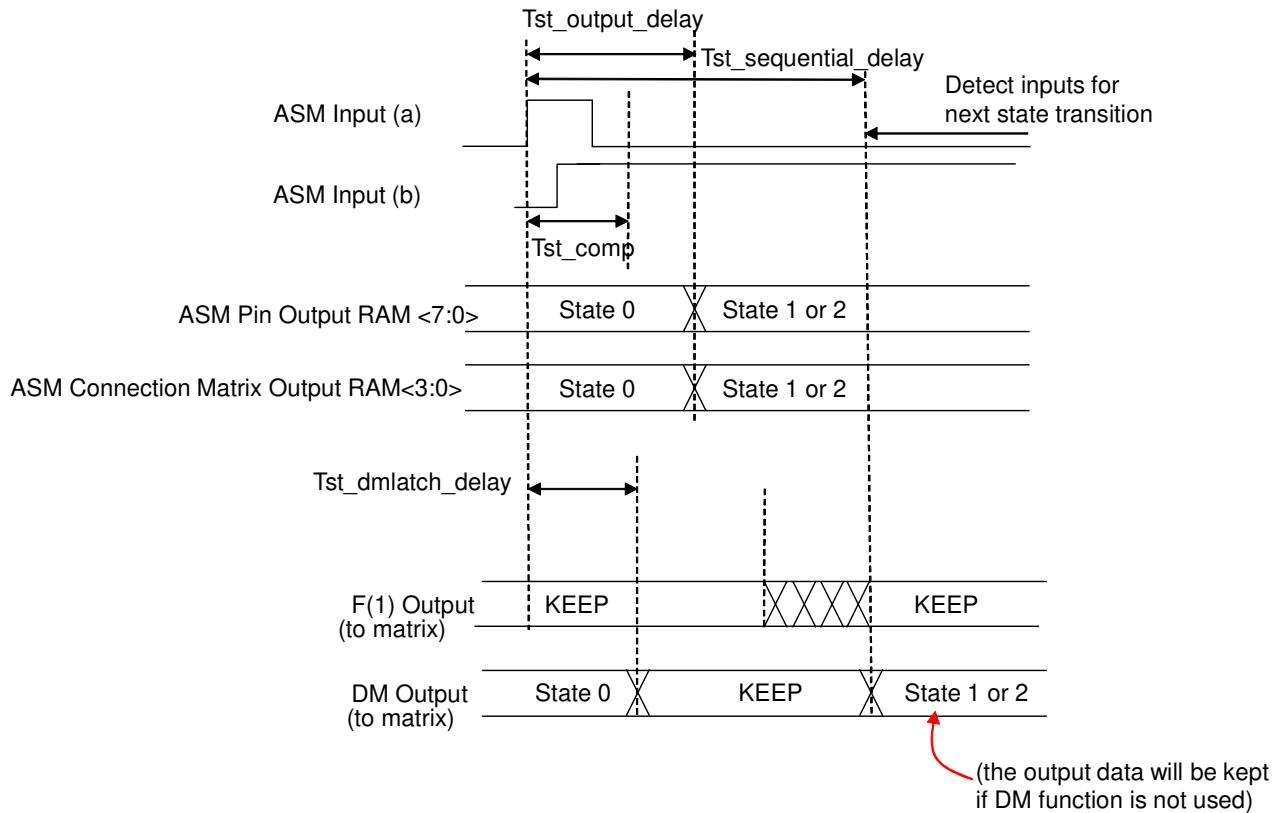
**Figure 101: State Transition Timing - Competing Inputs Indeterminate**
