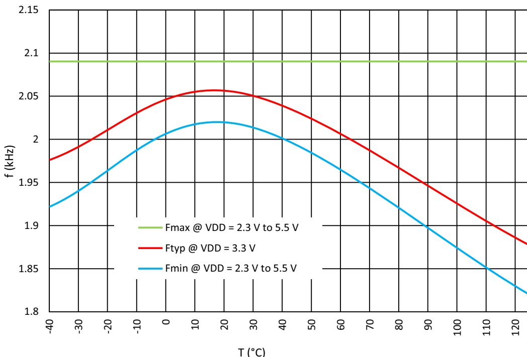
Figure 81: Oscillator0 Frequency vs. Temperature, OSC0 = 2.048 kHz
