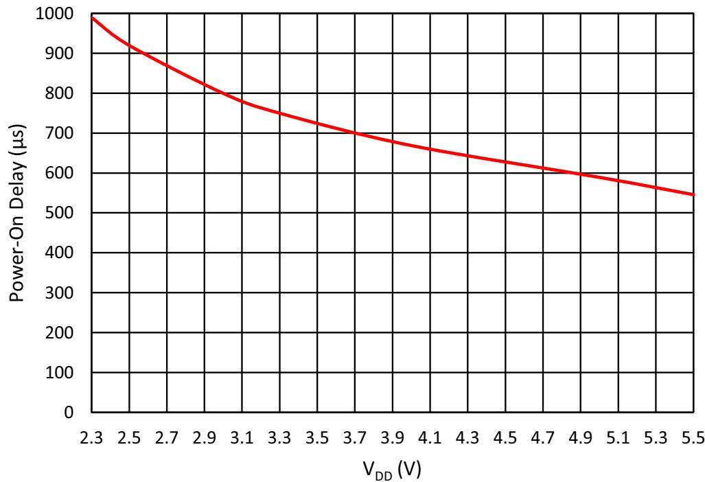
Figure 78: Oscillator0 Maximum Power-On Delay vs.  $V_{DD}$  at  $T = 25^{\circ}\text{C}$ , OSC0 = 2.048 kHz
