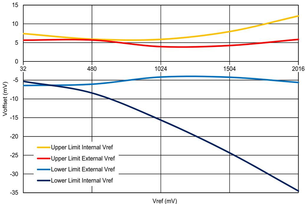
Figure 123: ACMP4F Input Offset Voltage vs. V<sub>ref</sub> at T = -40 °C to 125 °C, Input Buffer Disabled
