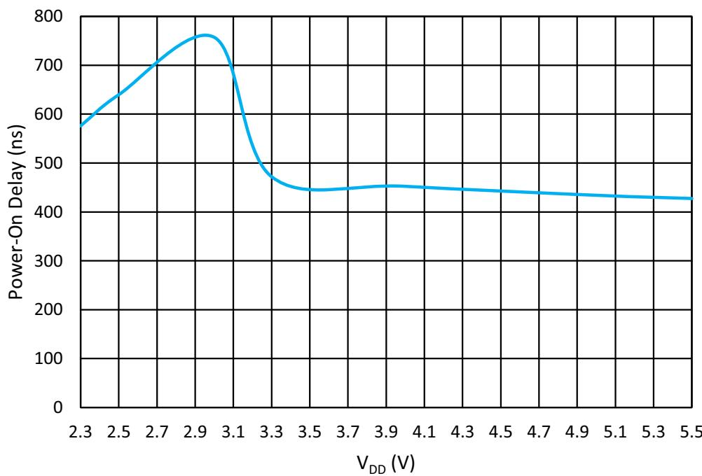
Figure 79: Oscillator1 Maximum Power-On Delay vs.  $V_{DD}$  at  $T = 25^{\circ}\text{C}$ , OSC1 = 2.048 MHz
