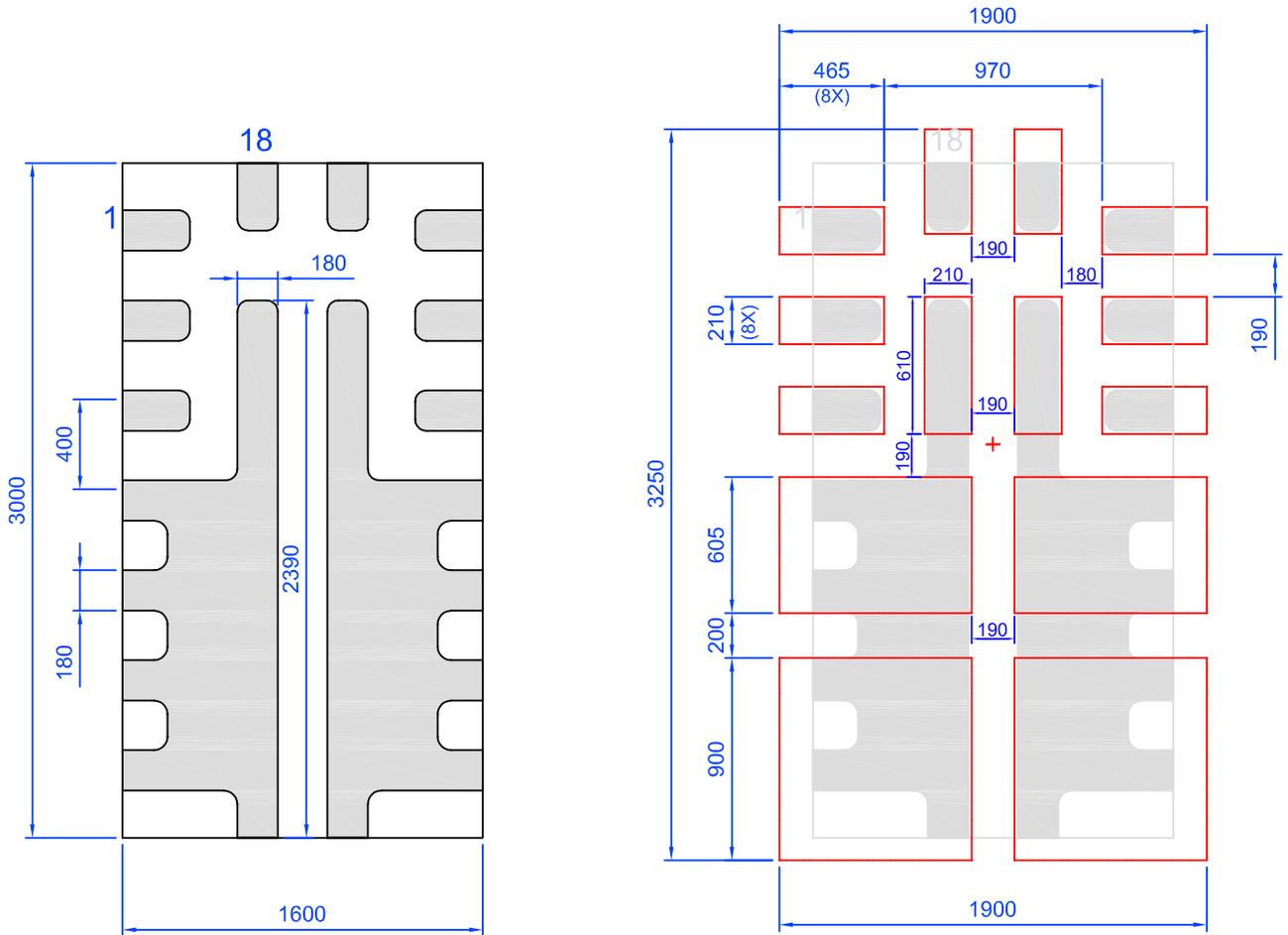
Note: All dimensions shown in micrometers ( $\mu\text{m}$ )
