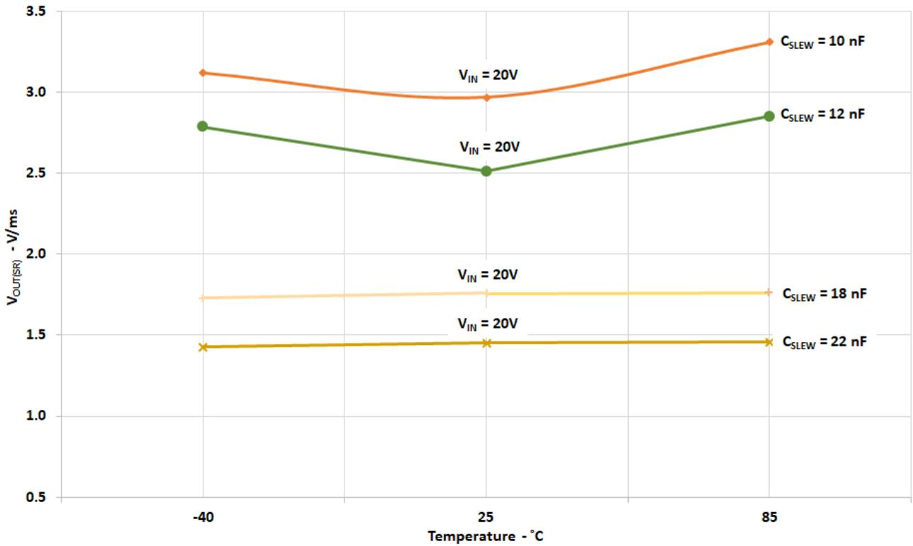
$T_{Total\_ON}$  vs.  $C_{SLEW}$  and Temperature
