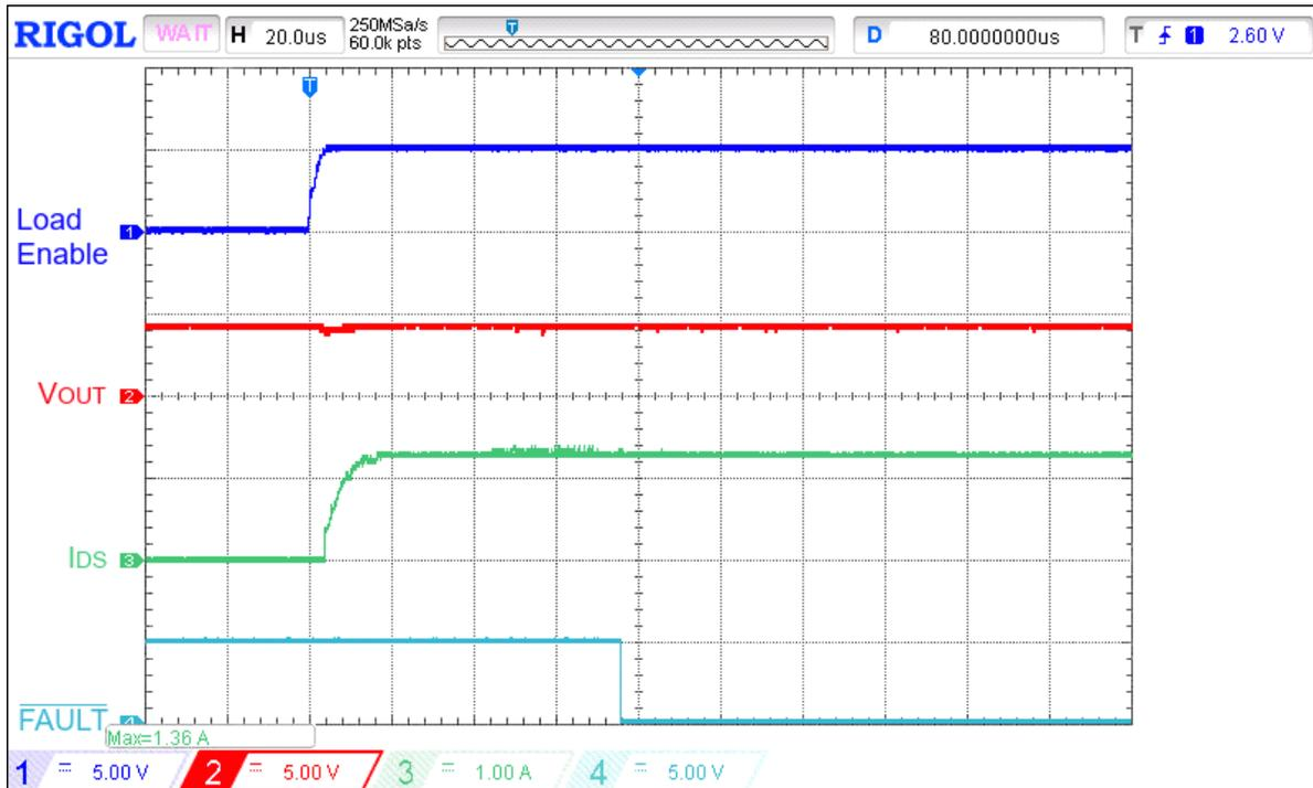
Figure 8. Typical FAULT assertion waveform for  $V_{IN} = 4.5\text{ V}$ ,  $C_{LOAD} = 10\text{ }\mu\text{F}$ ,  $I_{ACL} = 1\text{ A}$ ,  $R_{SET} = 91\text{ k}\Omega$ , switch on  $3.3\text{ }\Omega$  load
