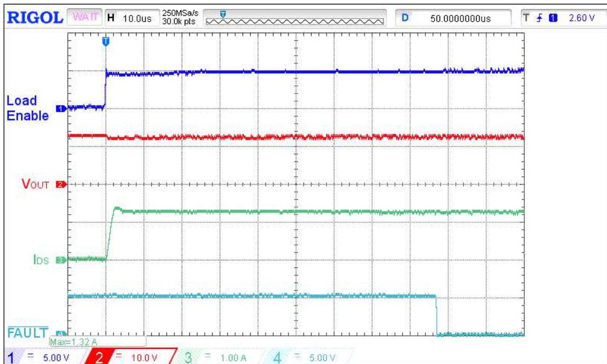
Figure 14. Typical  $\overline{\text{FAULT}}$  assertion waveform for  $V_{IN} = 12 \text{ V}$ ,  $C_{LOAD} = 10 \mu\text{F}$ ,  $I_{ACL} = 1 \text{ A}$ ,  $R_{SET} = 95.3 \text{ k}\Omega$ , switch on  $10 \Omega$  load
