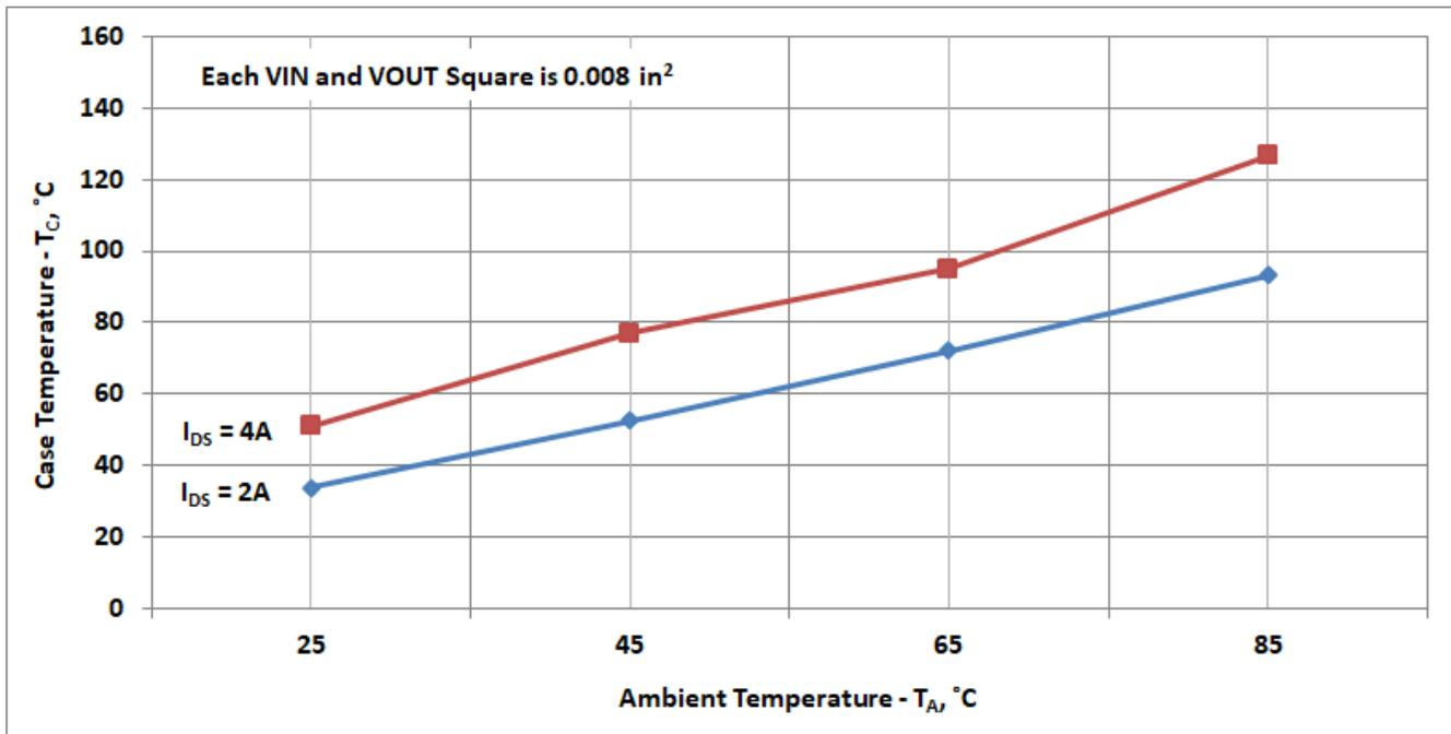
Case Temperature vs. Ambient Temperature (each  $V_{IN}$  and  $V_{OUT}$  square is 0.25 in<sup>2</sup>, no airflow)
