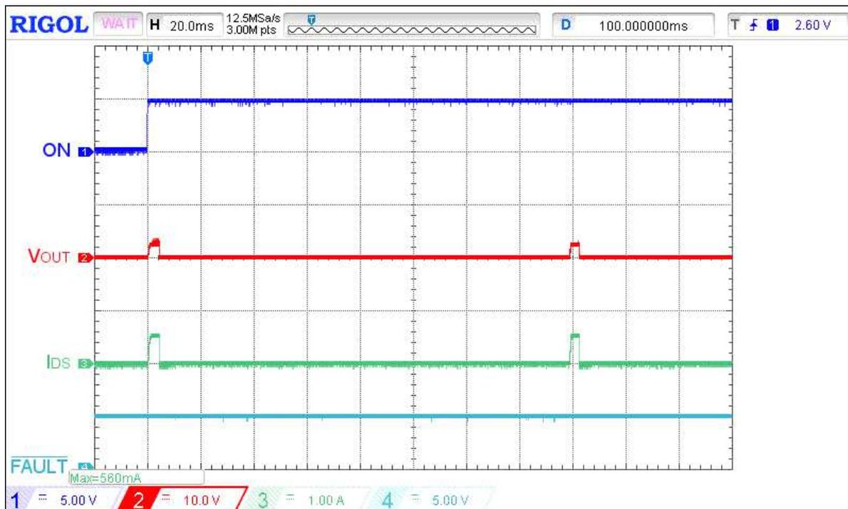
Figure 18. Extended typical SOA waveform during power up under heavy load for  $V_{IN} = 12\text{ V}$ ,
