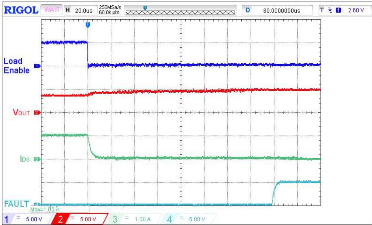
Figure 13. Typical  $\overline{\text{FAULT}}$  de-assertion waveform for  $V_{IN} = 4.5 \text{ V}$ ,  $C_{LOAD} = 10 \mu\text{F}$ ,  $I_{ACL} = 1 \text{ A}$ ,  $R_{SET} = 95.3 \text{ k}\Omega$ , switch out  $3.3 \Omega$  load
