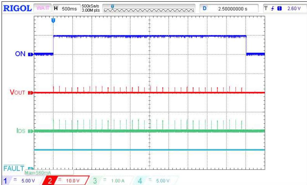
Figure 17. Typical SOA waveform during power up under heavy load for  $V_{IN} = 12\text{ V}$ ,
