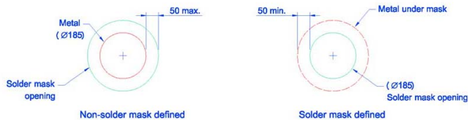
Solder mask detail (not to scale)
