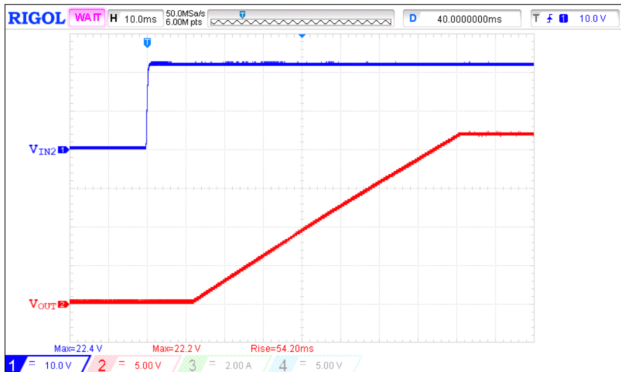
Figure 6. Typical Turn ON operation waveform for V_{IN2} = 22\text{ V} , C_{SS} = 220\text{ nF} , R_{LOAD} = 100\text{ }\Omega , C_{LOAD} = 2\text{ }\mu\text{F}
