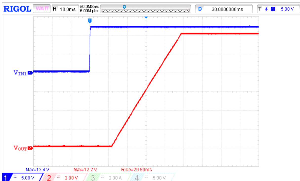
Figure 2. Typical Turn ON operation waveform for V_{IN1} = 12\text{ V} , C_{SS} = 220\text{ nF} , R_{LOAD} = 100\text{ }\Omega , C_{LOAD} = 2\text{ }\mu\text{F}
