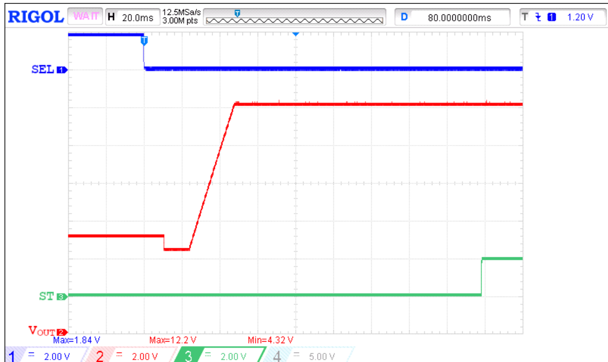
Figure 8. Switchover operation waveform for V_{IN1} = 12\text{ V} , V_{IN2} = 5\text{ V} , C_{SS} = 220\text{ nF} , PR = 0\text{ V} , SEL = \text{High} \rightarrow \text{Low} , R_{LOAD} = 100\text{ }\Omega , C_{LOAD} = 2\text{ }\mu\text{F}
