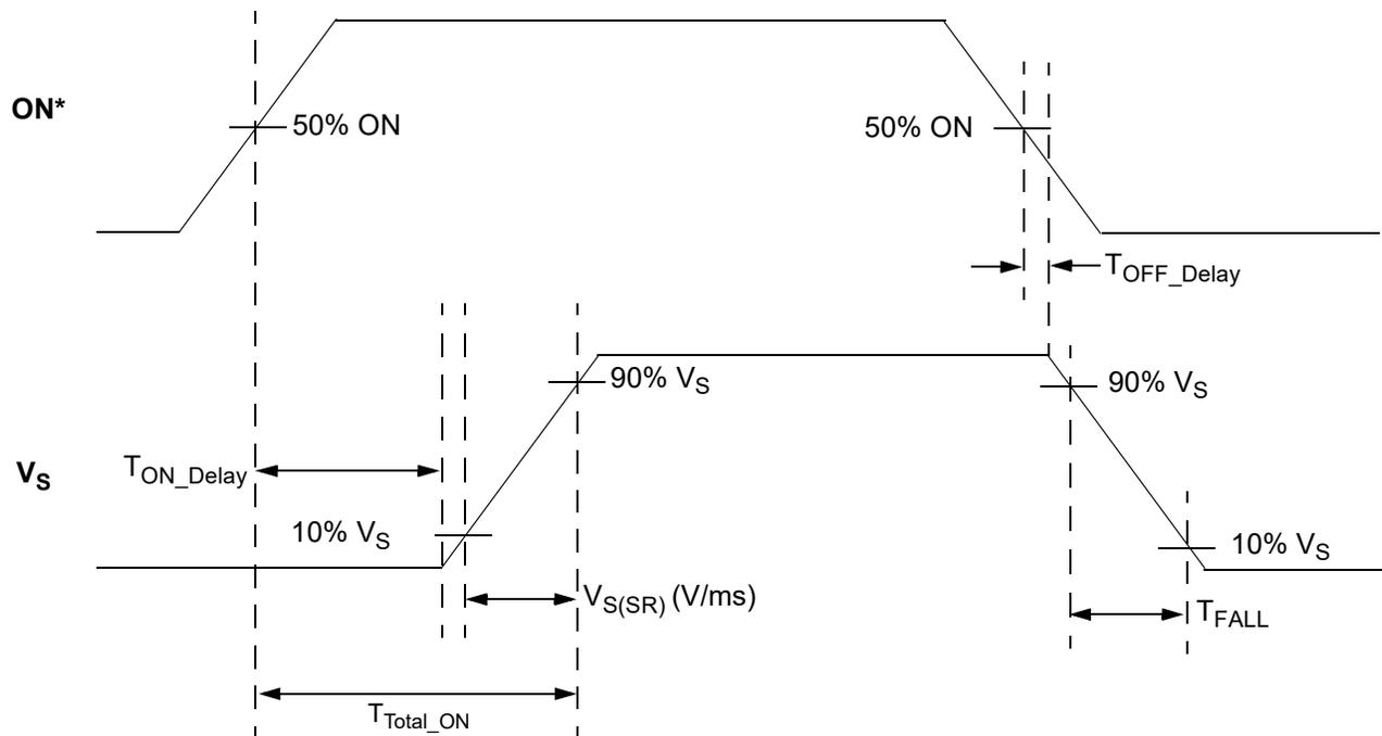
Note: \* Rise and Fall times of the ON signal are 100 ns
