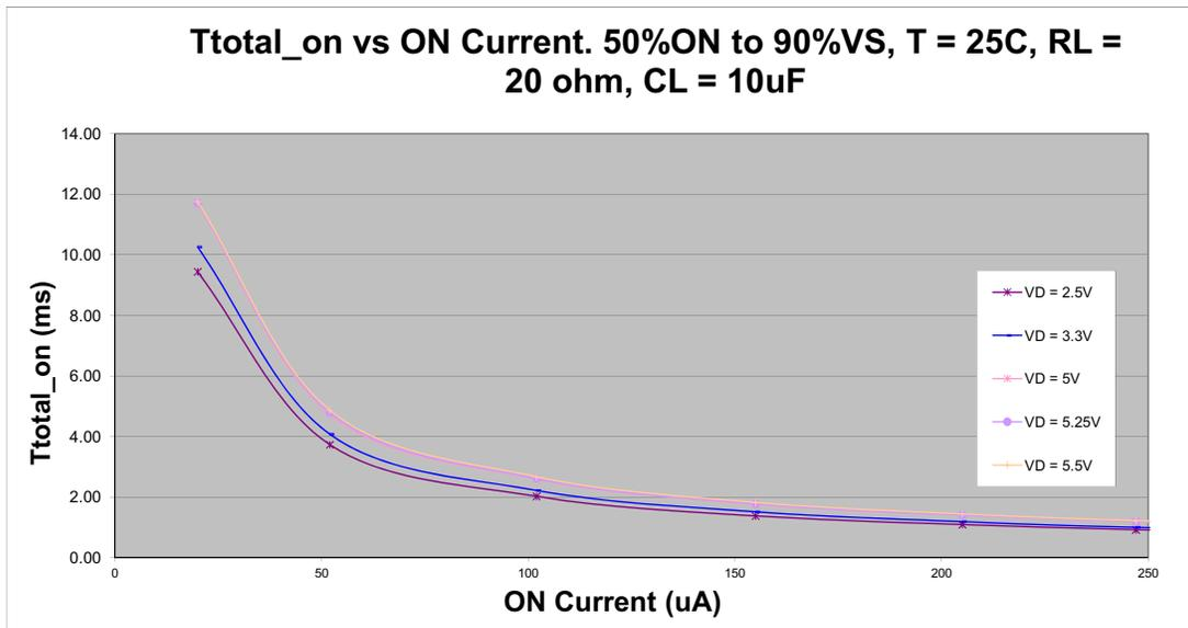
$T_{Total\_ON}$ ,  $T_{ON\_Delay}$  and Slew Rate Measurement
