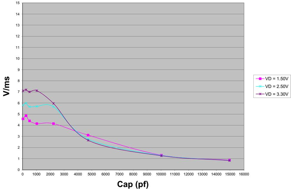
**T<sub>SLEW</sub> vs. CAP @ V<sub>DD</sub> = 5.0 V**
