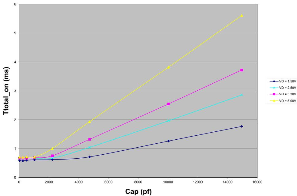
**T<sub>SLEW</sub> vs. CAP @ V<sub>DD</sub> = 3.3 V**
