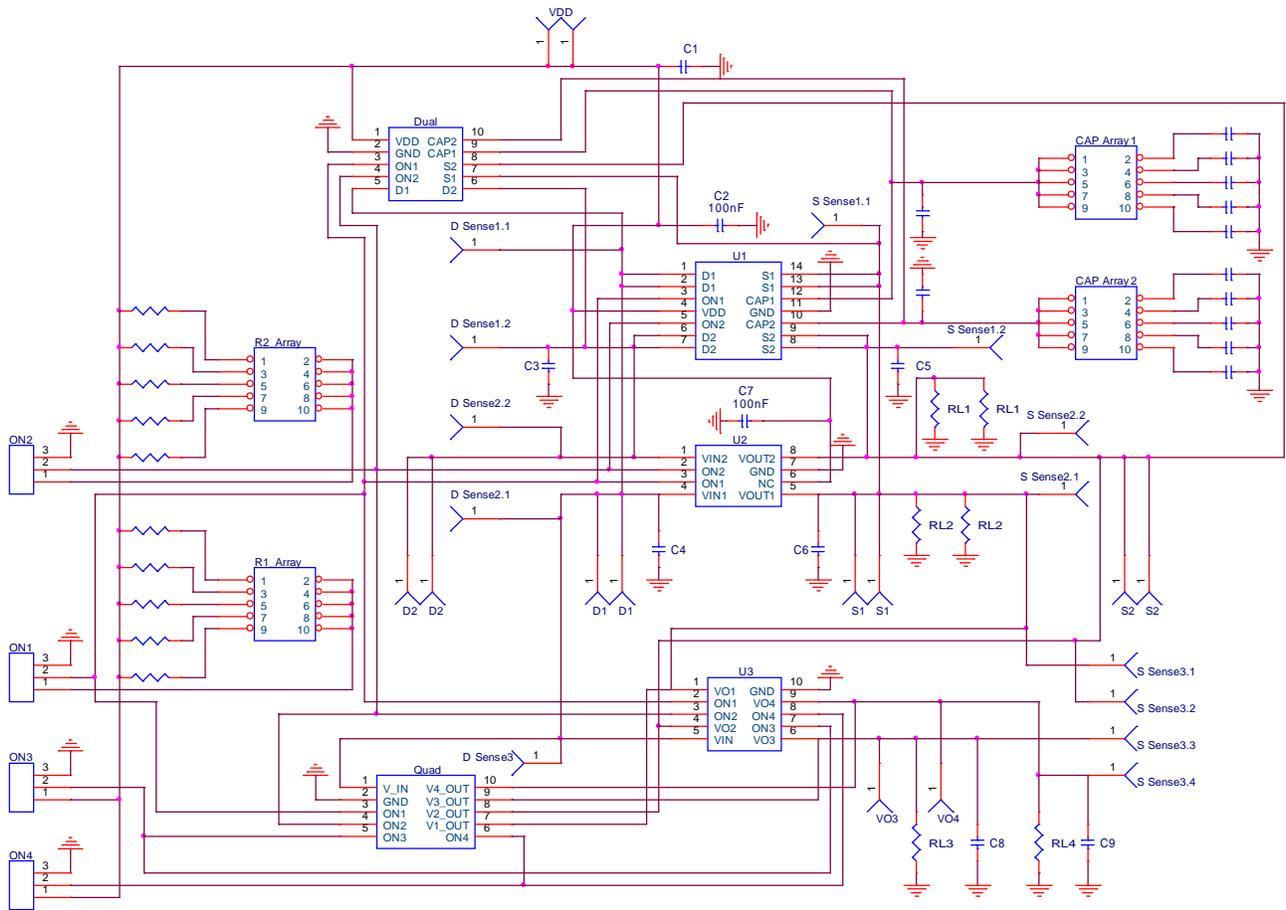
Figure 2. SLG59M1527V Evaluation Board Connection Circuit
