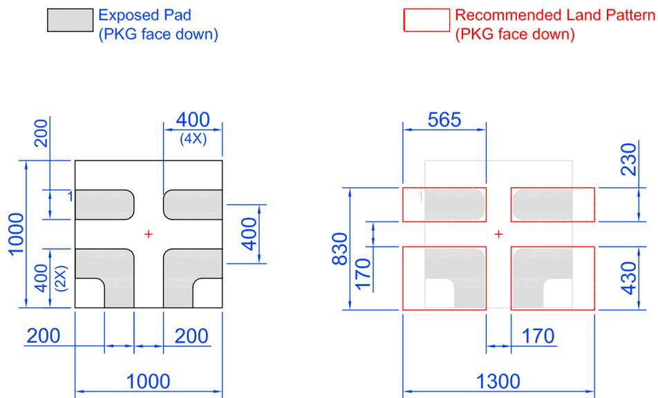
Note: All dimensions shown in micrometers ( $\mu m$ )
