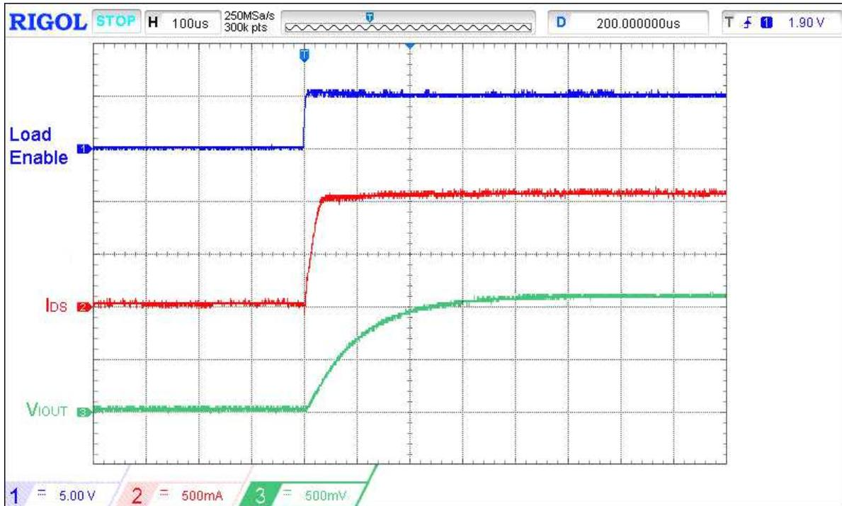
Figure 11. Typical  $I_{OUT}$  response time waveform for  $V_{DD} = V_{IN} = 5\text{ V}$ ,  $C_{LOAD} = 10\text{ }\mu\text{F}$ ,  $R_{LOAD} = 5\text{ }\Omega$ ,  $C_{IOUT} = 0.01\text{ }\mu\text{F}$ ,  $R_{IOUT} = 10\text{ k}\Omega$ , Load Step 0 A to 1 A
