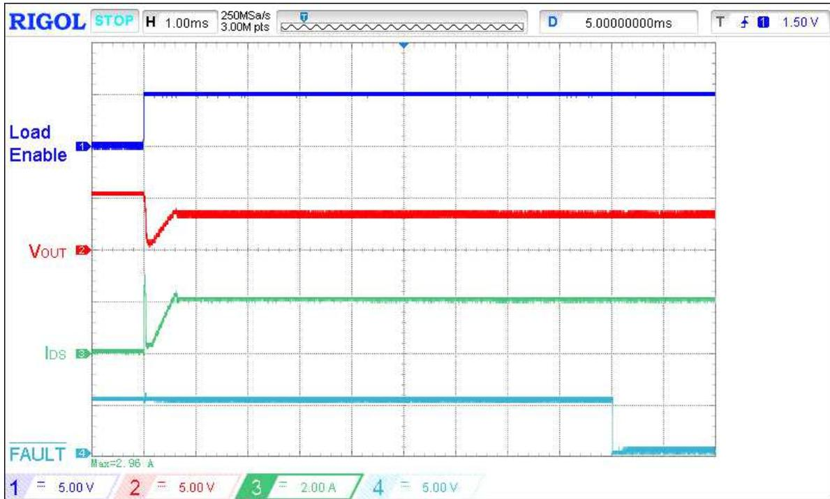
Figure 9. Typical FAULT assertion waveform for  $V_{DD} = V_{IN} = 5\text{ V}$ ,  $C_{LOAD} = 10\ \mu\text{F}$ ,  $I_{ACL} = 2\text{ A}$ ,  $R_{SET} = 40\ \text{k}\Omega$ , switch in  $2\ \Omega$  load
