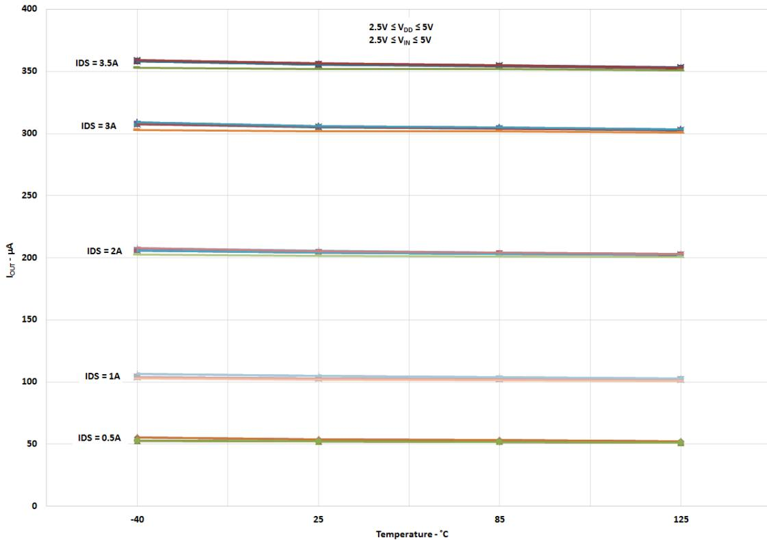
**I<sub>OUT</sub> vs. MOSFET IDS and Temperature**
