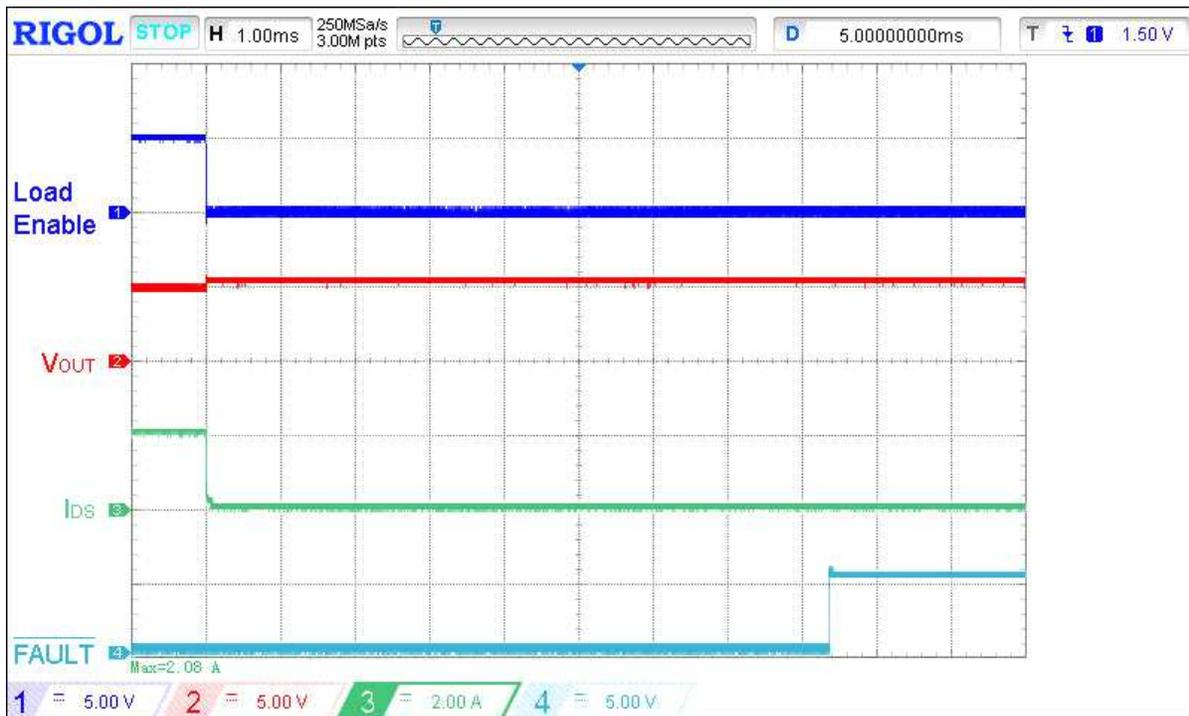
Figure 10. Typical FAULT de-assertion waveform for  $V_{DD} = V_{IN} = 5\text{ V}$ ,  $C_{LOAD} = 10\ \mu\text{F}$ ,  $I_{ACL} = 2\text{ A}$ ,  $R_{SET} = 40\ \text{k}\Omega$ , switch out  $2\ \Omega$  load
