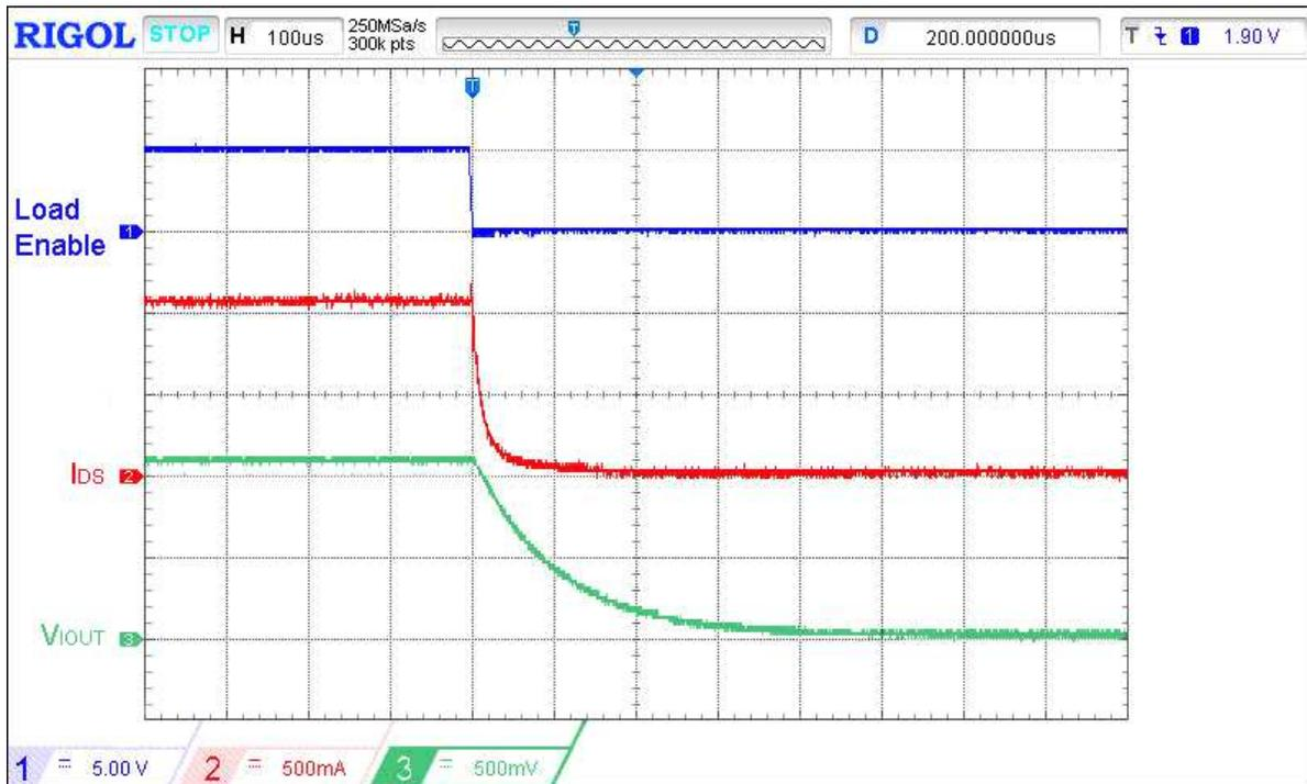
Figure 12. Typical  $I_{OUT}$  response time waveform for  $V_{DD} = V_{IN} = 5\text{ V}$ ,  $C_{LOAD} = 10\text{ }\mu\text{F}$ ,  $R_{LOAD} = 5\text{ }\Omega$ ,  $C_{IOUT} = 0.01\text{ }\mu\text{F}$ ,  $R_{IOUT} = 10\text{ k}\Omega$ , Load Step 1 A to 0 A
