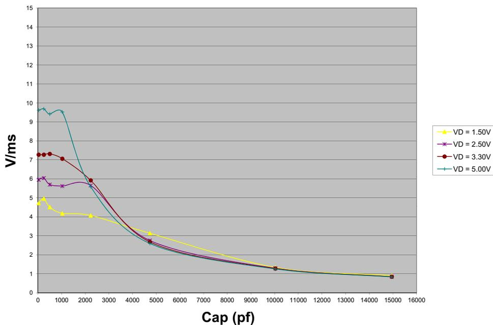
$T_{Total\_ON}$ ,  $T_{ON\_Delay}$  and Slew Rate Measurement
