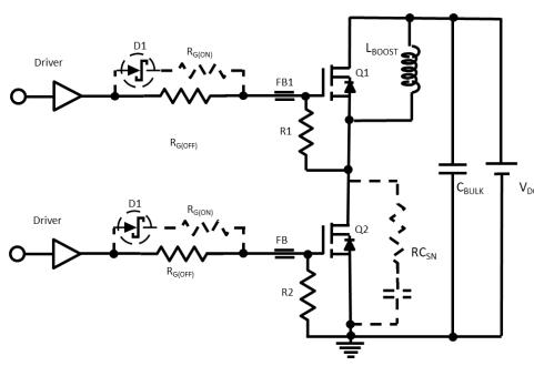
Figure 17. Switching Time Test Circuit
