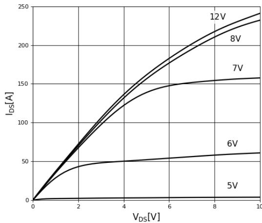
**Figure 3. Typical Output Characteristics,  $T_J = 25^\circ\text{C}$**
