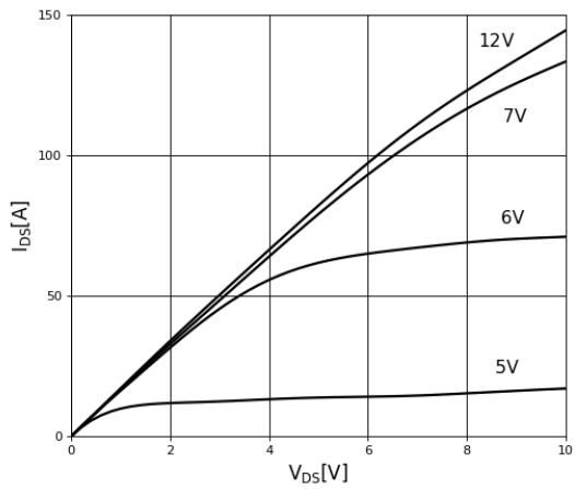
**Figure 4. Typical Output Characteristics,  $T_J = 150^\circ\text{C}$**
