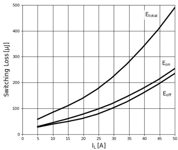
**Figure 16. Inductive Switching Loss  $T_C = 25^\circ\text{C}$**
