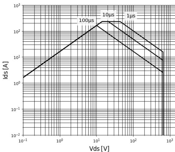
**Figure 15. Safe Operating Area  $T_C = 25^\circ\text{C}$**
