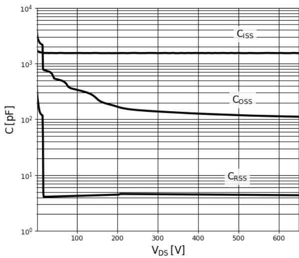
**Figure 7. Typical Capacitance**
