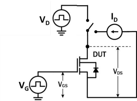
Figure 21. Dynamic  $R_{DS(on)eff}$  Test Circuit
