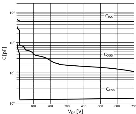
**Figure 8. Typical Capacitance**
