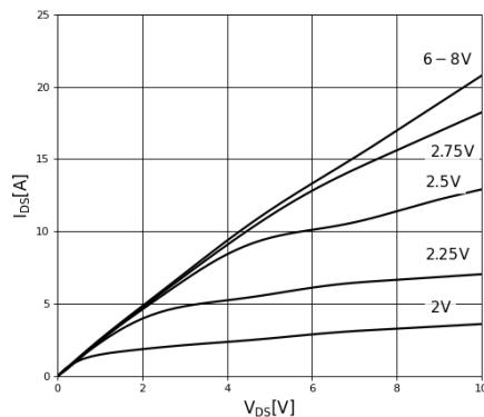
**Figure 5. Typical Output Characteristics,  $T_J = 150^\circ\text{C}$**
