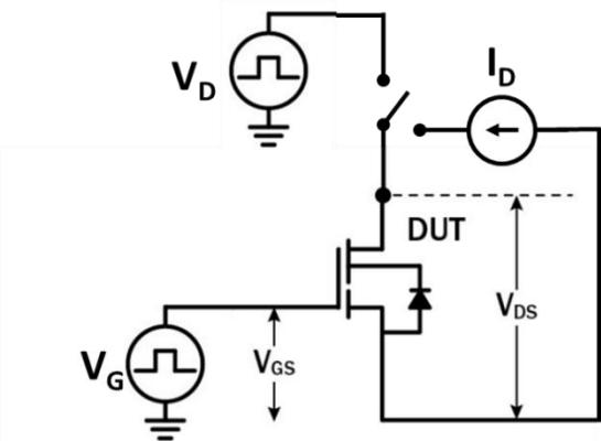
Figure 21. Dynamic  $R_{DS(on)eff}$  Test Circuit
