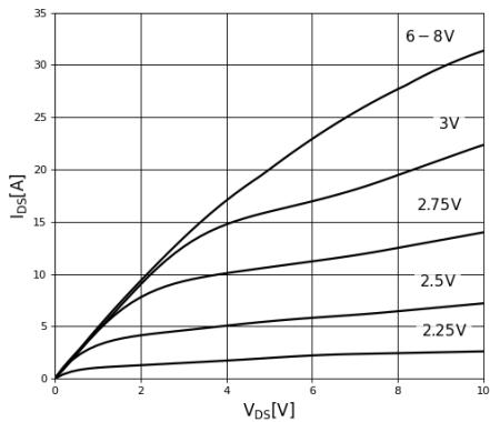
**Figure 4. Typical Output Characteristics,  $T_J = 25^\circ\text{C}$**
