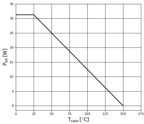
Figure 12. Power Dissipation
