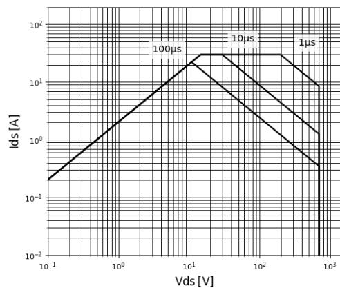
Figure 16. Safe Operating Area  $T_c = 25^\circ\text{C}$
