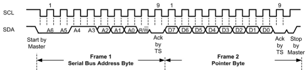
SMBus/I<sup>2</sup>C write to the pointer register followed by a write data word
