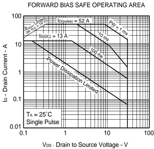
**Remark** Mounted on ceramic substrate of 1200 mm<sup>2</sup> × 0.7 mm
