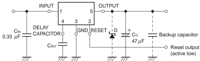
C<sub>IN</sub> : 0.1 μF to 0.47 μF. Determine the capacitance depending on the line between the power supply smoothing circuit and input pin.
