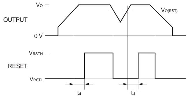
**Remark**  $t_d = 30 \text{ ms TYP. at } C_{DLY} = 0.1 \mu\text{F}$
