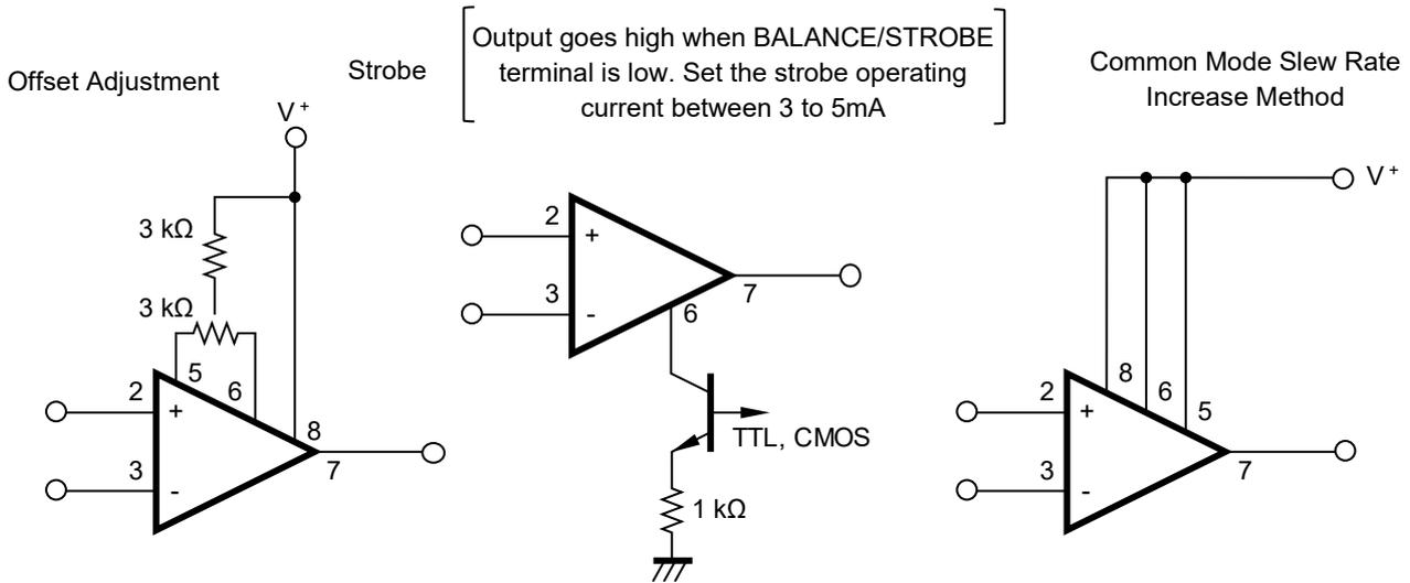
Note Use either pin 5 and pin 6 open (no offset adjustment), the offset adjustment circuit, the strobe circuit (pin 5 open) or the common mode slew rate increase method as shown in above figures. In other cases, malfunction, characteristic deterioration or damage may occur.
