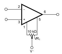
**(Note)** OFFSET NULL pin should be open or connected to V <sup>-</sup> via a resistor as shown above. Any connection other than V <sup>-</sup> may cause malfunction, characteristics degradation or damage.
