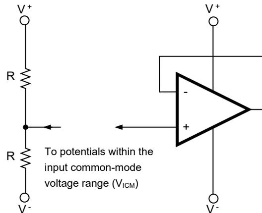
Note in this example, an intermediate voltage of  $V^+$  and  $V^-$  is applied.
