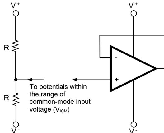
**Remark :** In this example, an intermediate potential between  $V^+$  and  $V^-$  is applied.
