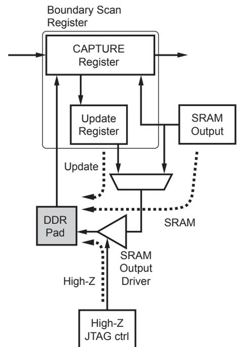
Boundary Scan Register Status of Output Pins CQ, CQ# and DQ
