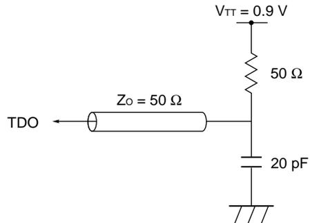
JTAG AC Characteristics (T<sub>A</sub> = 0 to 70°C)
