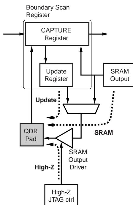
**Boundary Scan Register Status of Output Pins CQ, CQ# and Q**
