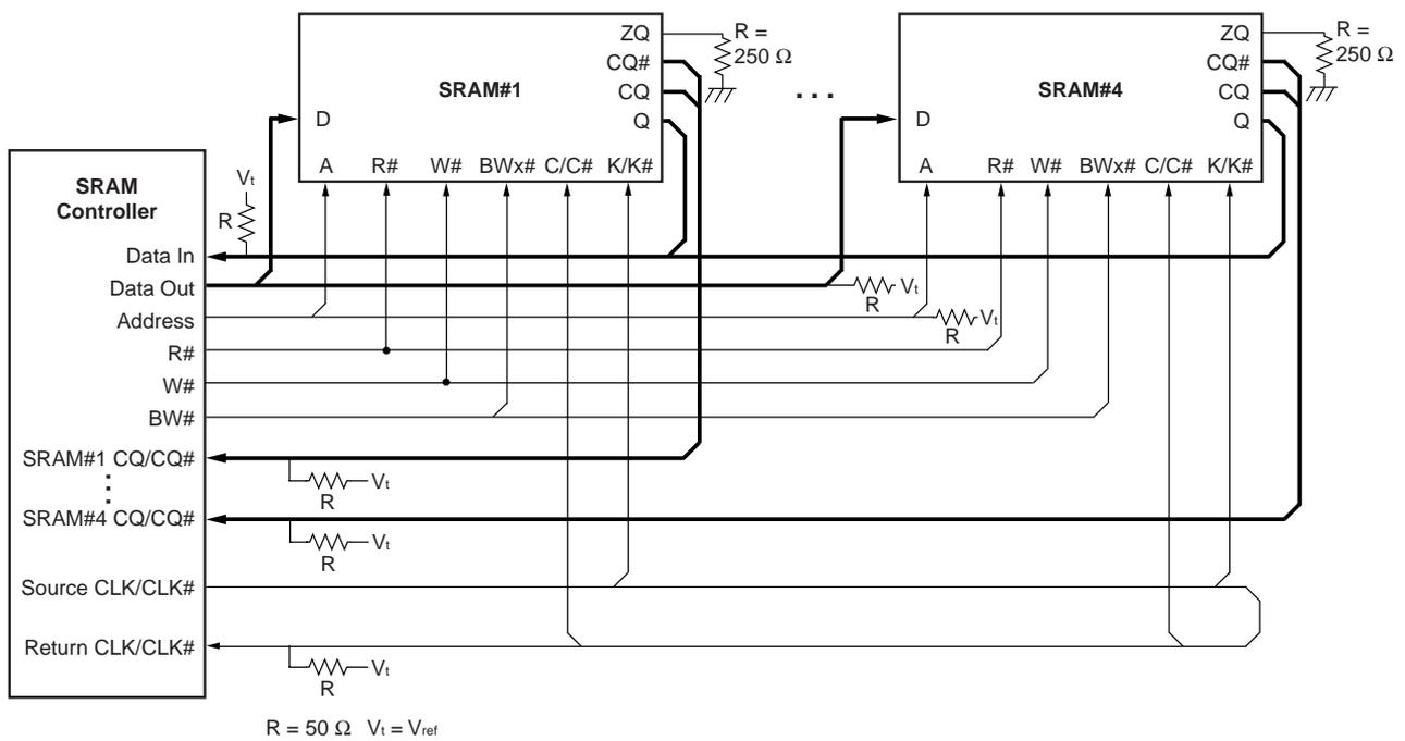
**Remark** AC Characteristics are defined at the condition of SRAM outputs, CQ, CQ# and Q with termination.
