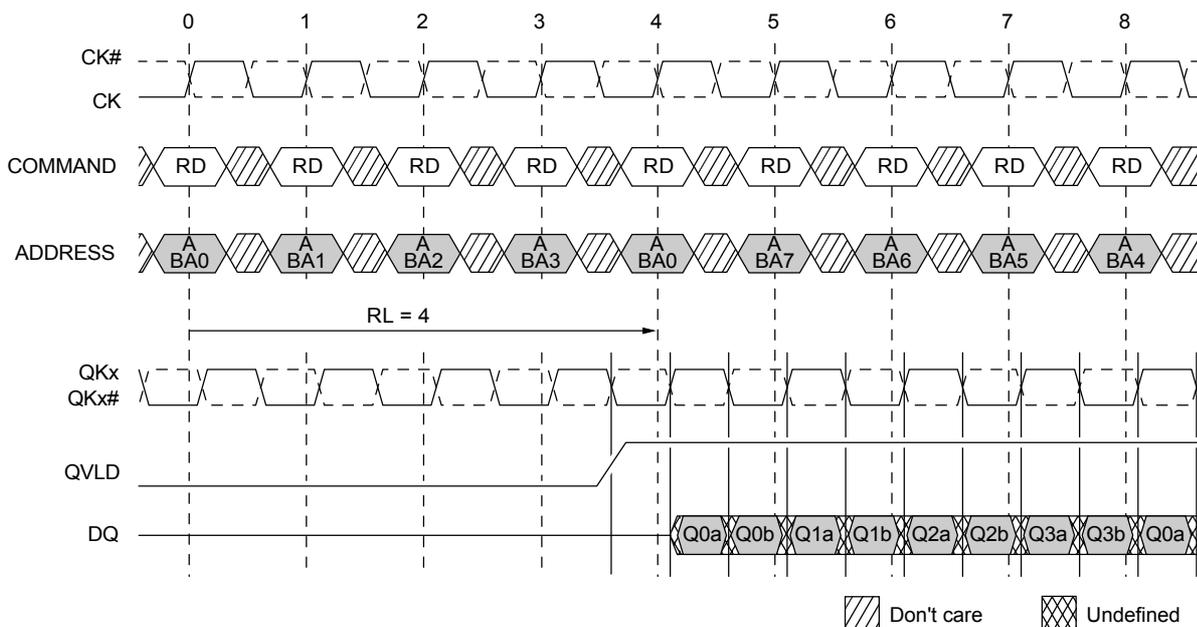
Figure 2-15. READ Burst Basic Sequence: BL=4, RL=4, Configuration 1
