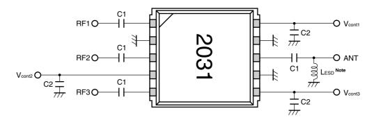
**Note** Recommend attached Lesp to antenna port for ESD protection.
