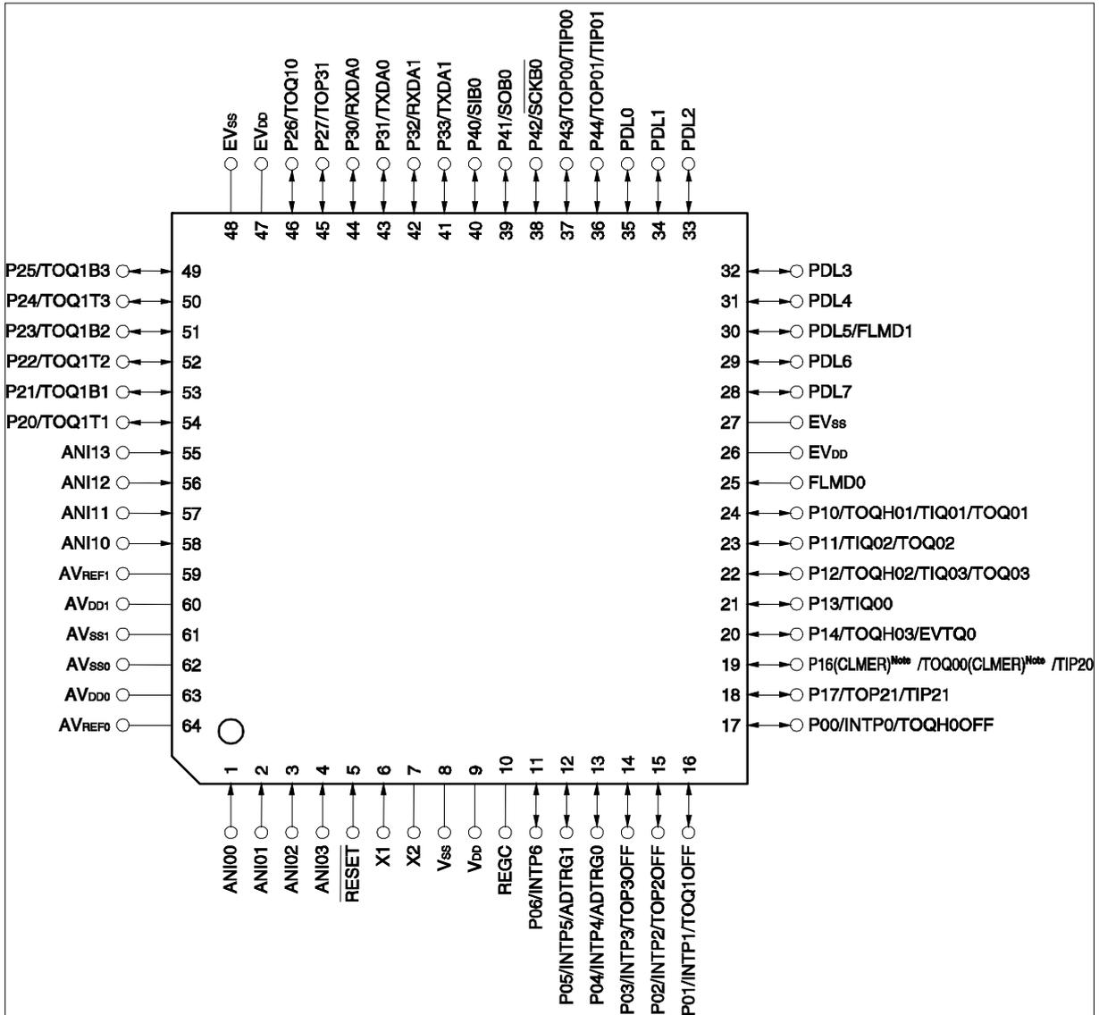
**Notes** The CLMER signal is enabled only when P16 is specified as an output port or the output function of TOQ00. When an error (oscillator stop) is detected by the clock monitor, a low level is forcibly output. Low-level output is released by reset signal.
