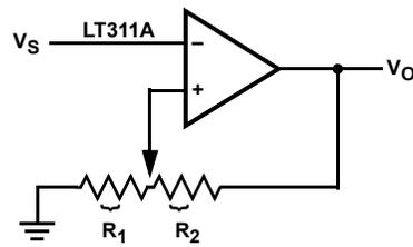
$$V_{UL} = \{R_1/(R_1+R_2)\} V_O(\text{max})$$
