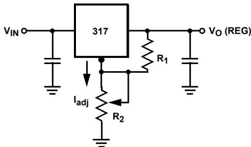
$$V_O \text{ (REG)} = 1.25V (1+R_2/R_1)+I_{adj} R_2$$
