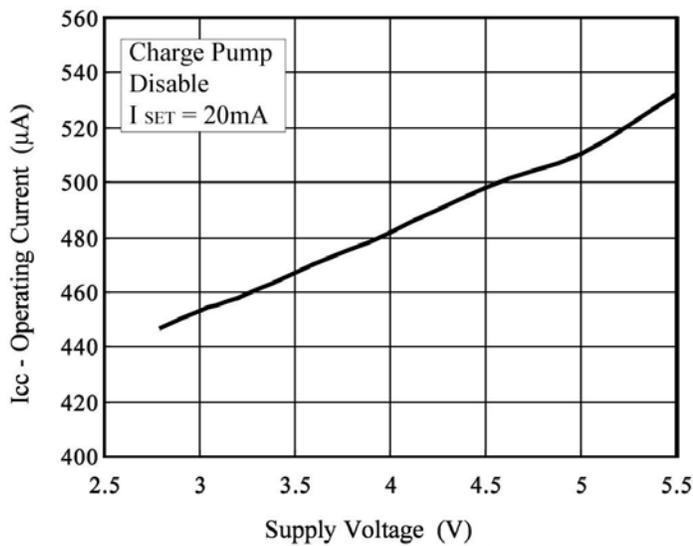
**Figure 1.2 LED Current over Supply Voltage  $V_{CC}$  Range (2.8V to 5.5V) for Outputs D0:D5 (LED0:LED5)**
