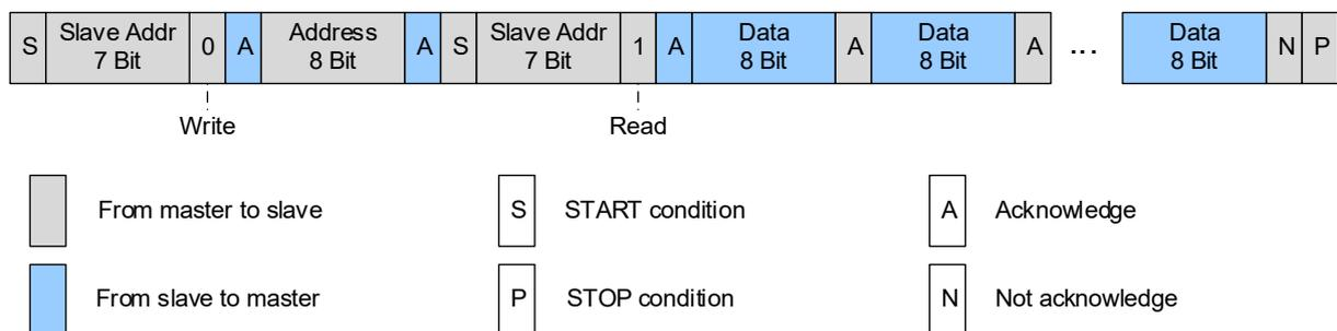
Figure 15. I<sup>2</sup>C Data Transmission Protocol
