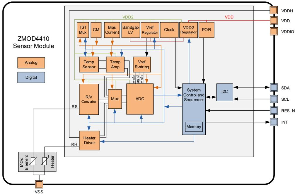
Figure 2. Block Diagram
