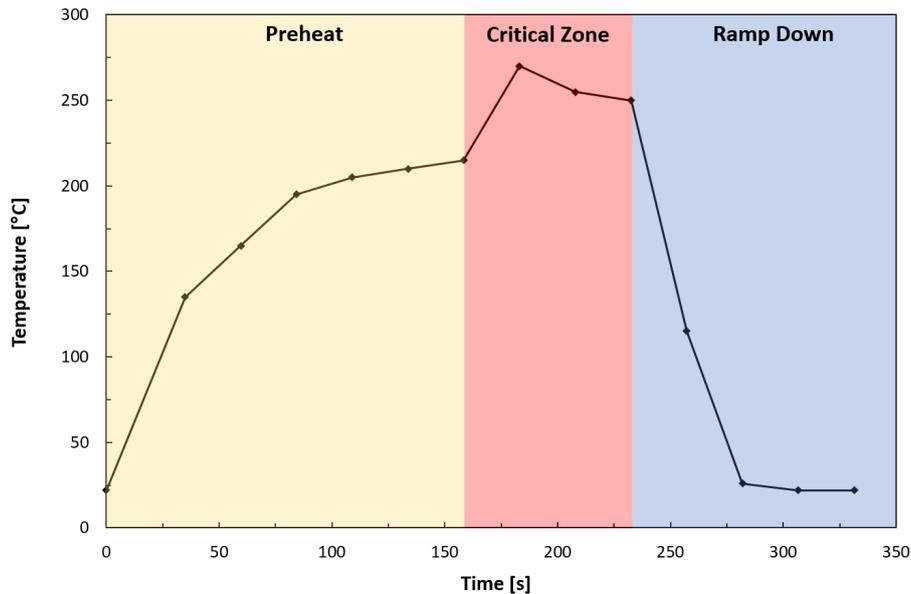
Figure 14. Typical Solder Profile
