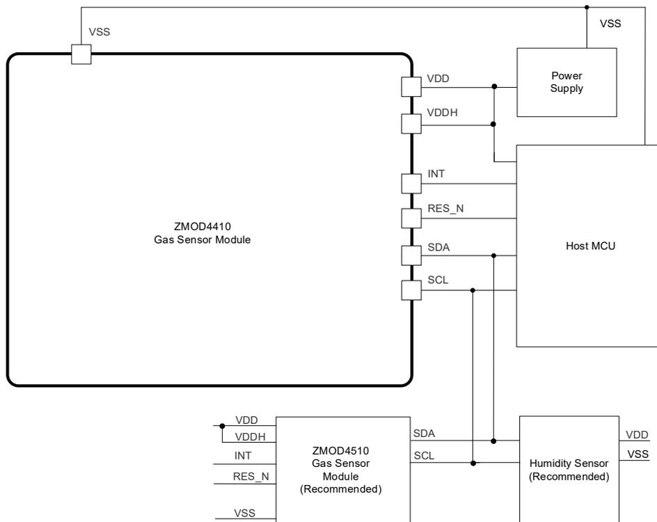
Figure 3. Application Circuit
