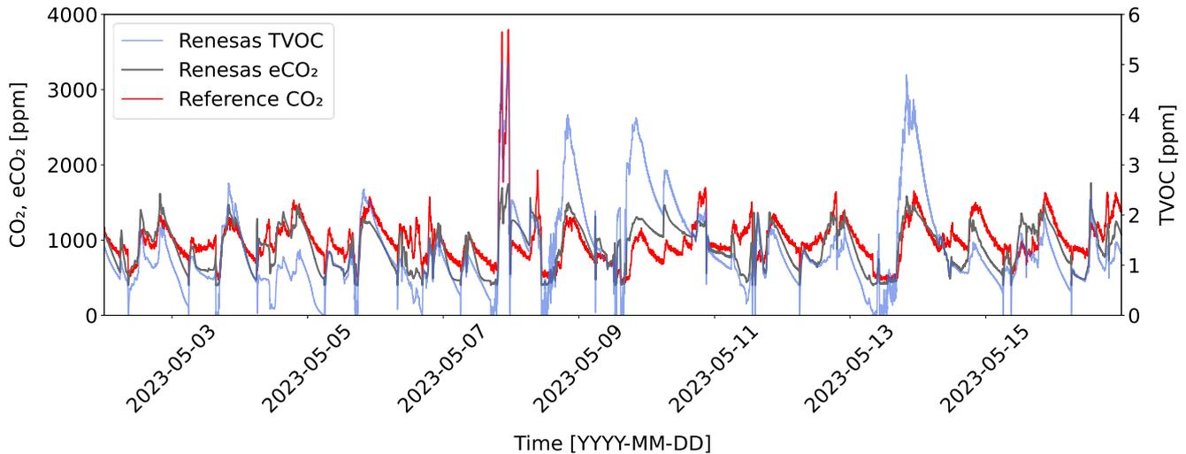
Figure 8. Typical Graph of CO<sub>2</sub> Estimation in an Application
