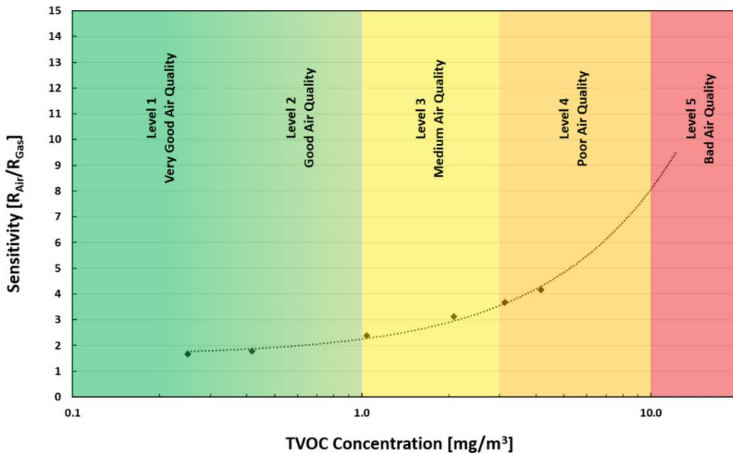
Figure 9. Typical ZMOD4410 Response to Levels of TVOC Described by UBA Using EPA Standard Mixture
