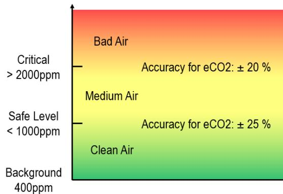
Figure 11. Concentration Dependent Accuracy for eCO2<sup>6</sup>
