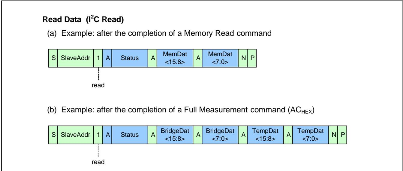
All mandatory I<sup>2</sup>C™ bus protocol features are implemented. Optional features like clock stretching, 10-bit slave address, etc., are not supported by the ZSSC3016's interface.
