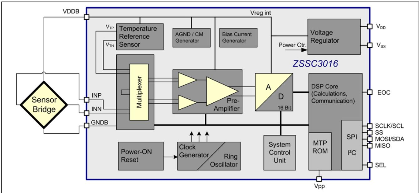
The amplifier consists of two stages with programmable gain values. The 1/f noise and inherent offset are suppressed by auto-zero and chopper stabilizer techniques. This auto-zero sequence is performed before each bridge sensor and temperature measurement to compensate for the inherent offset of the amplifier.
