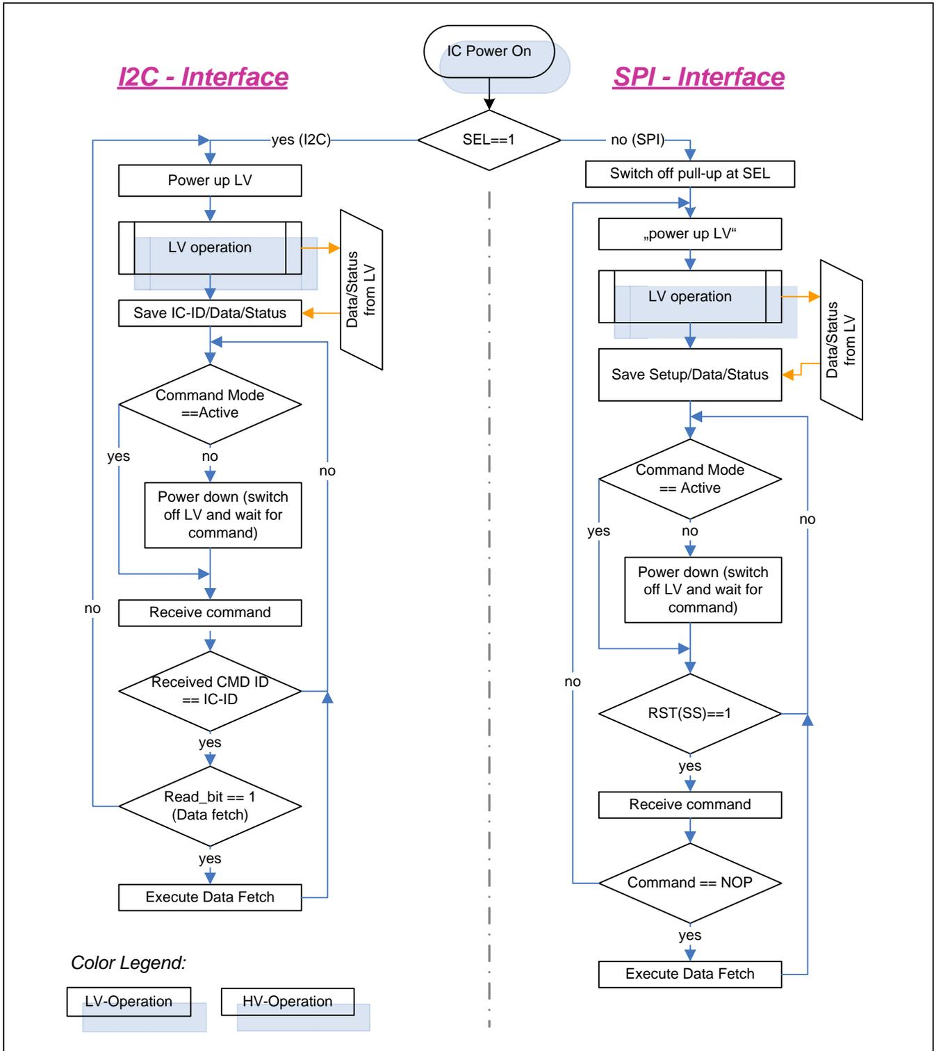
Figure 3.2 Operational Flow Chart: Command Mode and Normal Mode
