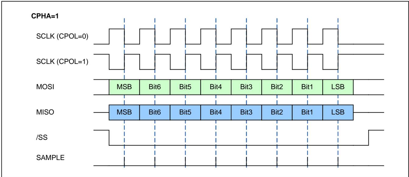
In SPI mode, each command except NOP is started as shown in Figure 3.5. After the execution of a command (busy = 0), the expected data can be read as illustrated in Figure 3.6 or if no data are returned by the command, the next command can be send. The status can be read at any time with the NOP command (see Figure 3.7
