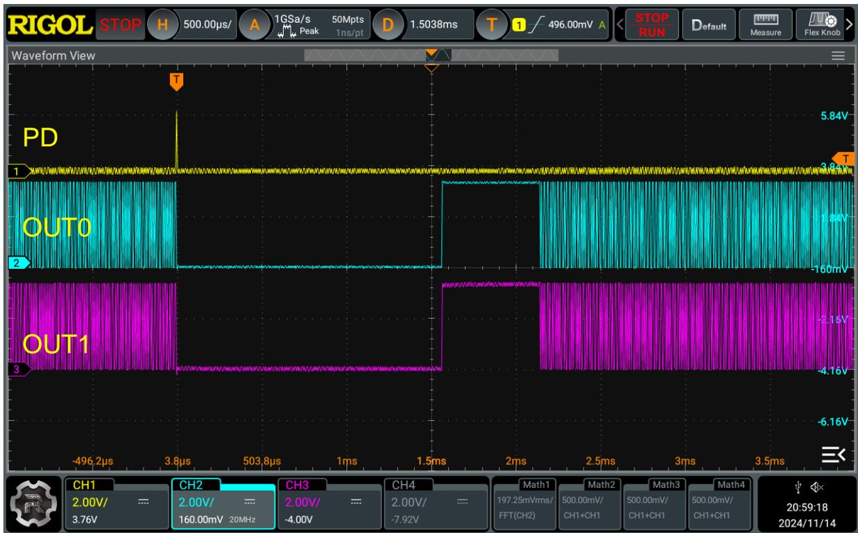
Figure 17. 2 MHz OSC Long Start-Up
