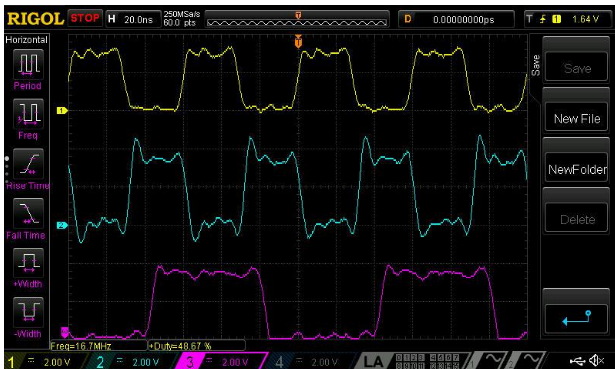
Figure 9. Output Waveforms at Period = 60 ns, Pulse Width = 30 ns, DC = 50 % (Incorrect Functionality)
