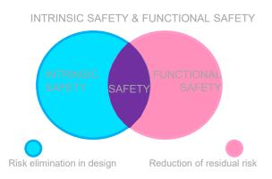
Functional safety defines application specific risks, and the requirements to minimize these via the control system for specific end applications. Functional Safety is based on the premise that things break and fail, perfect software is impossible, and people make mistakes. Functional safety's objective is to keep these risks (residual risks that cannot be eliminated at the design stage) to people, equipment, property, and the environment below acceptable limits through "functionality".
