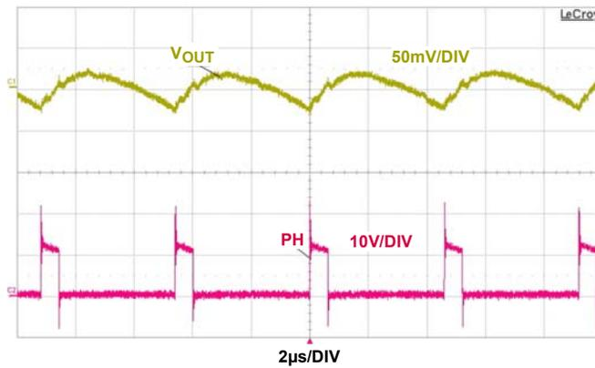
FIGURE 10. OUTPUT VOLTAGE RIPPLE AT 30A LOAD CONDITION
