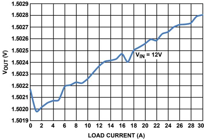
FIGURE 6.  $V_{OUT}$  LOAD REGULATION AT CCM MODE
