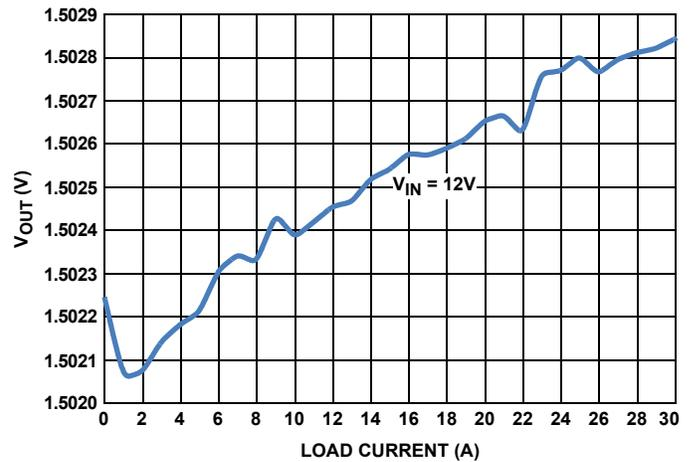
FIGURE 7.  $V_{OUT}$  LOAD REGULATION AT DEM MODE
