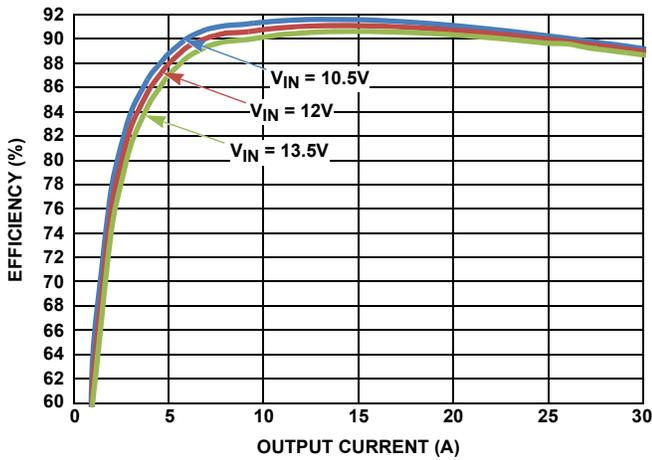
FIGURE 4. EFFICIENCY vs LOAD CURRENT AT CCM MODE
