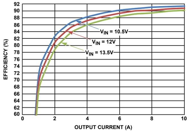
FIGURE 5. EFFICIENCY vs LOAD CURRENT AT DEM MODE
