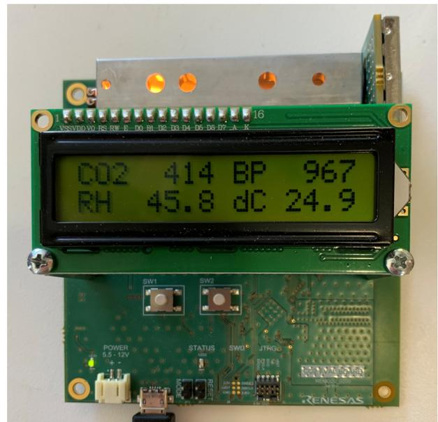
Two pushbuttons are used for viewing additional information and calibrating the board. **Sw1** cycles through displaying available modes and **Sw2** selects the currently displayed mode for further operations.
