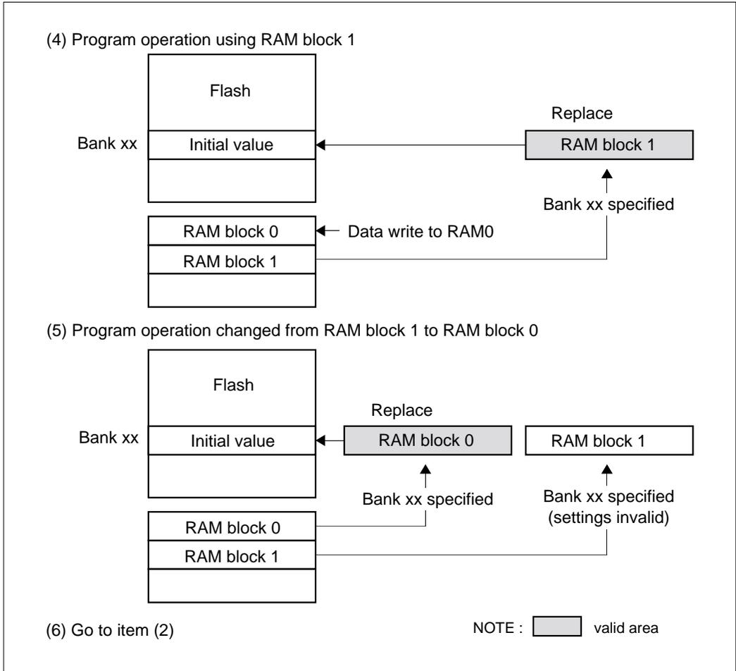
Figure 6.7.16 Application Example of Virtual Flash Emulation (2/2)
