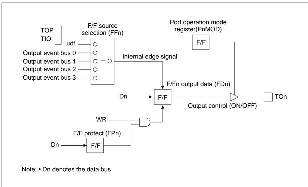
**Figure 10.2.3 Configuration of the F/F Output Circuit**
