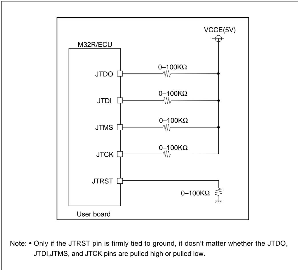
Figure 19.7.1 Processing Pins when Not Using JTAG
