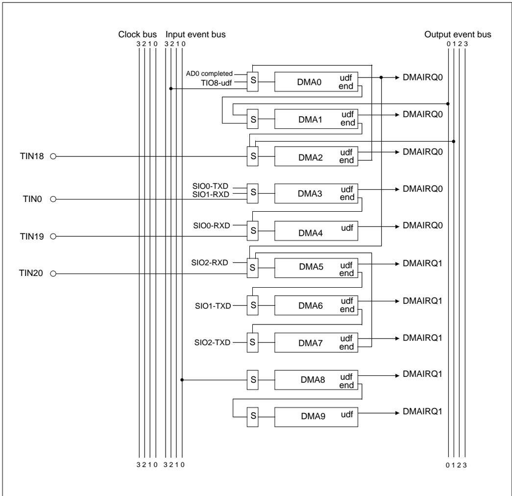
Figure 9.1.2 Causes of DMAC Requests Connection Diagram
