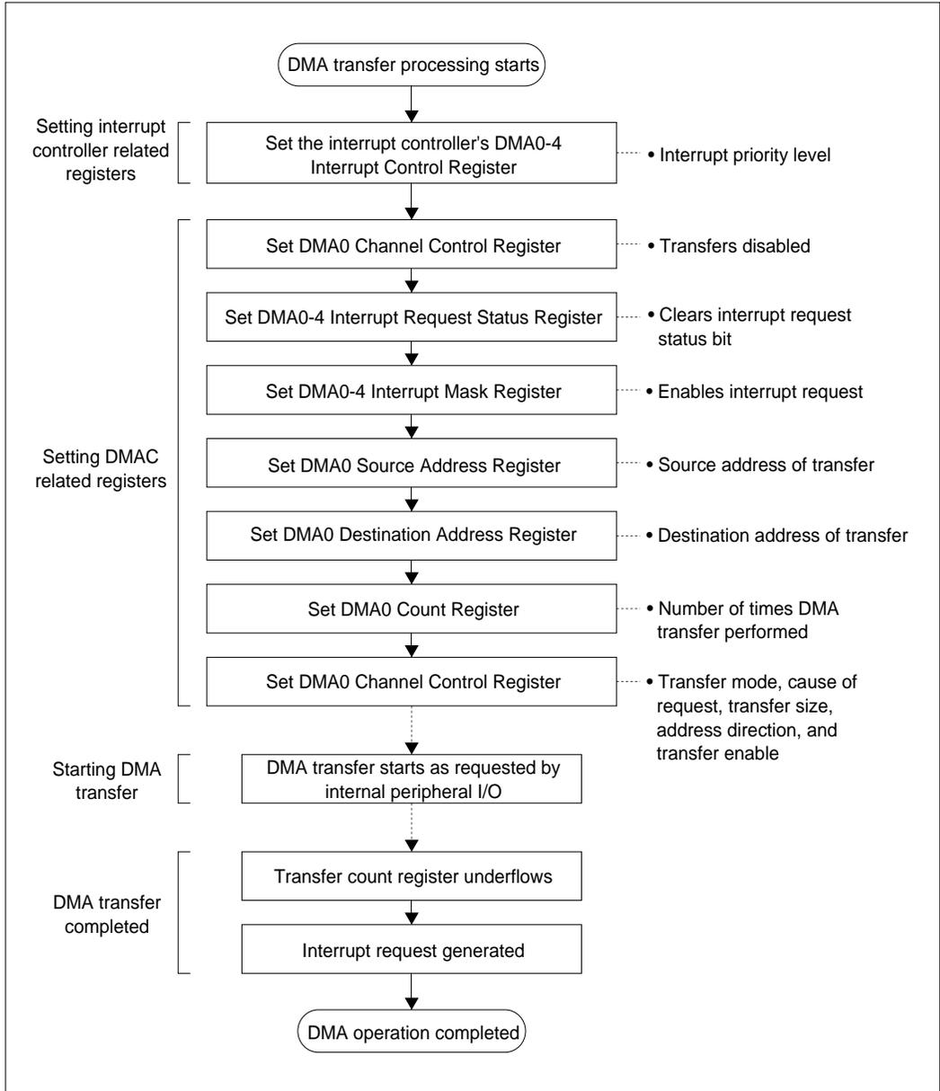
Figure 9.3.1 Example of a DMA Transfer Processing Procedure
