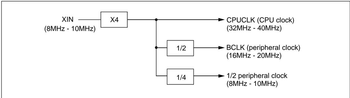
Figure 1.1.1 Conceptual Diagram of the Clock Frequency Multiplier
