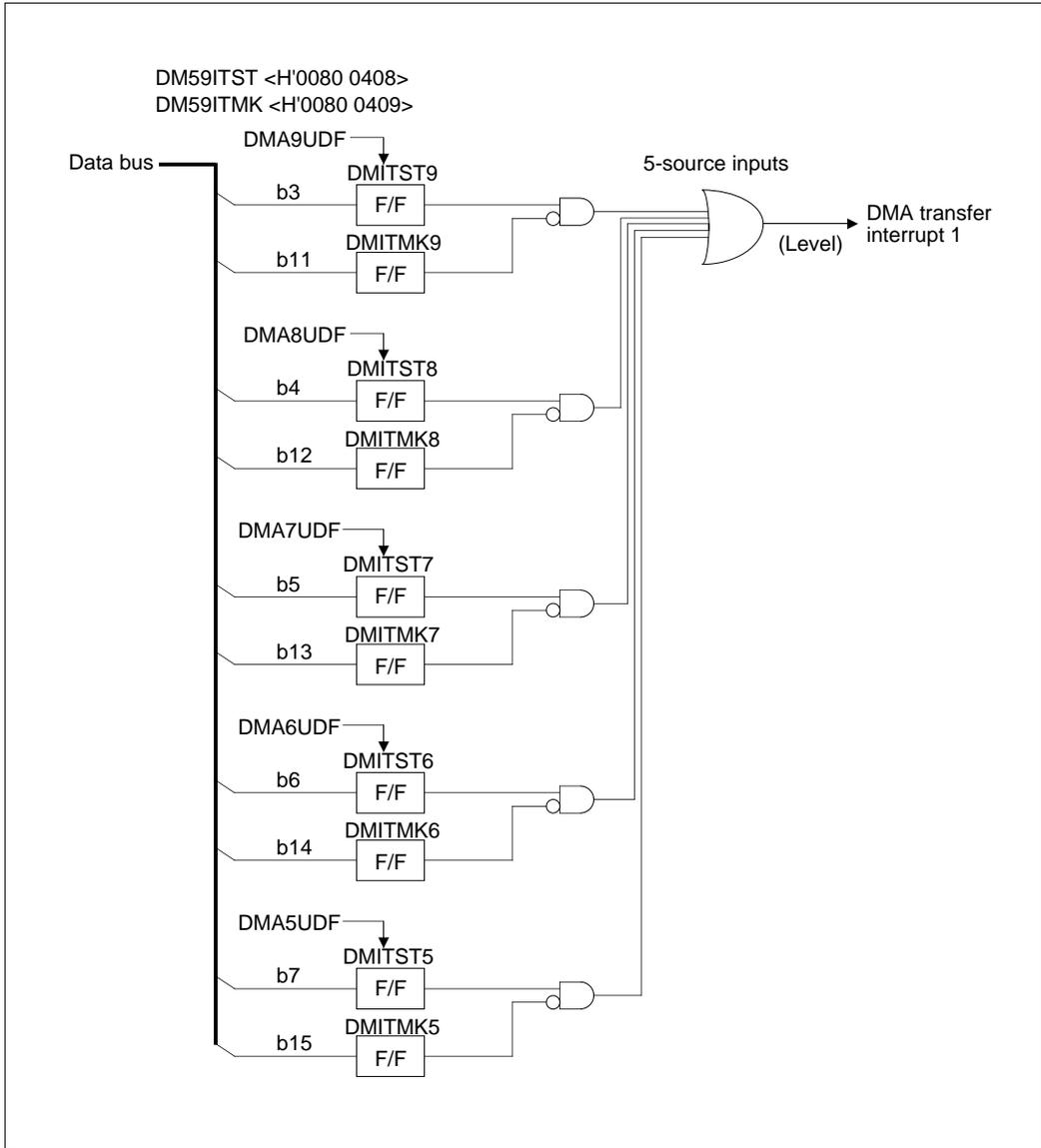
Figure 9.2.4 Block Diagram of DMA Transfer Interrupt 1
