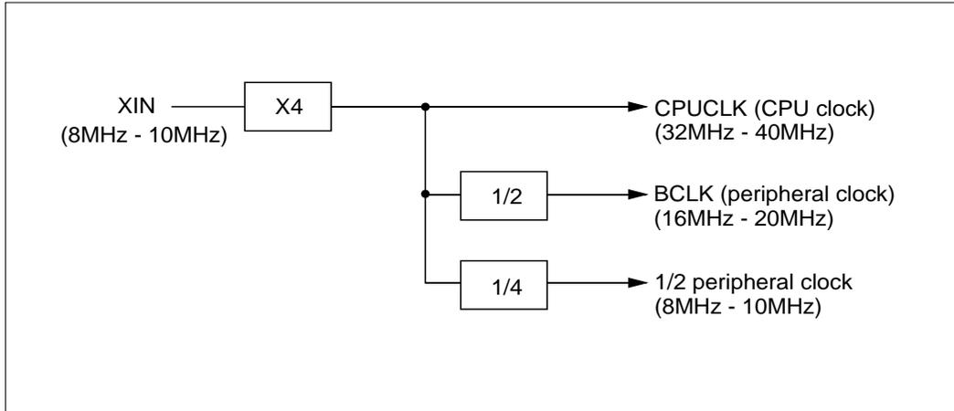
Figure 18.2.1 Configuration of the Clock Generator Circuit
