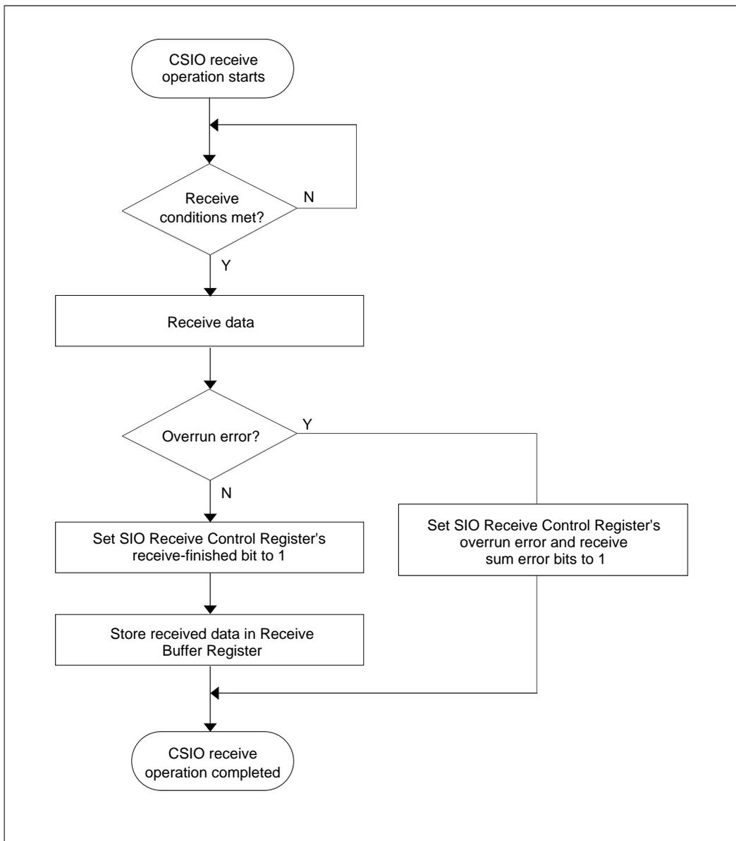
Figure 12.4.2 Receive Operation during CSIO Mode (Hardware Processing)
