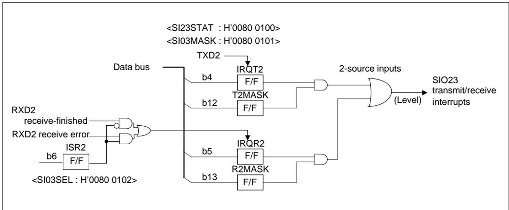
Figure 12.2.4 Block Diagram of SIO23 Transmit Interrupts
