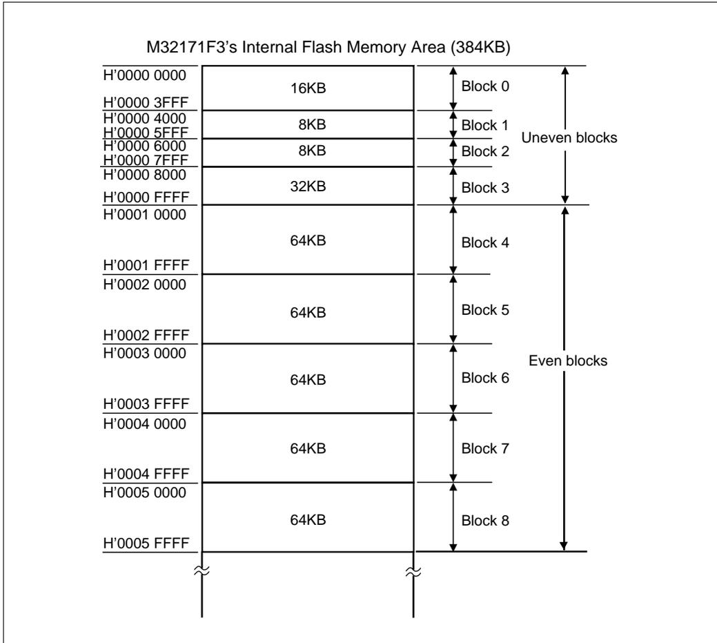
Figure 6.5.8 Block Configuration of the M32171F3 Flash Memory
