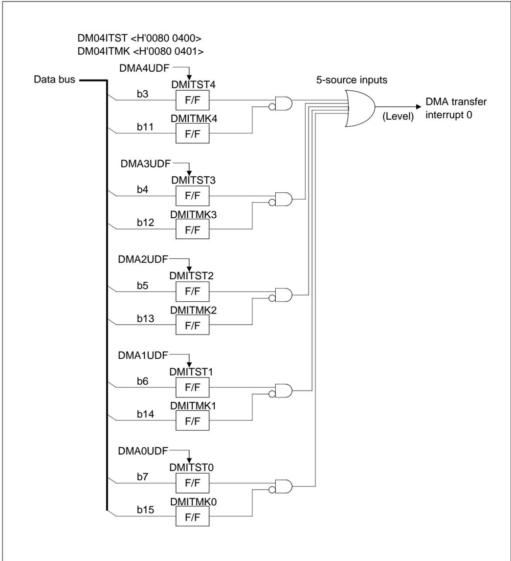
Figure 9.2.3 Block Diagram of DMA Transfer Interrupt 0
