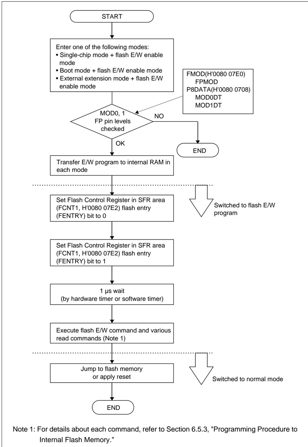
Figure 6.5.6 Procedure for Entering Flash E/W Enable Mode
