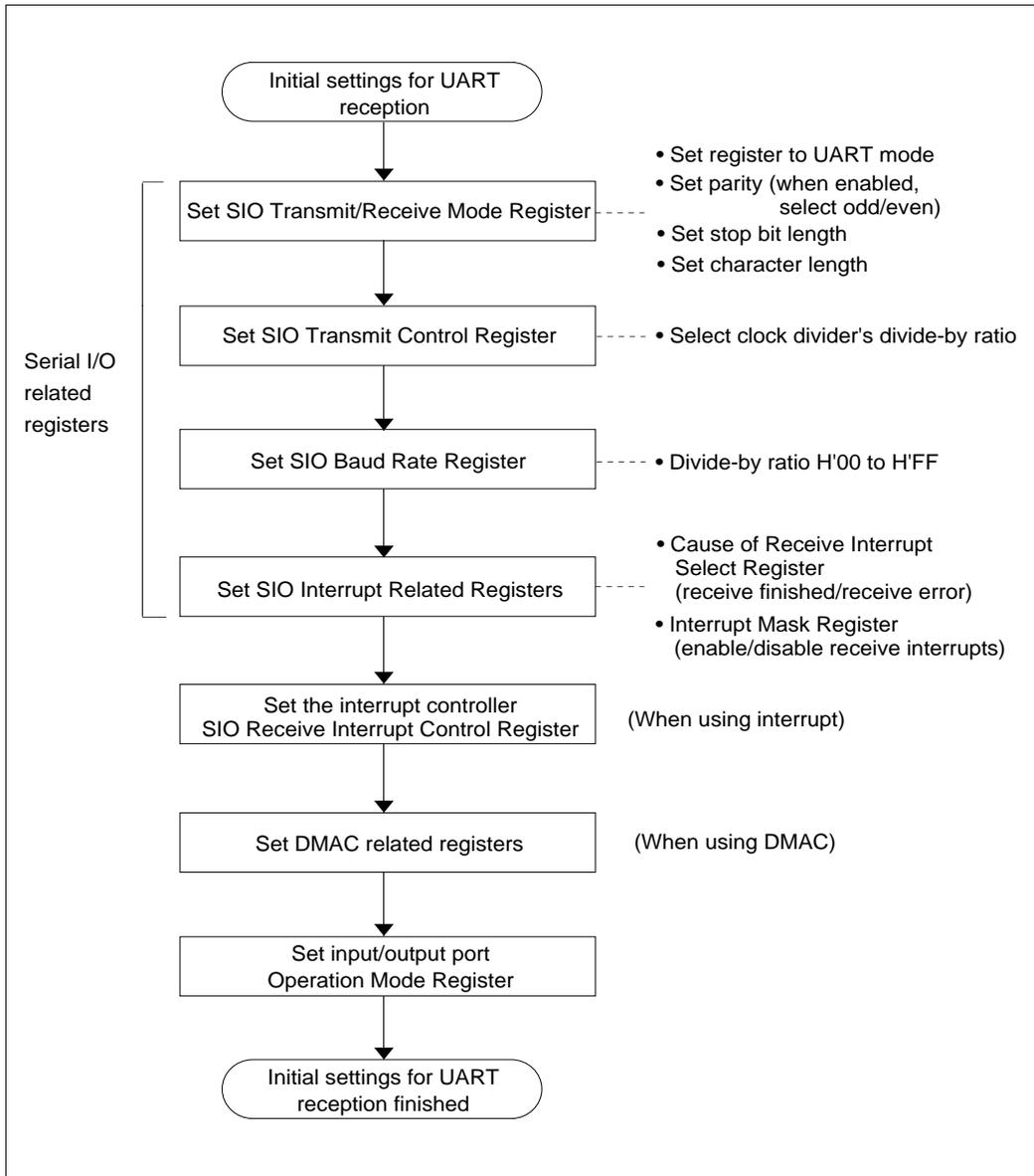
Figure 12.7.1 Procedure for UART Receive Initialization
