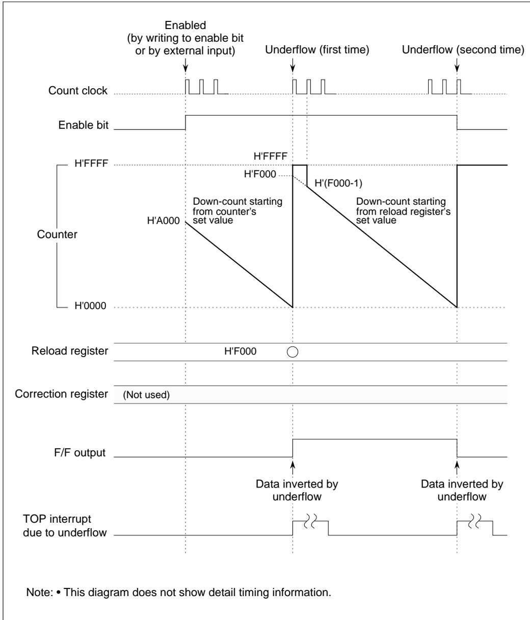
Figure 10.3.16 Typical Operation in TOP Delayed Single-shot Output
