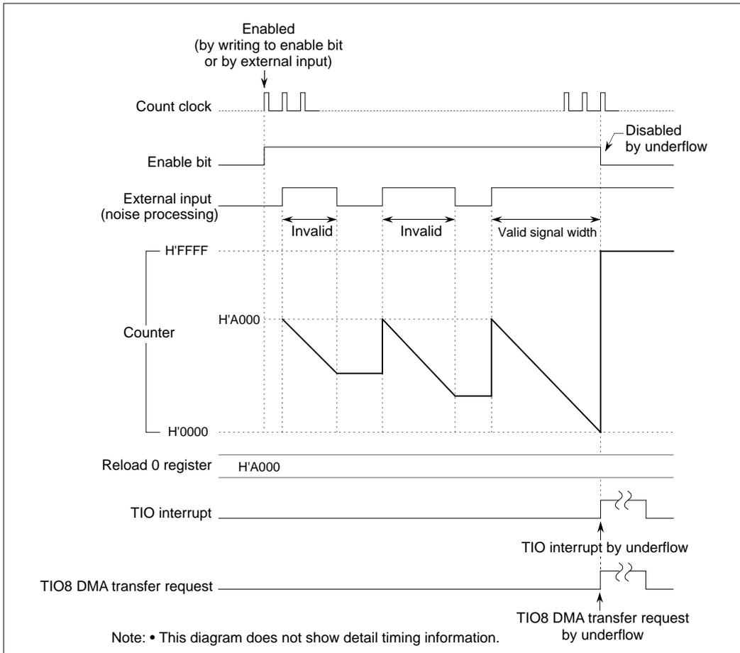
Figure 10.4.11 Typical Operation in Noise Processing Input Mode
