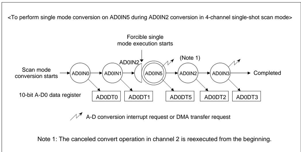
Figure 11.1.6 Forcible Single Mode Execution during Scan Mode
