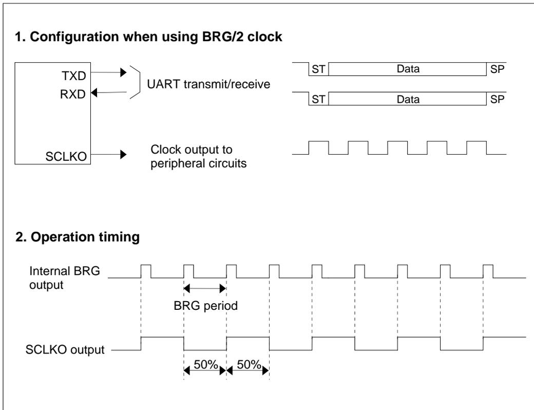
Figure 12.8.1 Example of Fixed Period Clock Output
