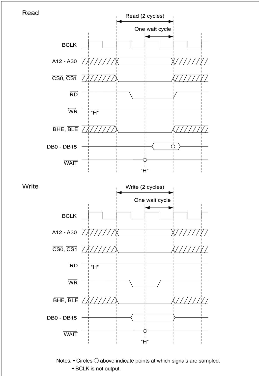
Figure 15.2.5 Read/Write Timing (for Shortest-case External Access)
