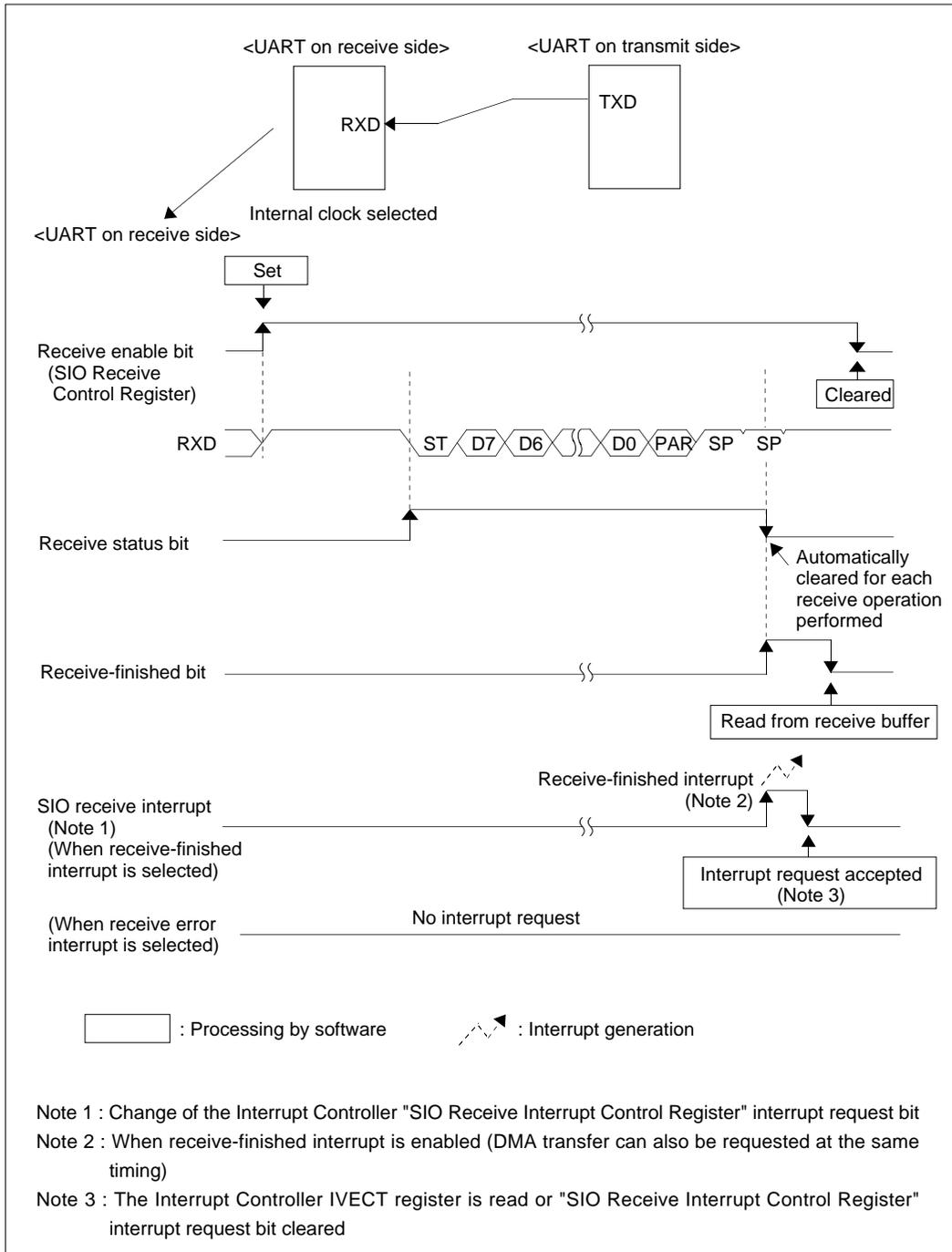
Figure 12.7.3 Example of UART Reception (When Received Normally)
