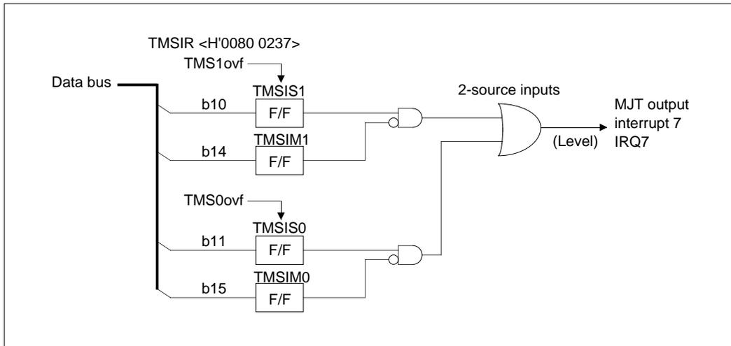
Figure 10.2.12 Block Diagram of MJT Output Interrupt 7
