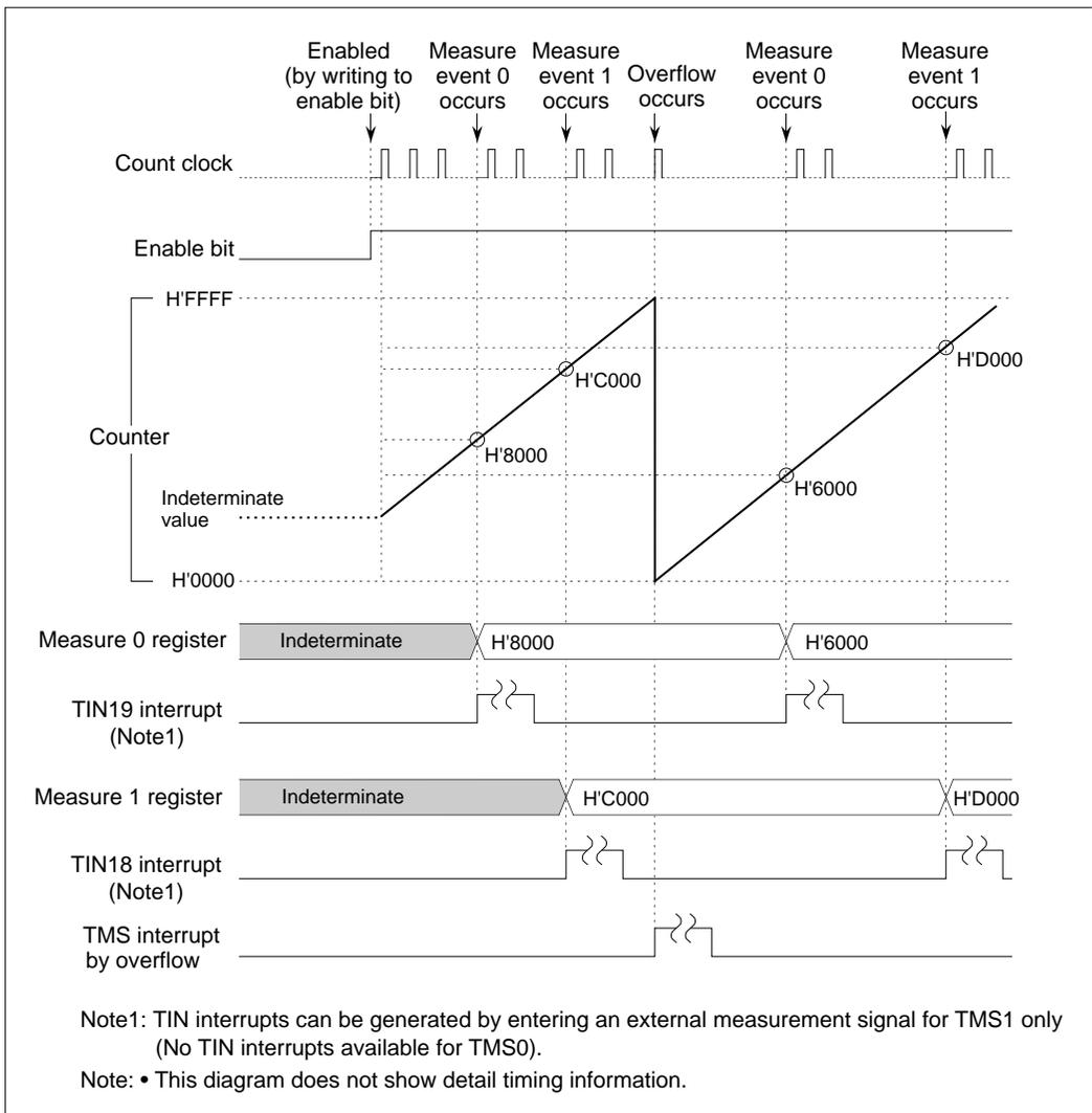
Figure 10.5.4 Typical Operation in TMS Measure Input
