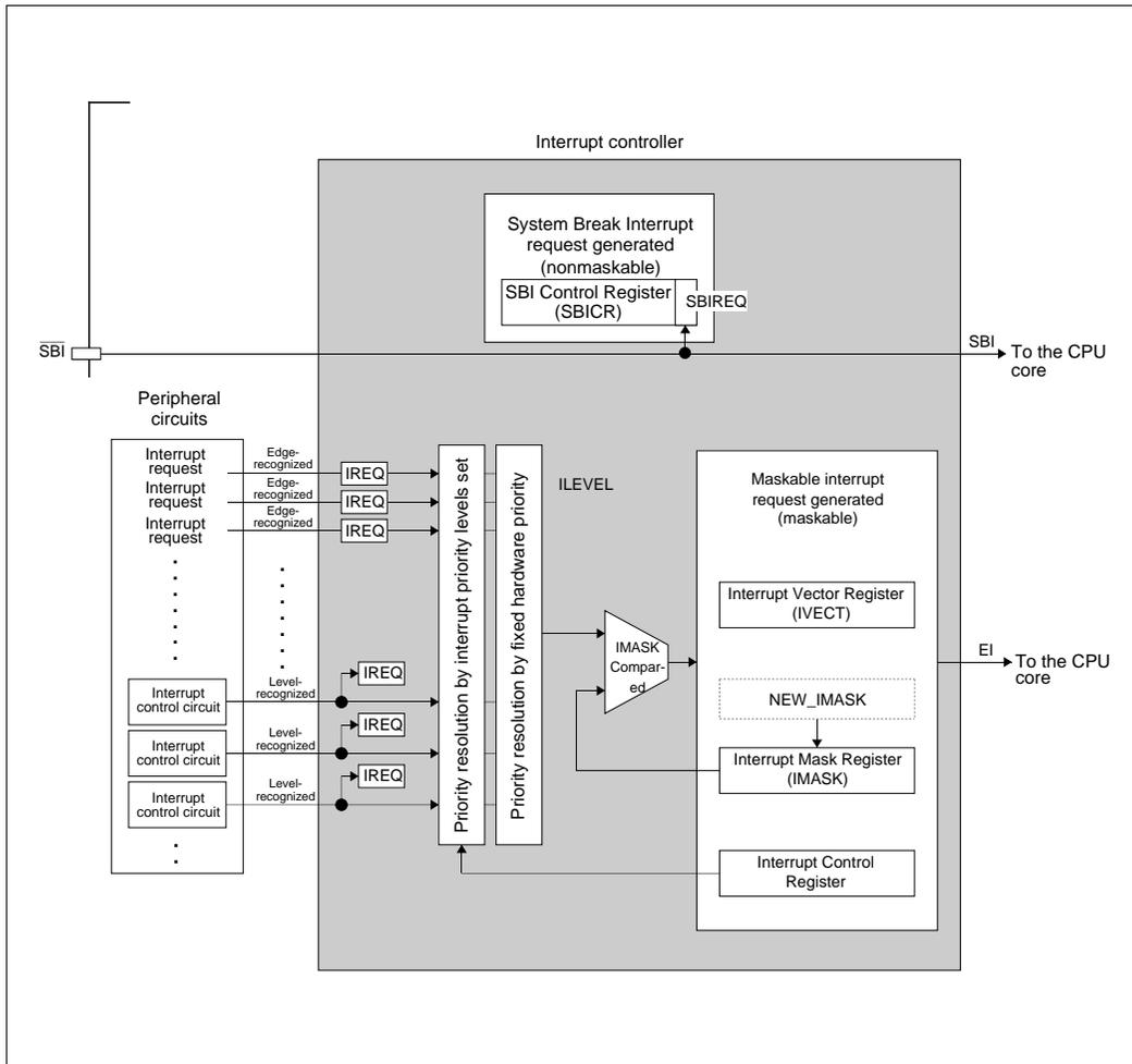
Figure 5.1.1 Block Diagram of the Interrupt Controller
