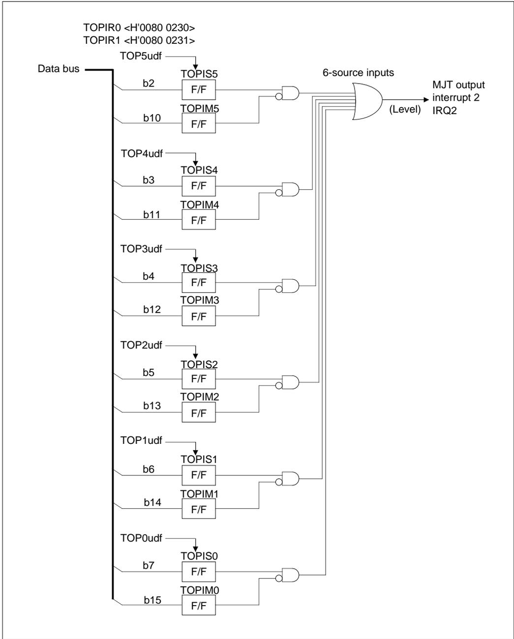
Figure 10.2.6 Block Diagram of MJT Output Interrupt 2
