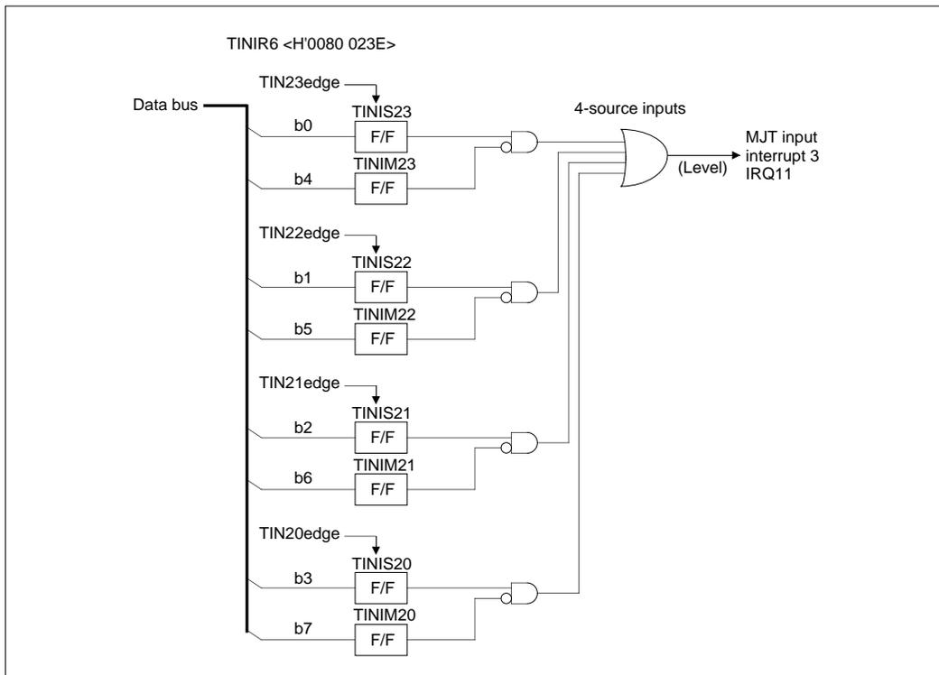
Figure 10.2.16 Block Diagram of MJT Input Interrupt 3
