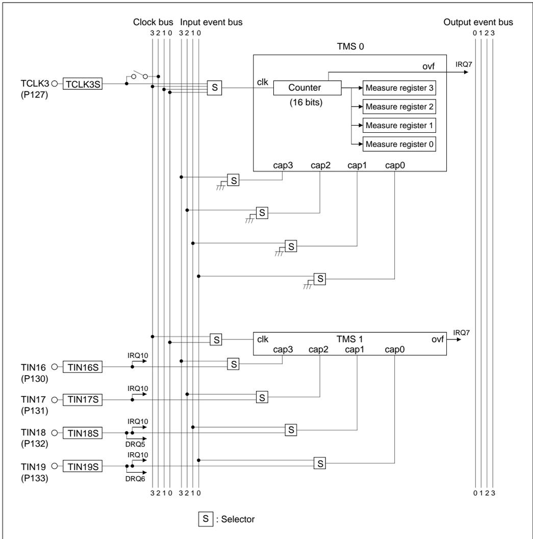
Figure 10.5.1 Block Diagram of TMS (Input-related 16-bit Timer)
