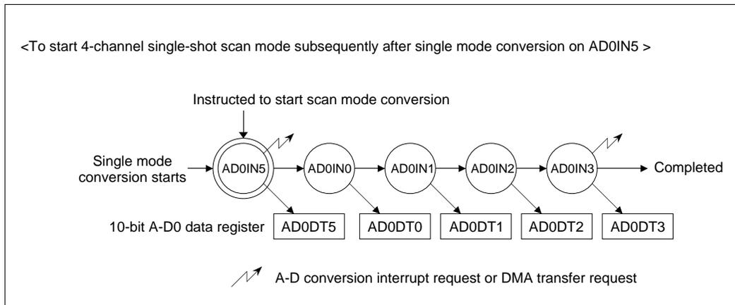
**Figure 11.1.7 Scan Mode Start after Single Mode Execution**
