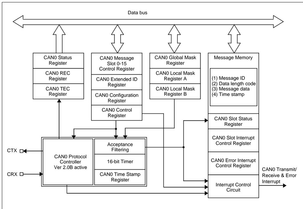
**Figure 13.1.1 Block Diagram of the CAN Module**
