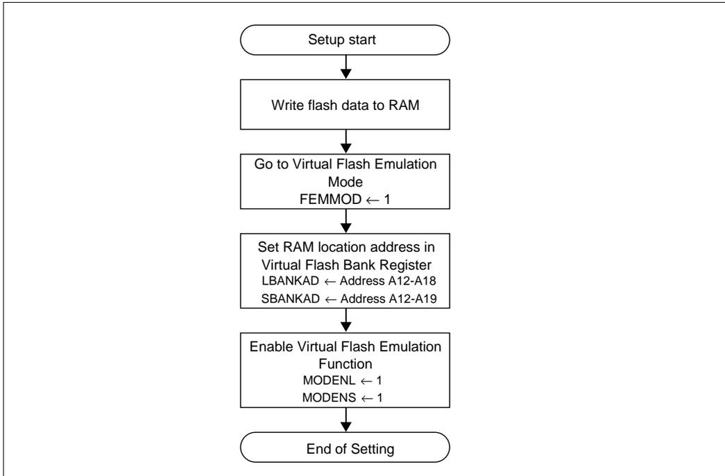
Figure 6.7.14 Virtual-flash Emulation Mode Sequence
