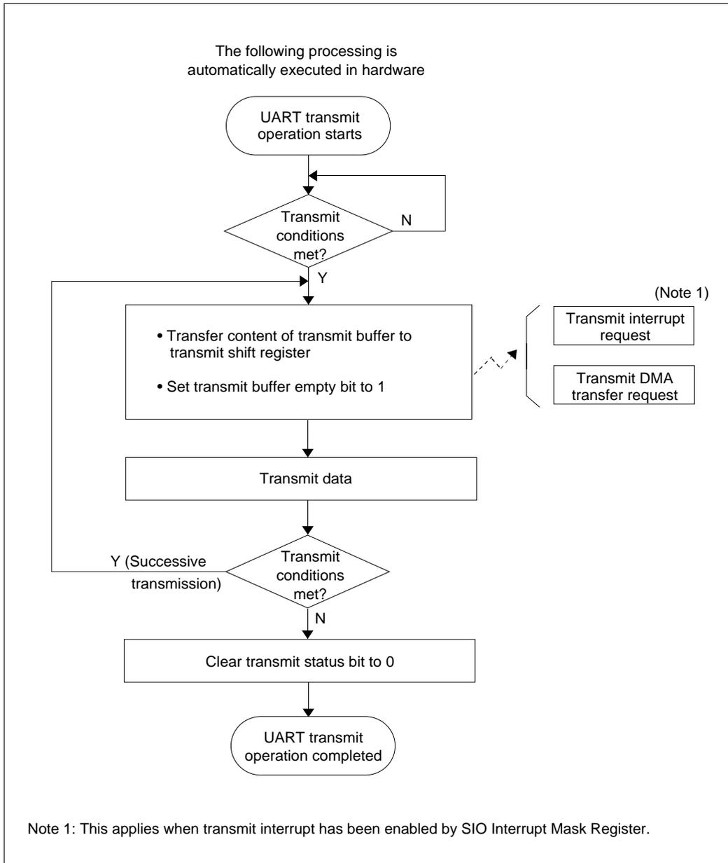
**Figure 12.6.4 Transmit Operation during UART Mode (Hardware Processing)**
