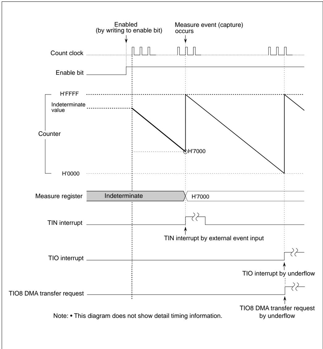
**Figure 10.4.10 Typical Operation in Measure Clear Input Mode**
