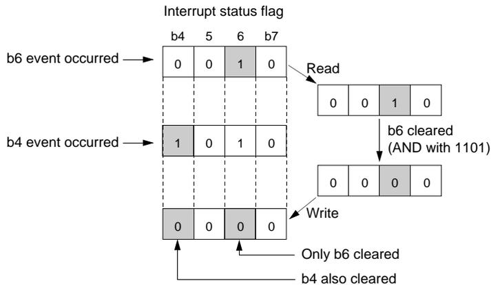
Figure 10.2.5 Example for Clearing the Interrupt Status
