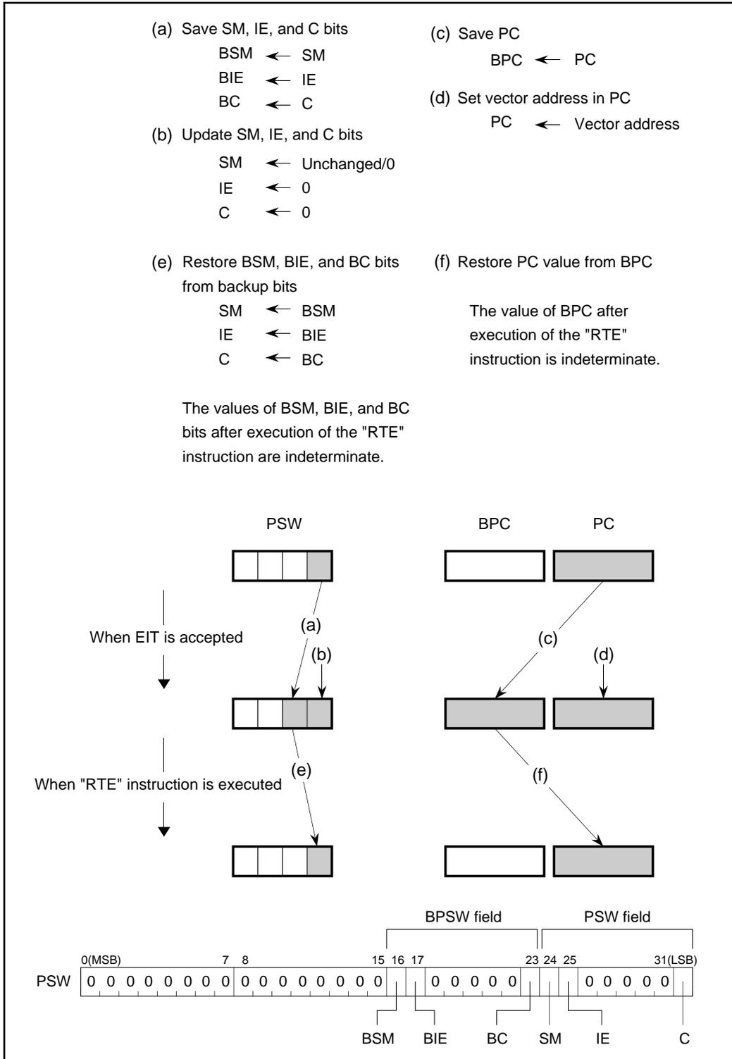
Figure 4.6.1 Saving and Restoring the PC and PSW
