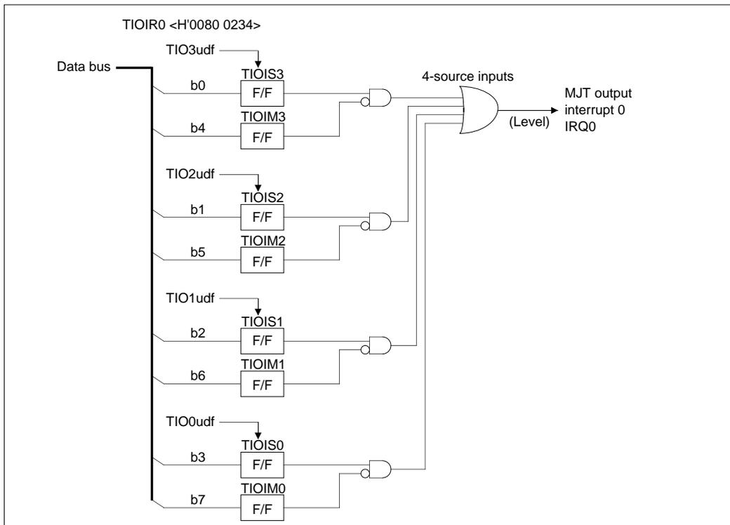
Figure 10.2.9 Block Diagram of MJT Output Interrupt 0
