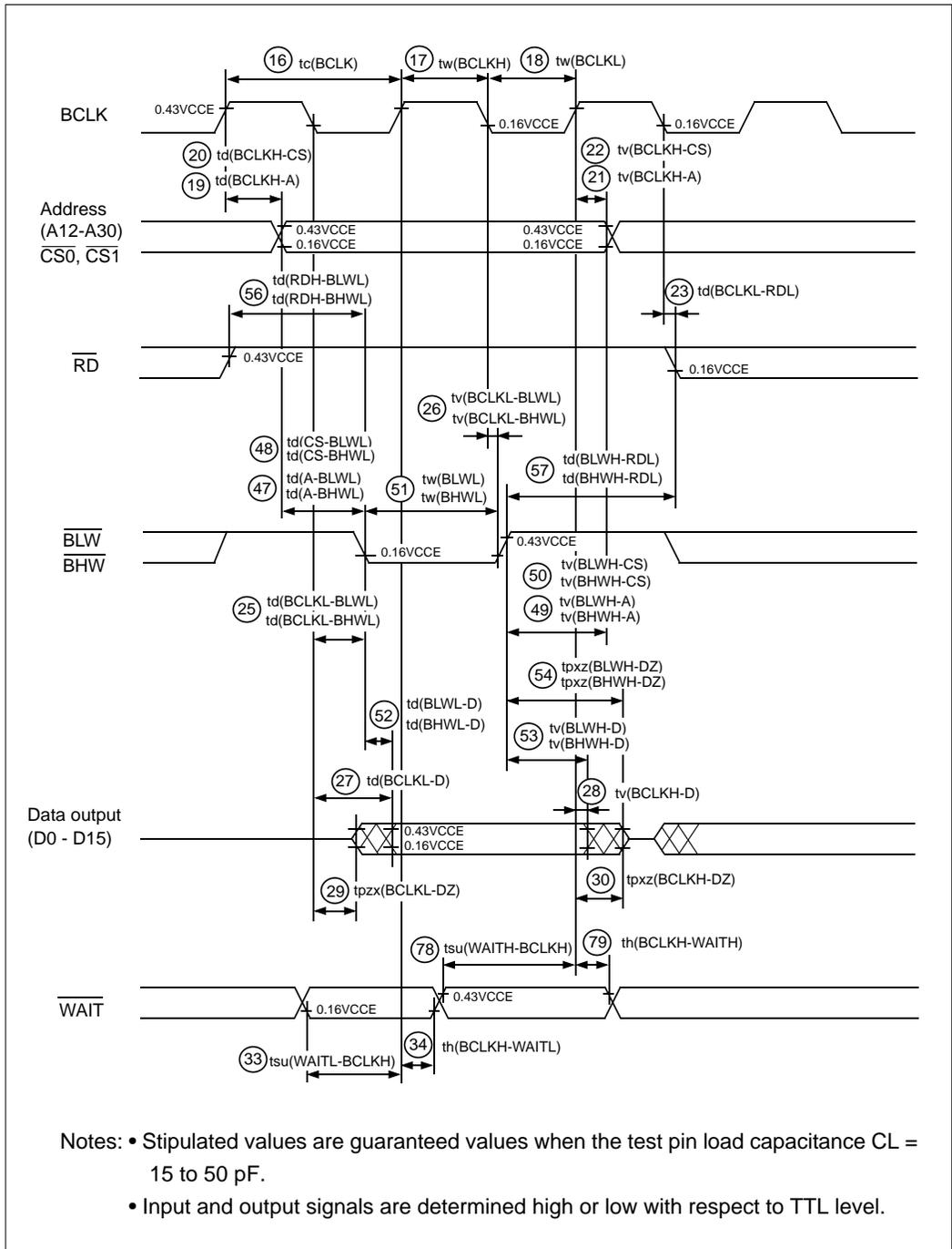
Figure 21.3.8 Write Timing
