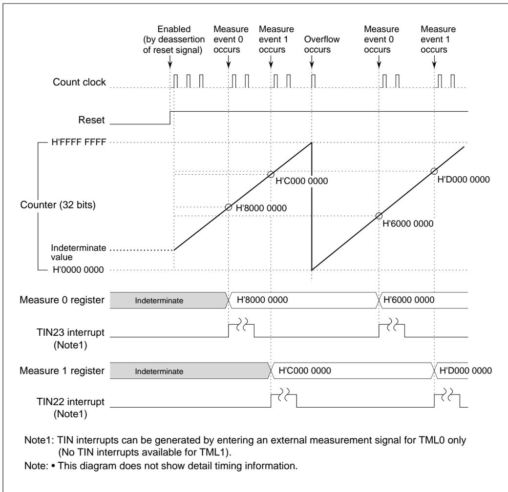
Figure 10.6.3 Typical Operation in TML Measure Input
