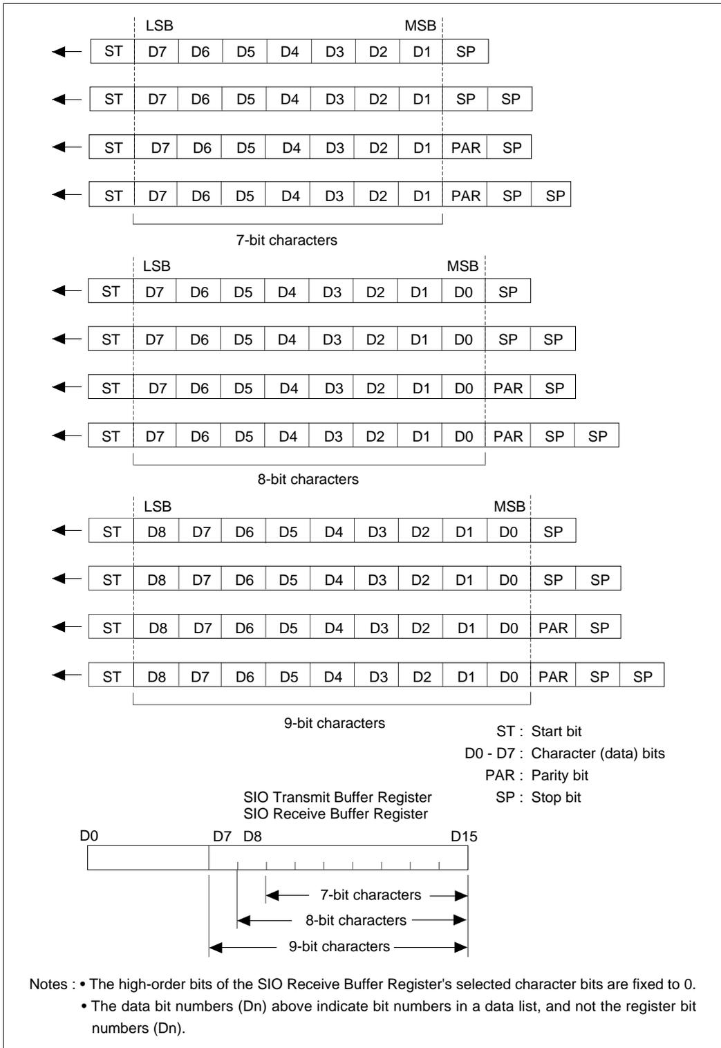
Figure 12.6.2 Selectable Data Formats during UART Mode
