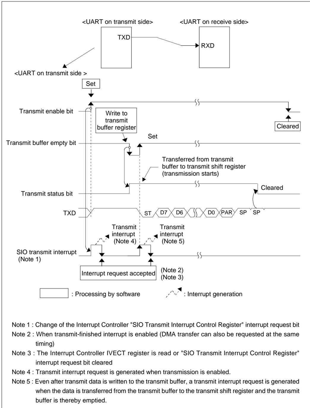
Figure 12.6.5 Example of UART Transmission (Transmitted Only Once, with Transmit Interrupt Used)
