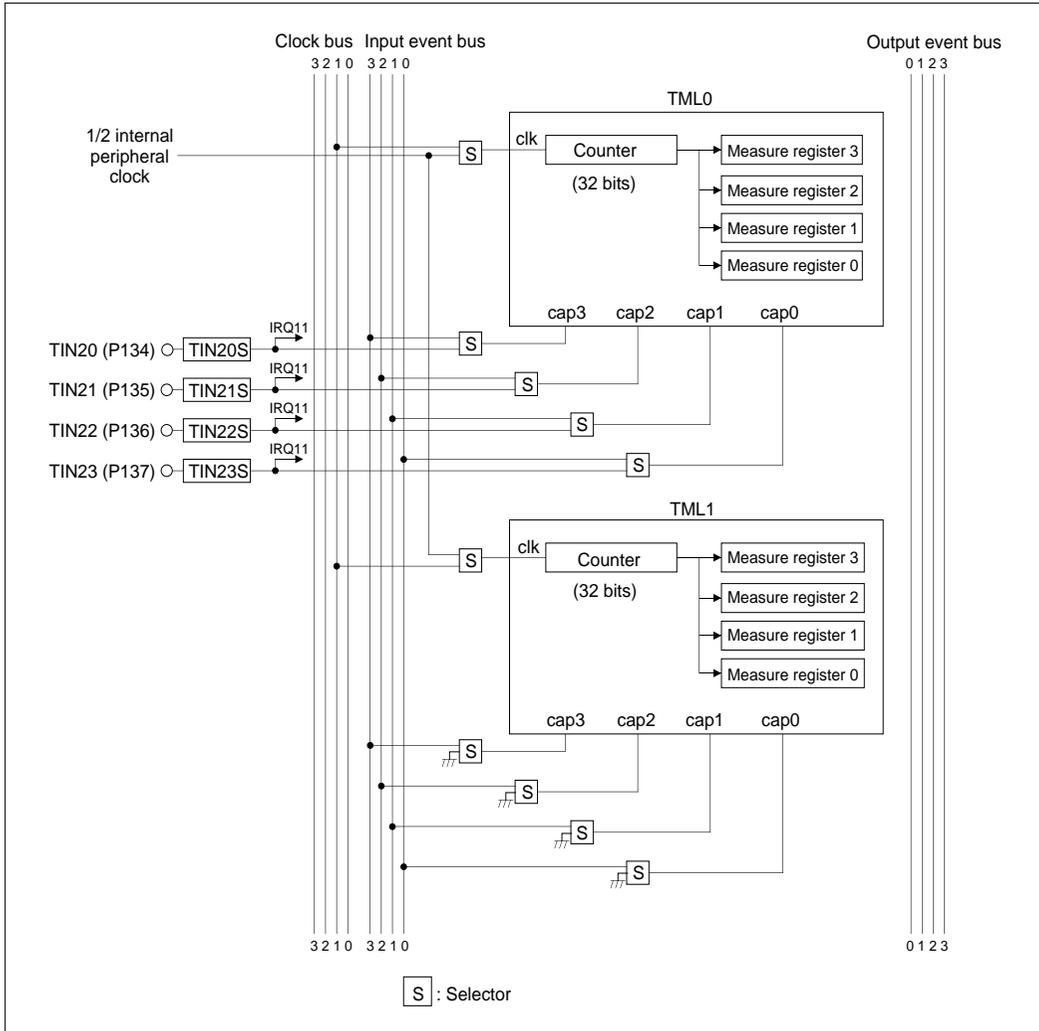
Figure 10.6.1 Block Diagram of TML (Input-related 32-bit Timer)
