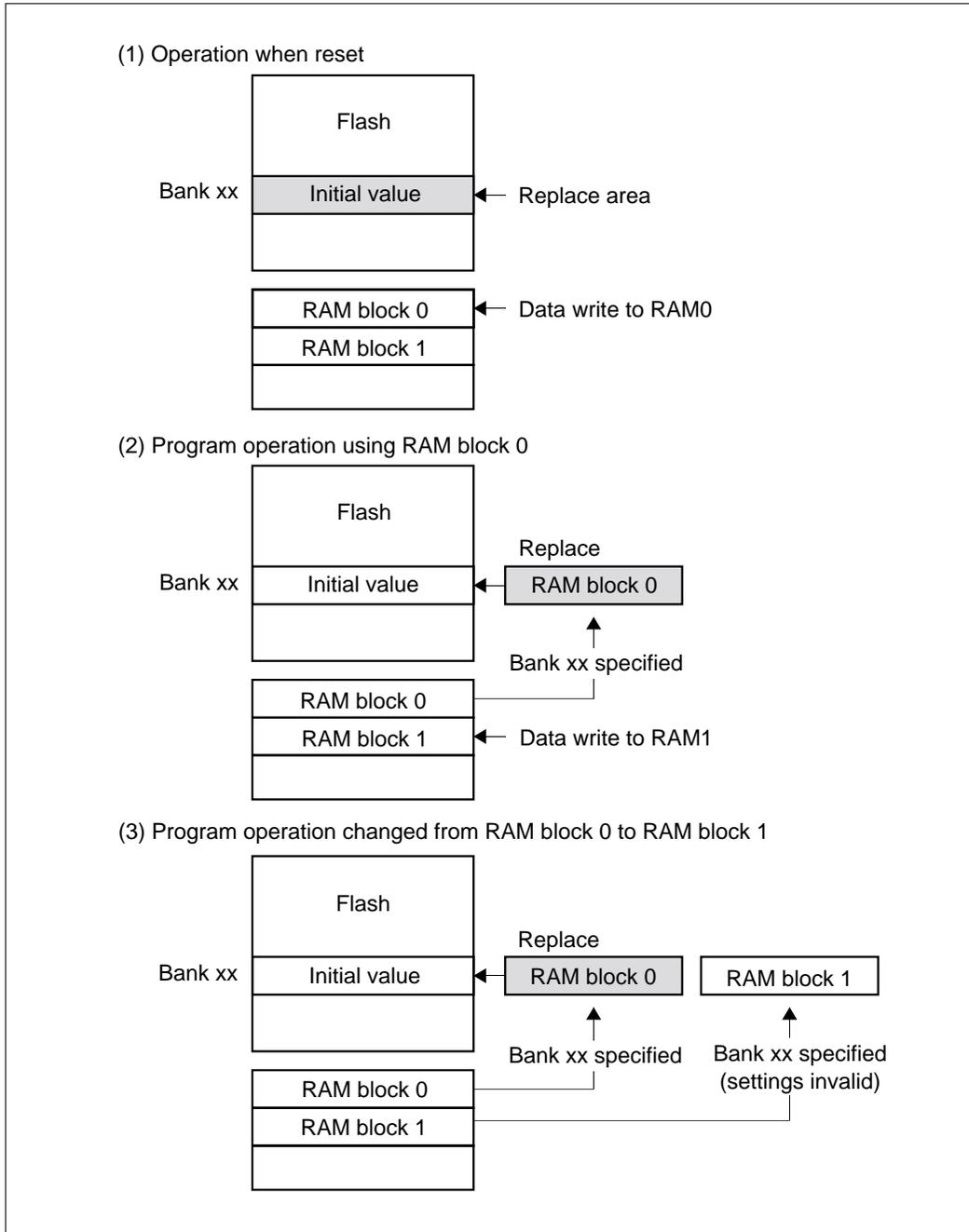
Figure 6.7.15 Application Example of Virtual Flash Emulation (1/2)
