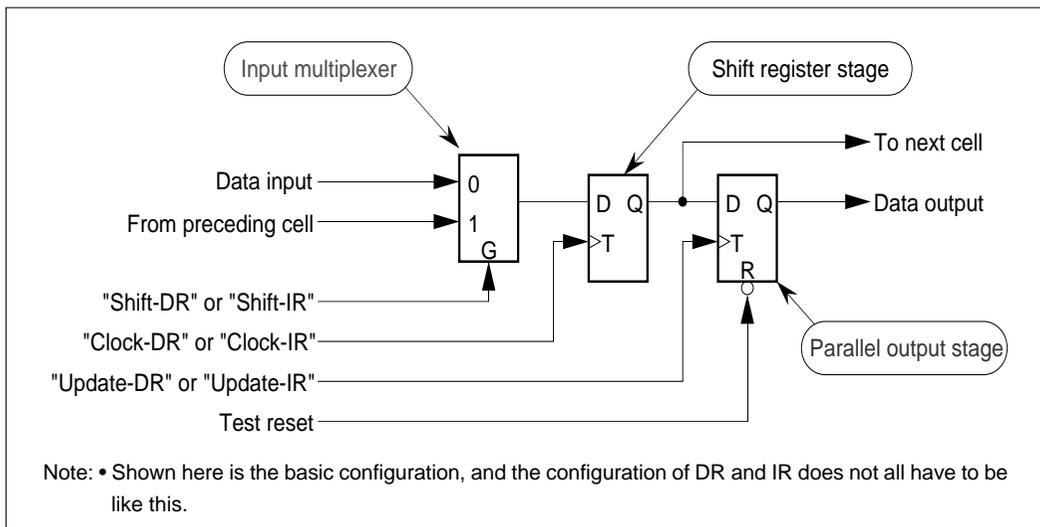
Figure 19.4.2 Basic Configuration of JTAG Related Registers
