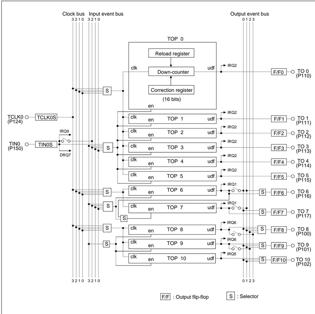
Figure 10.3.1 Block Diagram of TOP (Output-related 16-bit Timer)
