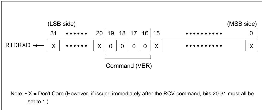
Figure 14.3.6 VER (Continuous Monitor) Command Data Format
