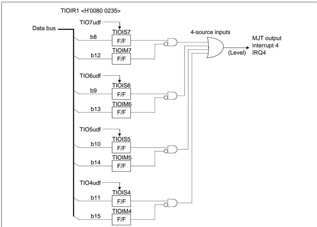
Figure 10.2.10 Block Diagram of MJT Output Interrupt 4
