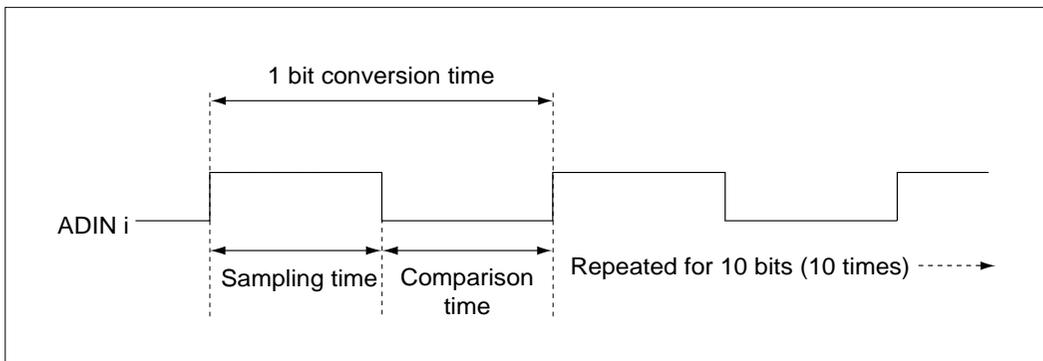
Figure A4.9.2 A-D Conversion Timing Diagram
