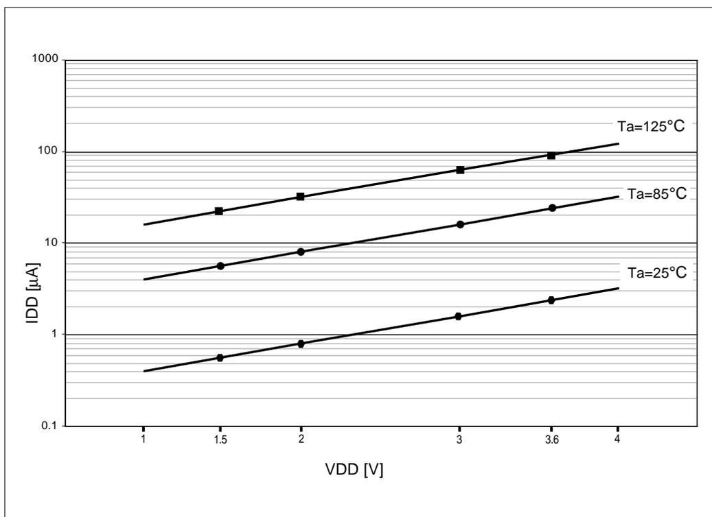
Standard sample's ICCI-3V temperature characteristics (when operating: f = 8 MHz, 10 MHz)
