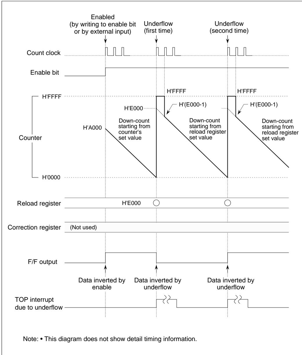
Figure 10.3.21 Typical Operation in TOP Continuous Output Mode
