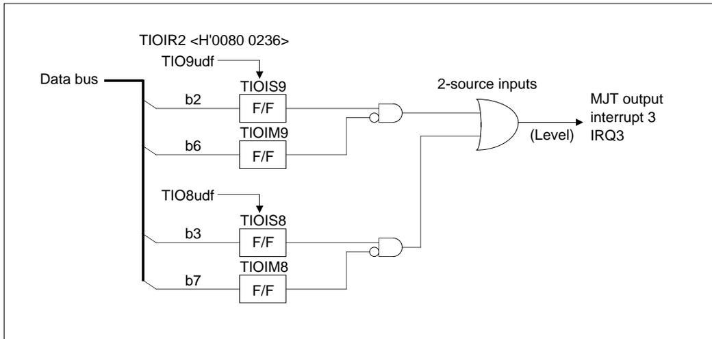
Figure 10.2.11 Block Diagram of MJT Output Interrupt 3
