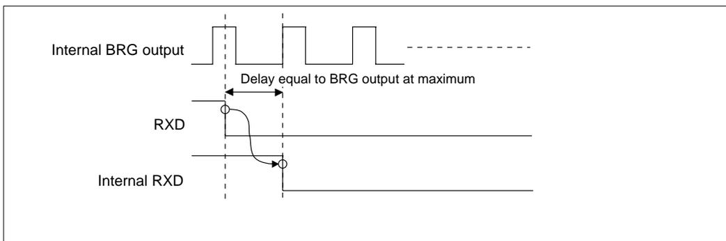
Figure 12.7.7 Delay when Receiving
