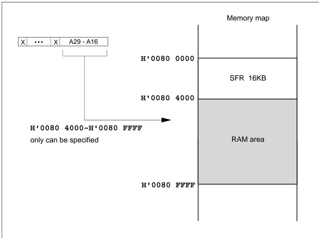
Figure 14.3.12 Method for Setting Addresses in Real-Time Debugger
