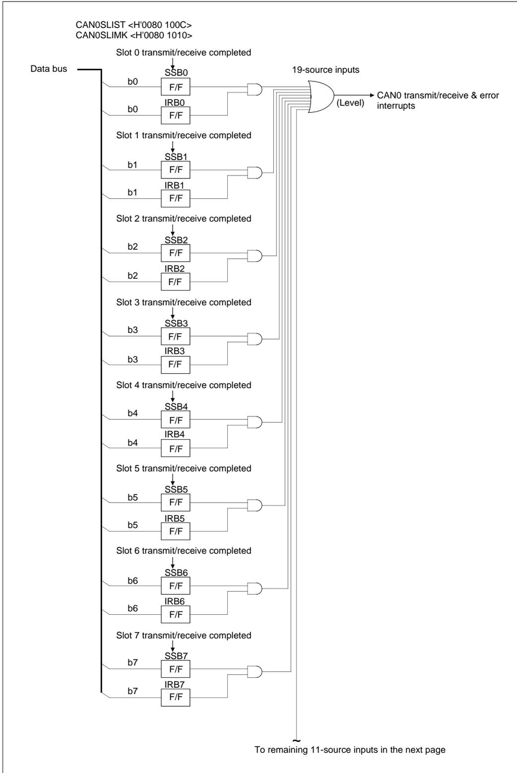
Figure 13.2.5 Block Diagram of CAN0 Group Interrupts (1/3)
