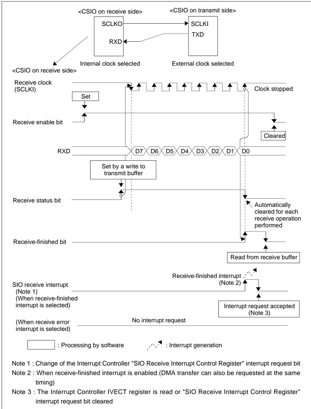
Figure 12.4.3 Example of CSIO Reception (When Received Normally)
