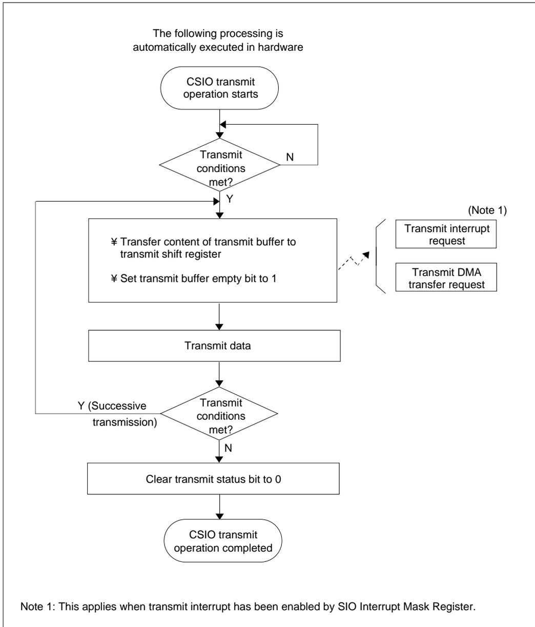
Figure 12.3.2 Transmit Operation during CSIO Mode (Hardware Processing)
