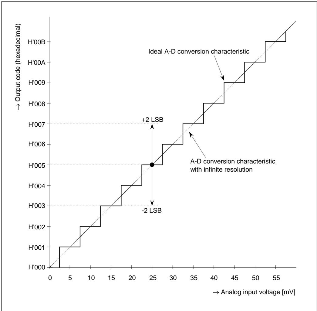
Figure 11.3.6 Absolute Accuracy of an A-D Converter
