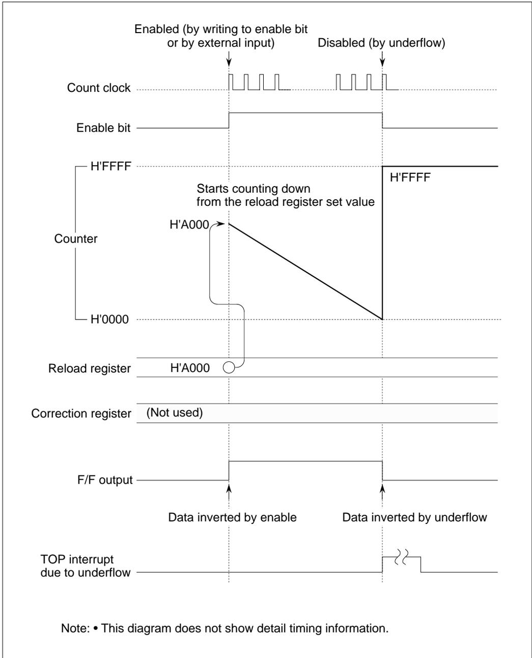
Figure 10.3.11 Typical Operation in TOP Single-shot Output Mode
