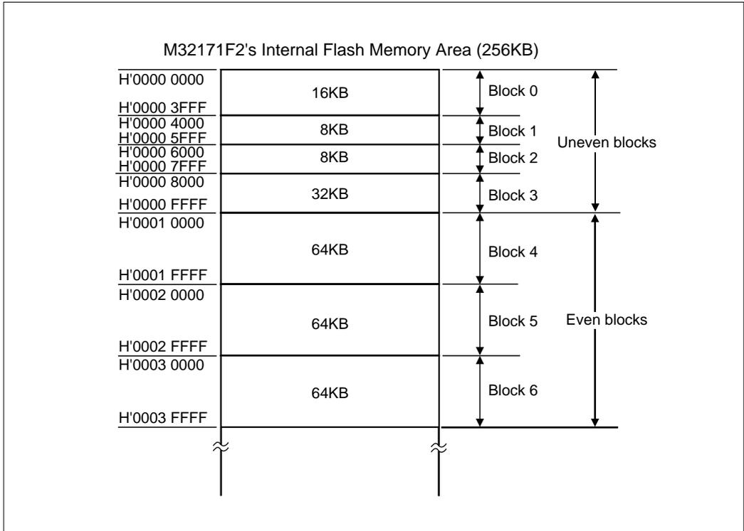
Figure 6.5.9 Block Configuration of the M32171F2 Flash Memory
