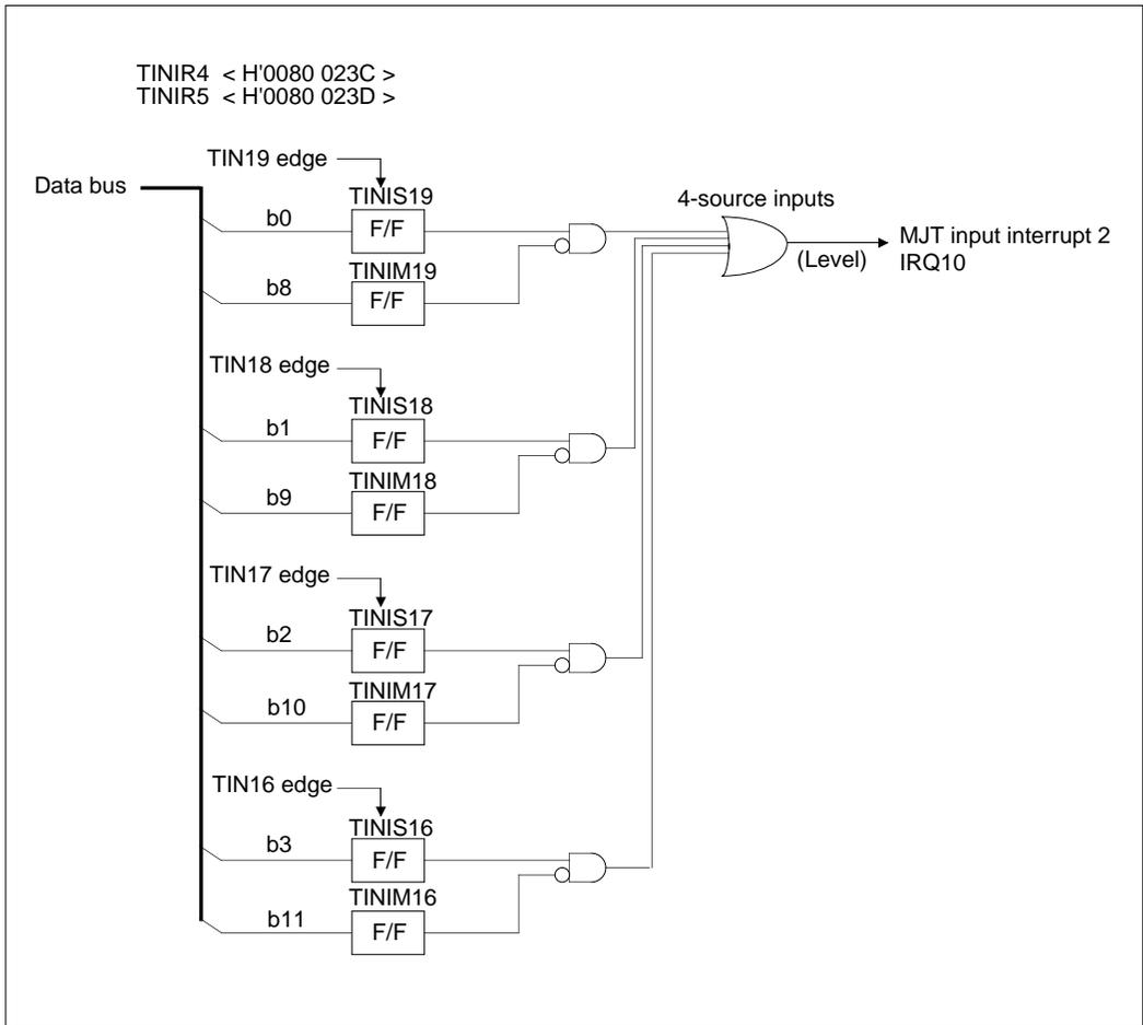
Figure 10.2.15 Block Diagram of MJT Input Interrupt 2
