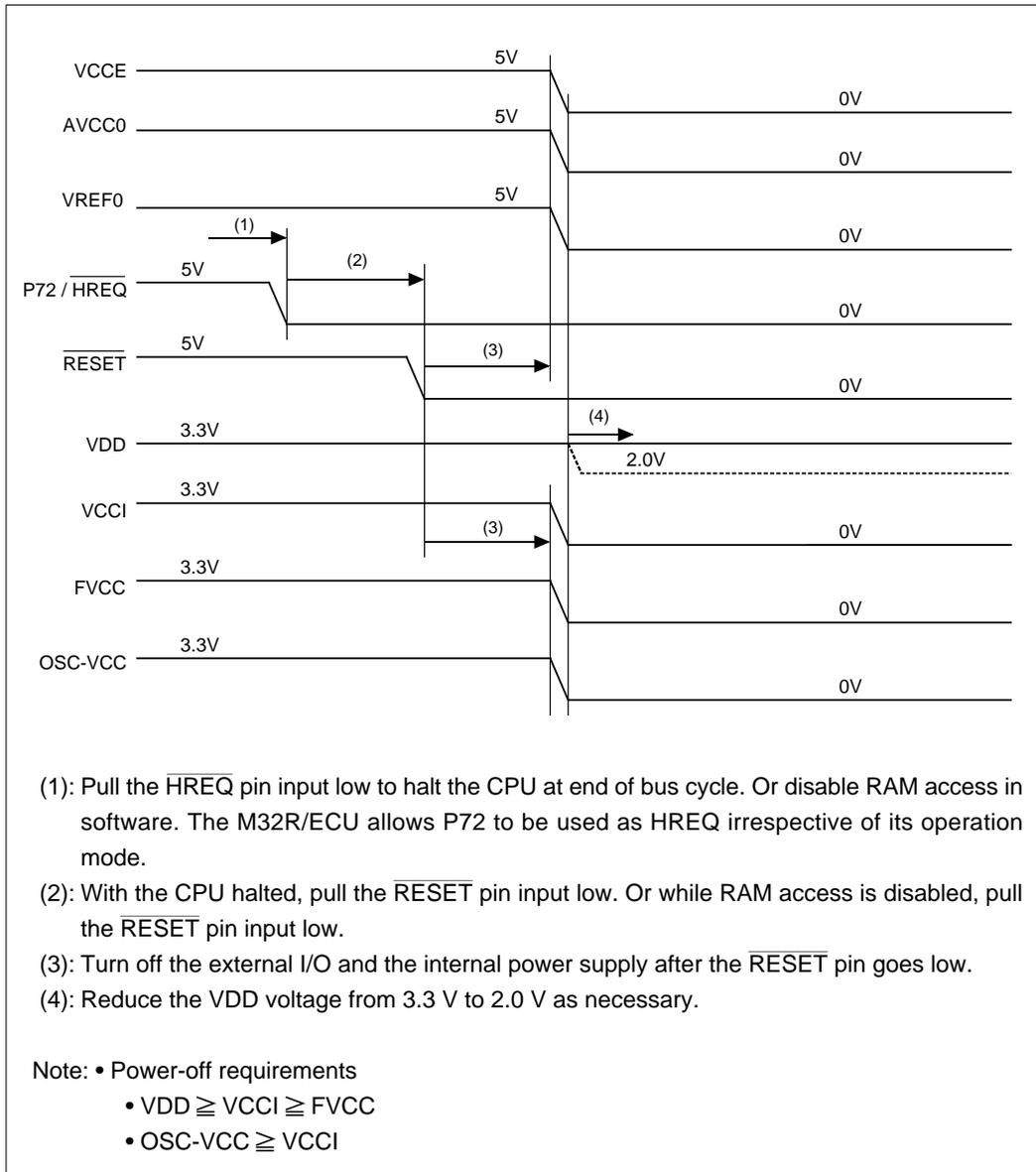
Figure 20.3.3 Power-off Sequence When Using RAM Backup(when external I/O power supply = 5 V)
