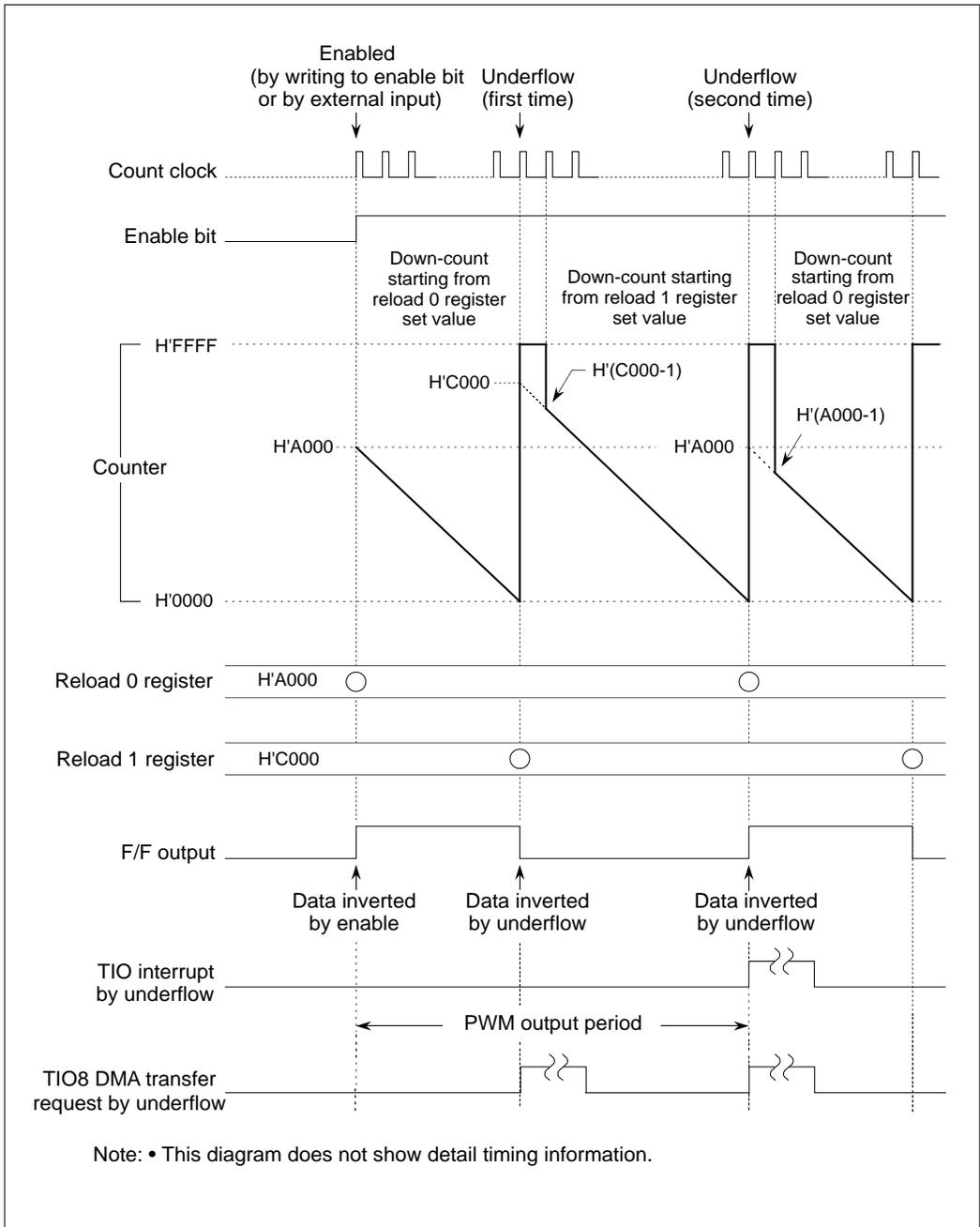
Figure 10.4.12 Typical Operation in PWM Output Mode
