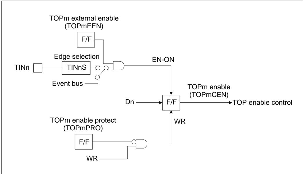
Figure 10.3.9 Configuration of the TOP Enable Circuit
