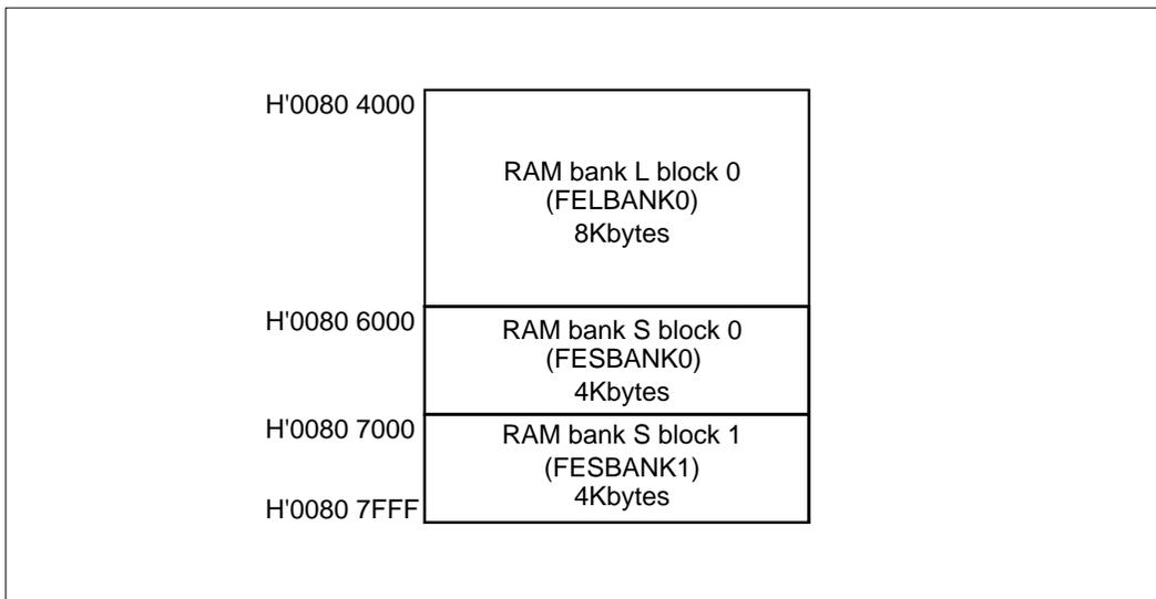
Figure 6.7.1 Internal RAM Bank Configuration of the 32171
