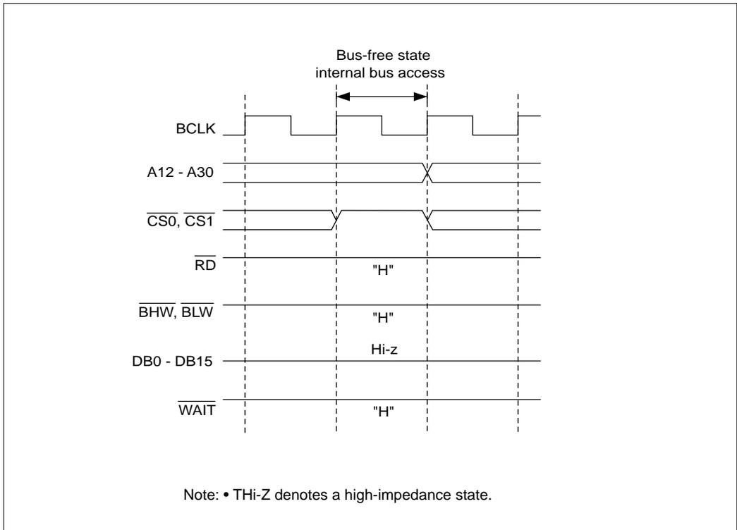
Figure 15.2.1 Internal Bus Access during Bus Free State
