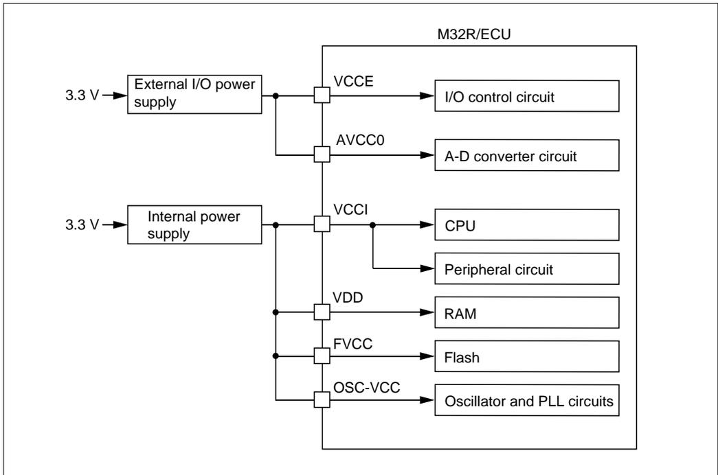
Figure 20.3.6 Microcomputer Ready to Run State 2
