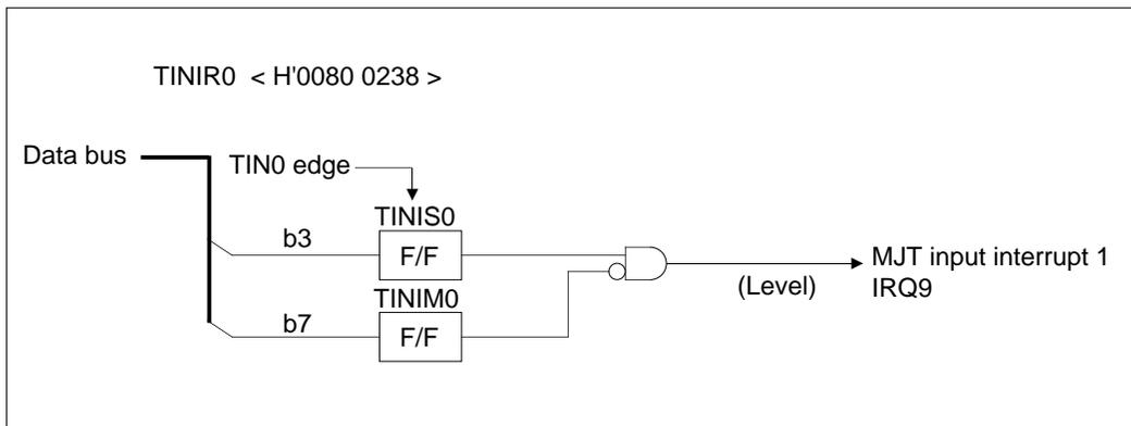
Figure 10.2.13 Block Diagram of MJT Input Interrupt 1
