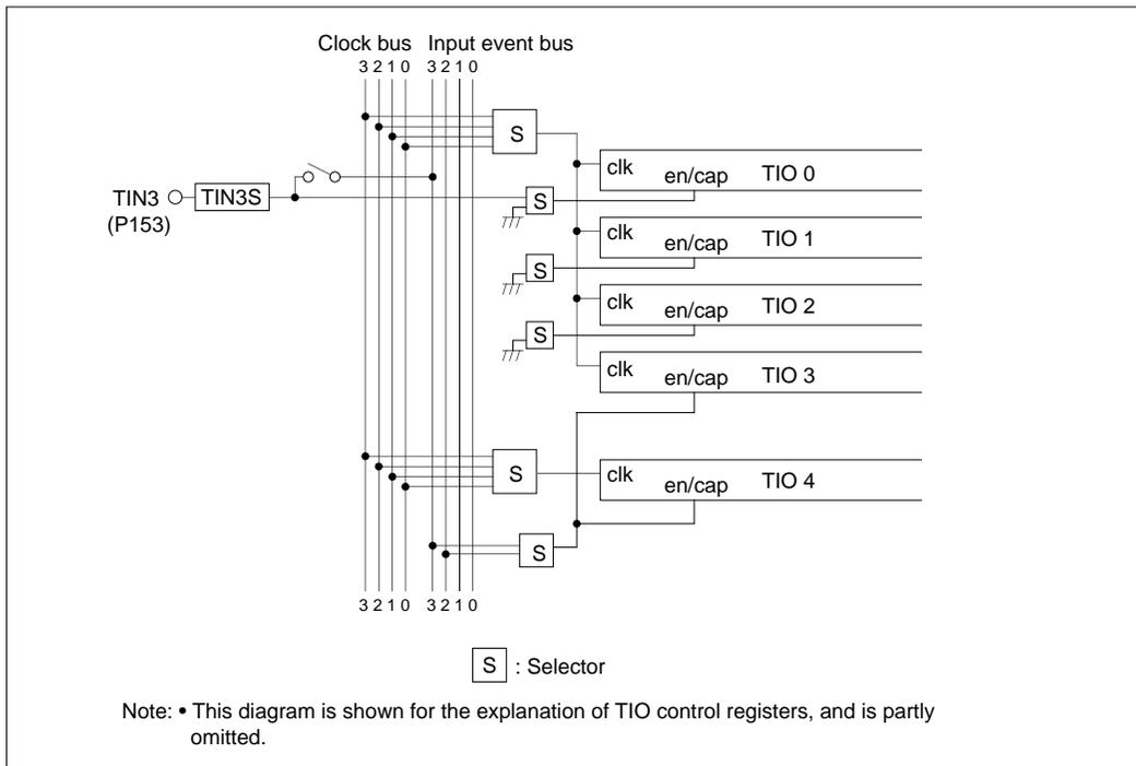
**Figure 10.4.6 Outline Diagram of TIO0-4 Clock/Enable Inputs**
