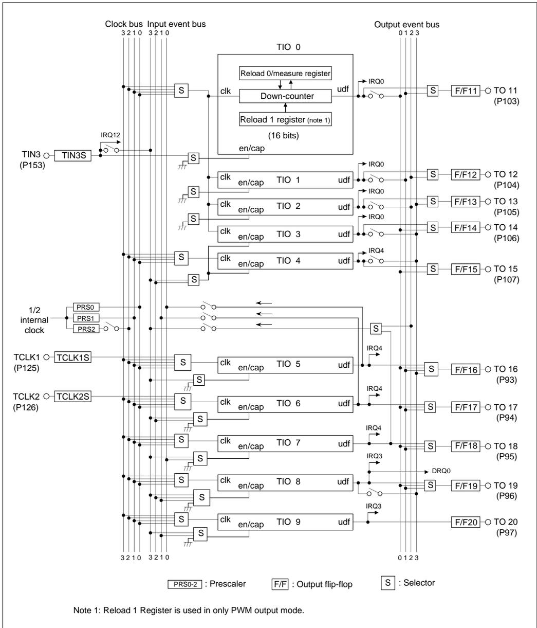
Figure 10.4.1 Block Diagram of TIO (Input/Output-related 16-bit Timer)
