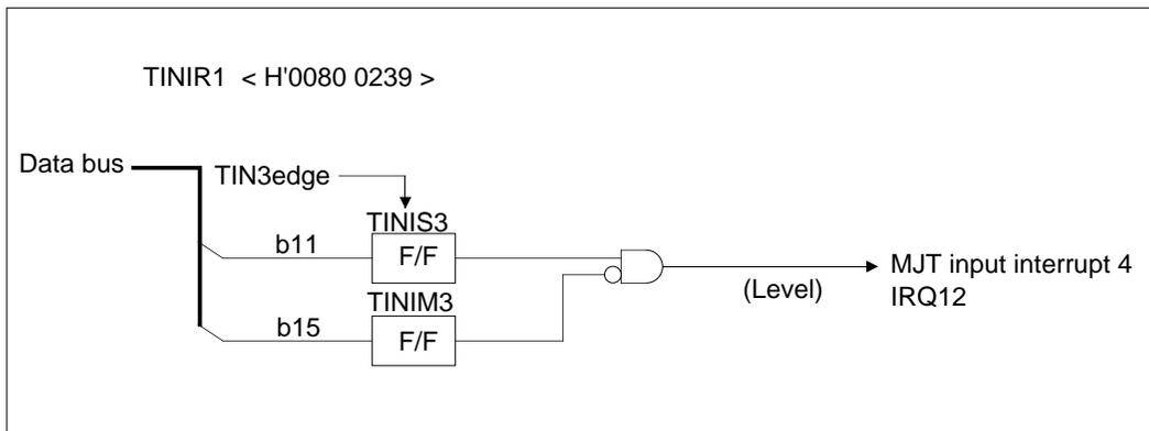
Figure 10.2.14 Block Diagram of MJT Input Interrupt 4
