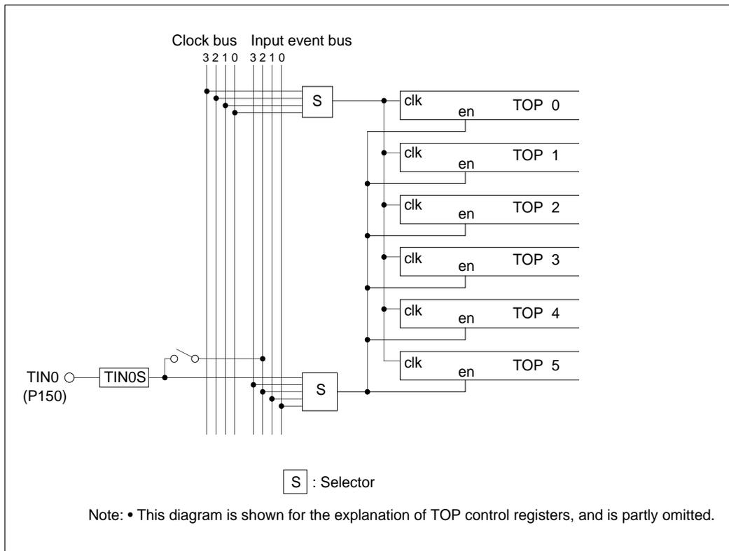
Figure 10.3.6 Outline Diagram of TOP0-5 Clock/Enable Inputs
