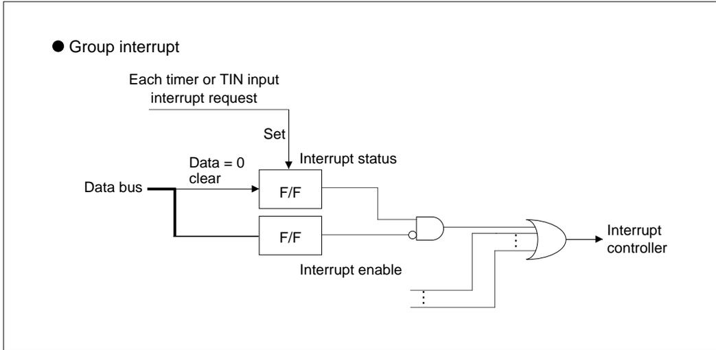
**Figure 10.2.4** Interrupt Status Register and Mask Register
