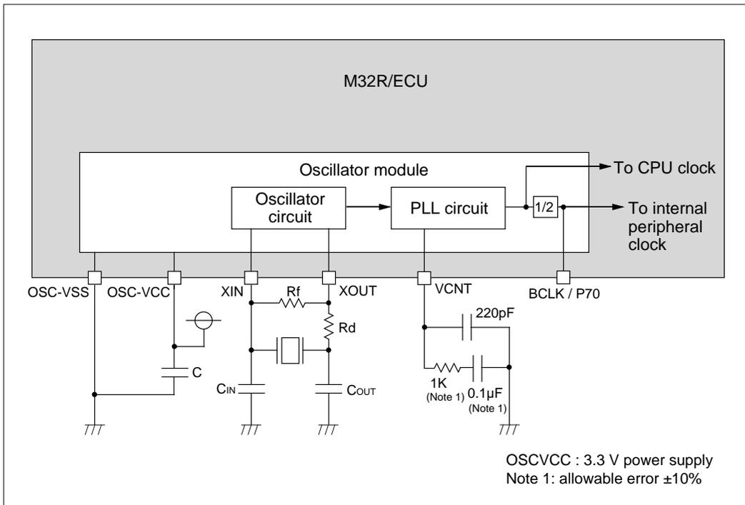
**Figure 18.1.1 Example of a System Clock Generating Circuit**
