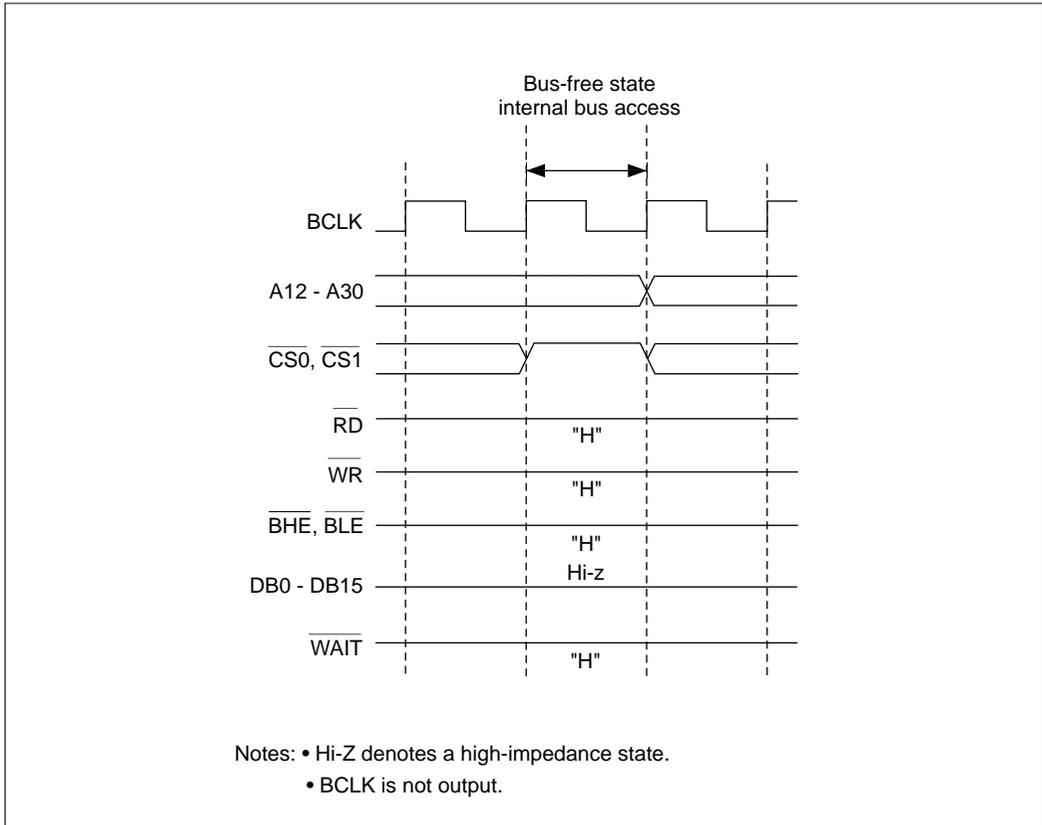
**Figure 16.3.8 Internal Bus Access during Bus Free State**
