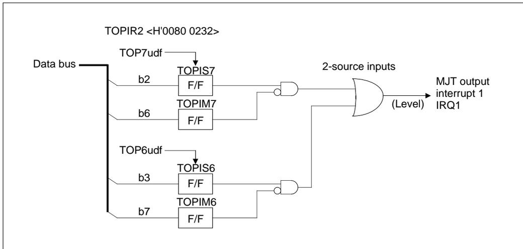
Figure 10.2.7 Block Diagram of MJT Output Interrupt 1
