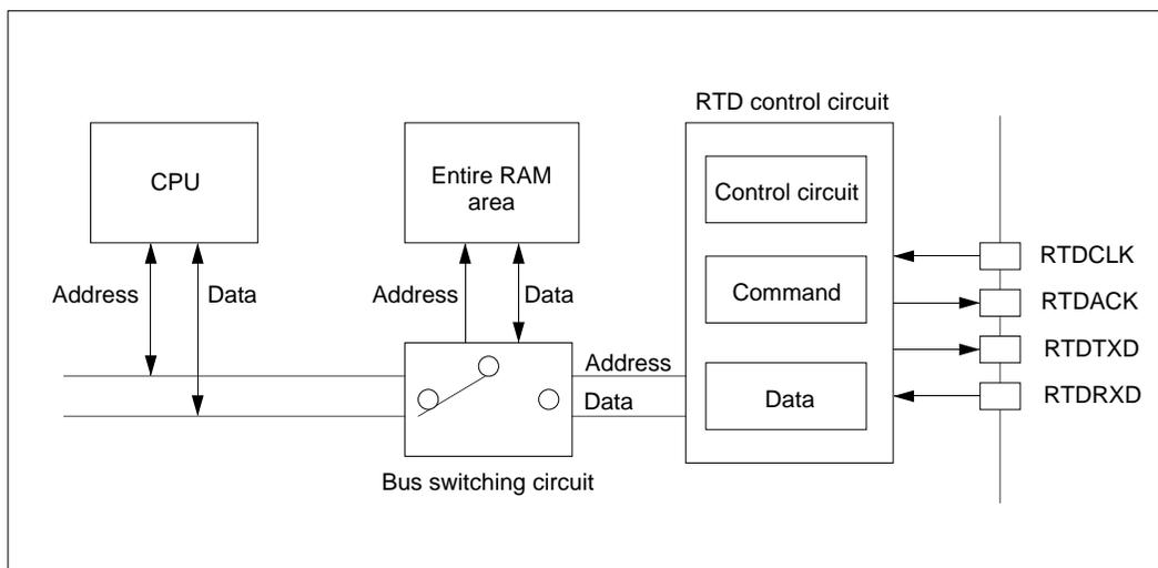
**Figure 14.1.1 Block Diagram of the Real-Time Debugger (RTD)**
