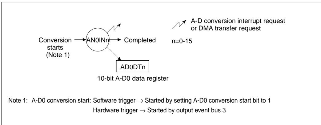
**Figure 11.1.2 Operation in Single Mode (A-D Conversion)**
