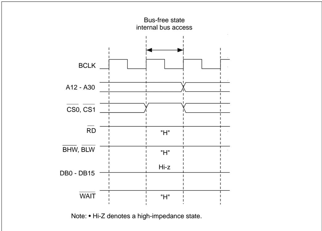
**Figure 16.3.1 Internal Bus Access during Bus Free State**
