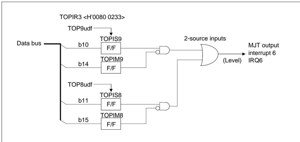
Figure 10.2.8 Block Diagram of MJT Output Interrupt 6
