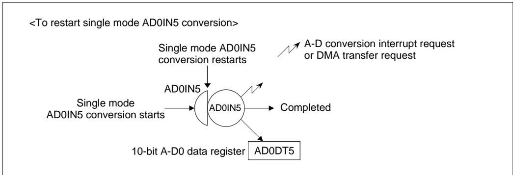
**Figure 11.1.8 Restarting Conversion during Single Mode Operation**
