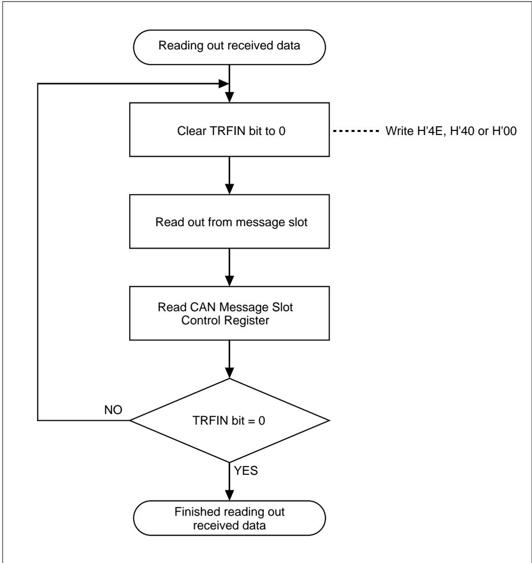
Figure 13.6.3 Procedure for Reading Out Received Data
