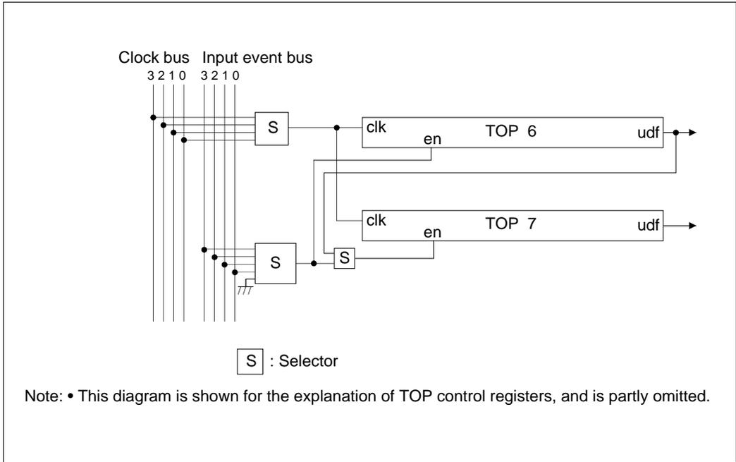
Figure 10.3.7 Outline Diagram of TOP6, TOP7 Clock/Enable Inputs
