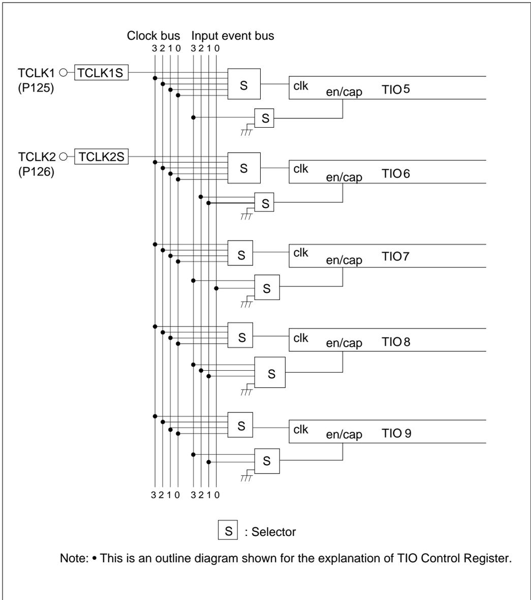
Figure 10.4.7 Outline Diagram of TIO5-9 Clock/Enable Inputs
