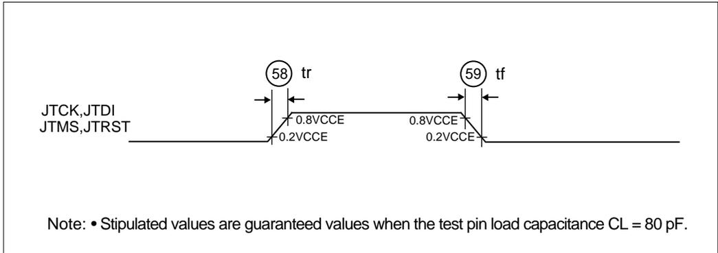
Figure 21.3.11 Input Transition Time on JTAG pins
