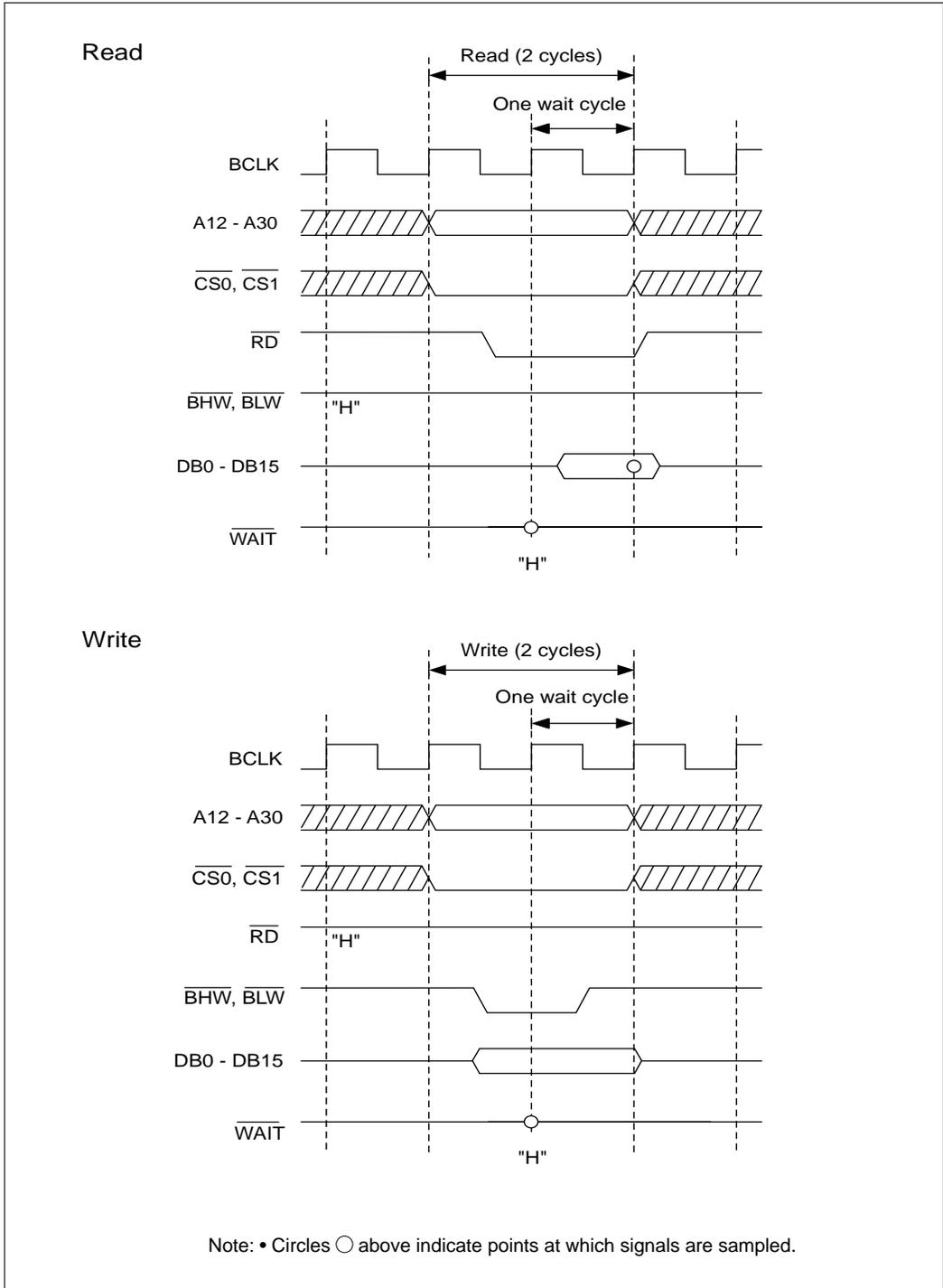
Figure 15.2.2 Read/Write Timing (for Shortest-case External Access)
