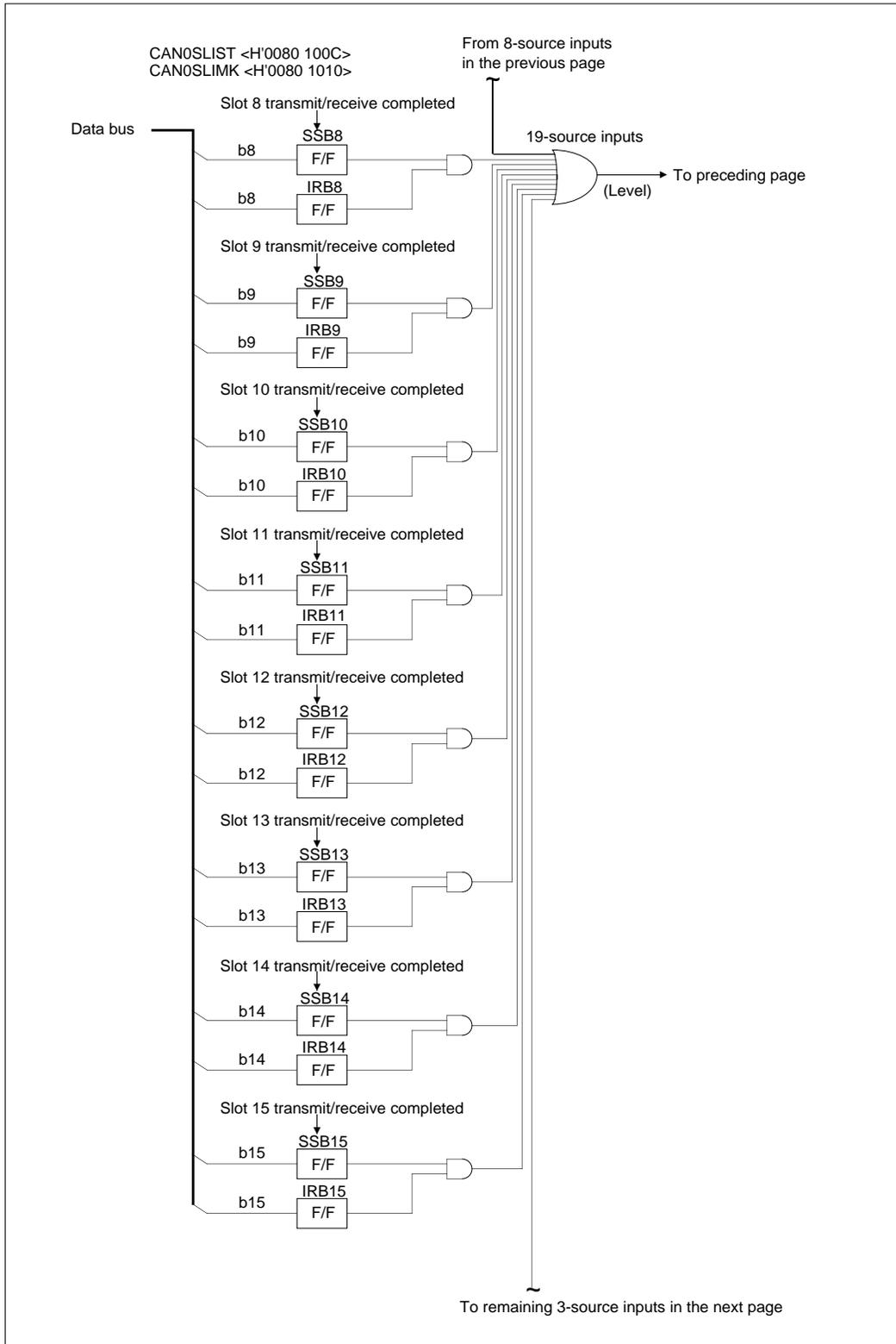
Figure 13.2.6 Block Diagram of CAN0 Group Interrupts (2/3)
