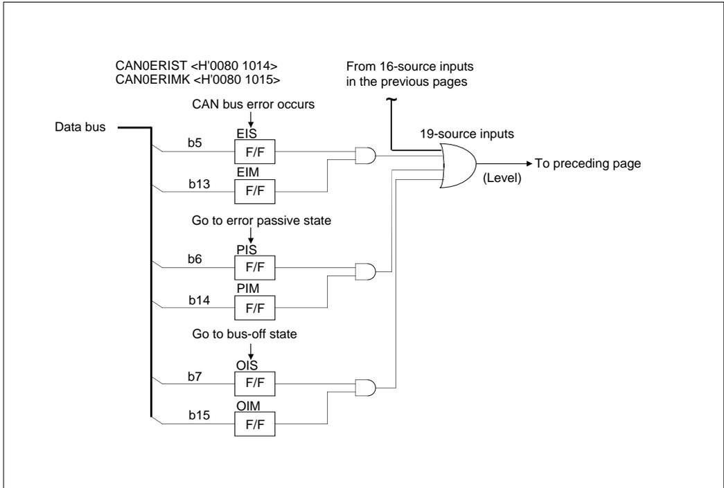
Figure 13.2.7 Block Diagram of CAN0 Group Interrupts (3/3)
