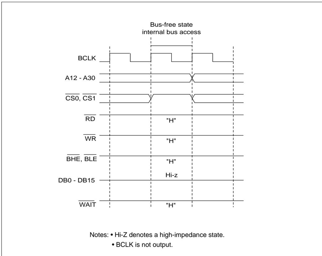
Figure 15.2.4 Internal Bus Access during Bus Free State
