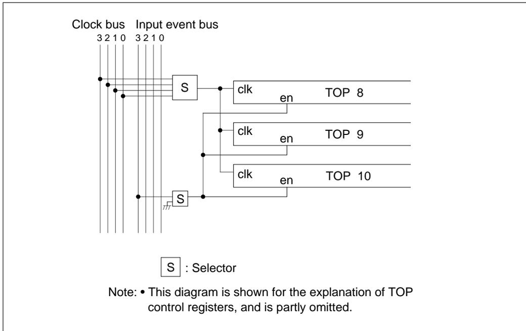
**Figure 10.3.8 Outline Diagram of TOP8-10 Clock/Enable Inputs**
