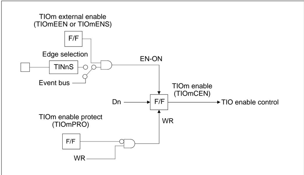
Figure 10.4.8 Configuration of the TIO Enable Circuit
