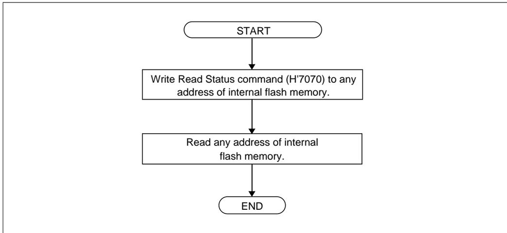
**Figure 6.5.15 Read Status Register**
