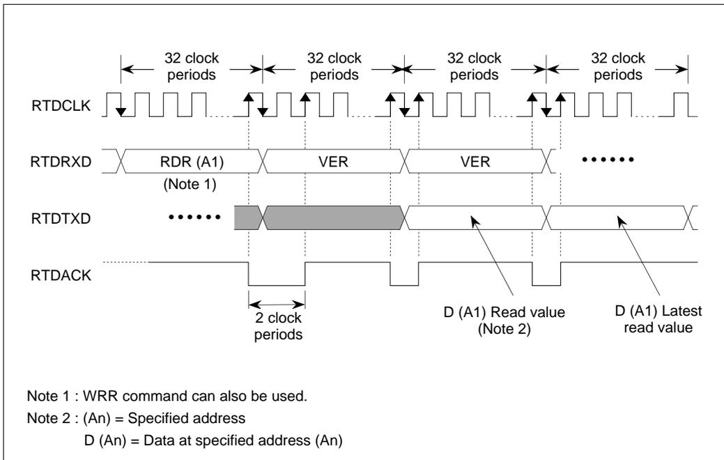
Figure 14.3.7 Operation of the VER (Continuous Monitor) Command
