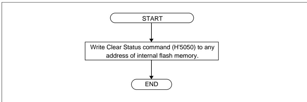
**Figure 6.5.16 Clear Status Register**
