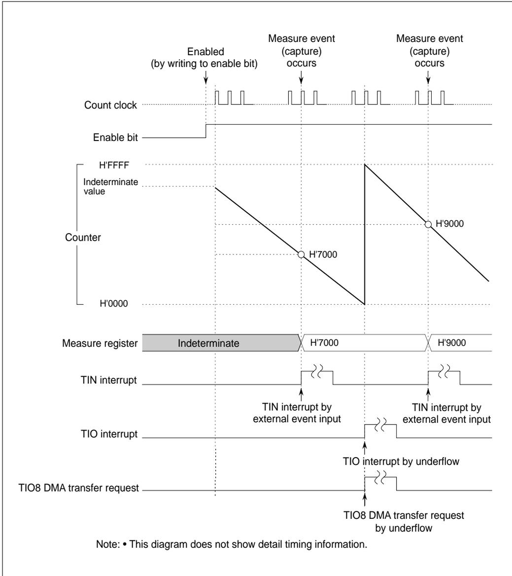
Figure 10.4.9 Typical Operation in Measure Free-run Input Mode
