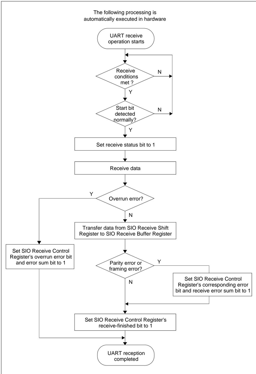
Figure 12.7.2 Receive Operation during UART Mode (Hardware Processing)
