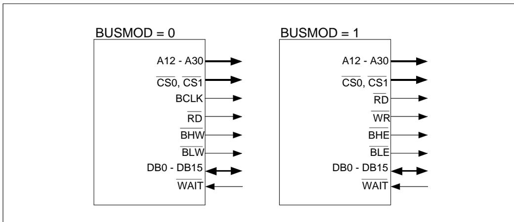
Figure 15.1.1 Pin Function when Bus Modes are Changed
