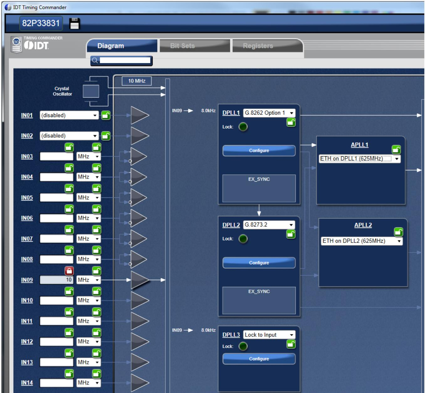
To associate an input clock (i.e., IN09) with a sync signal (such as 1PPS), click on the Input Buffer of IN09 (the triangle symbol following frequency entry box), a sub-configuration window for IN09 is shown below. In the window, IN10 is selected as sync signal.
