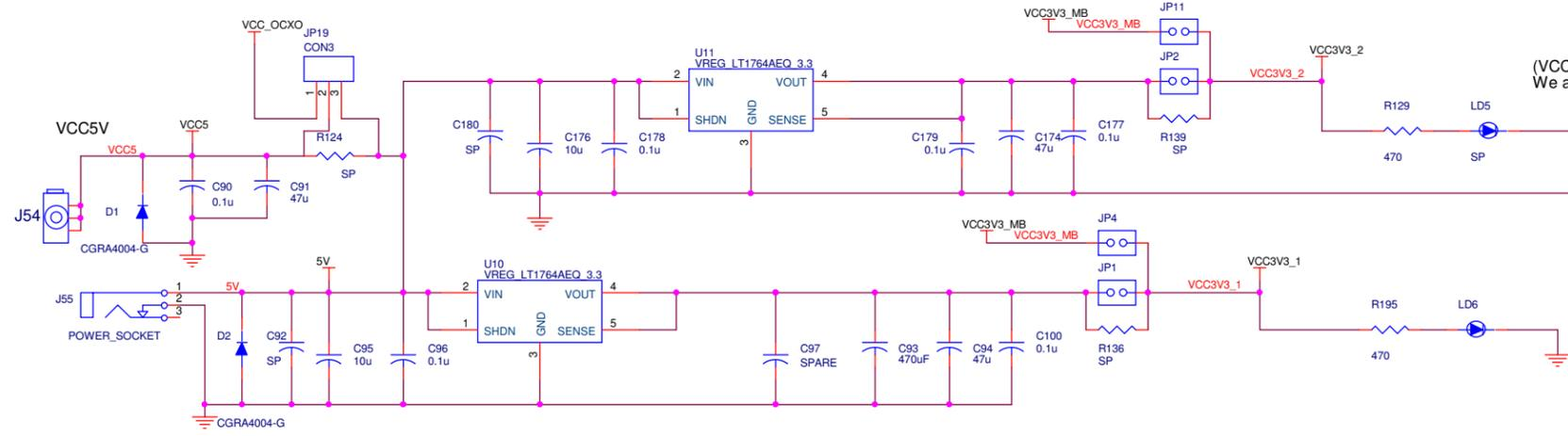
(VCC3V3\_1 is used for the 82V33910 DUT and VCC3V3\_2 is for the rest of the board circuits. We are not suggesting a dedicated LDO for the 82V33910 with this reference design, this is just convenient for the test.)
