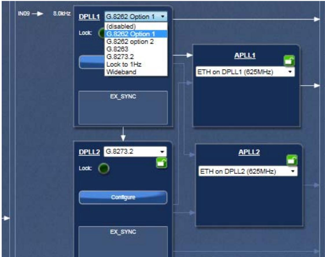
Click “Configure” button to open up configuration window for respective DPLL for additional or customized configuration. There are pull-down items for each configuration parameter. For example, in “Operation Mode” section, you can select:
