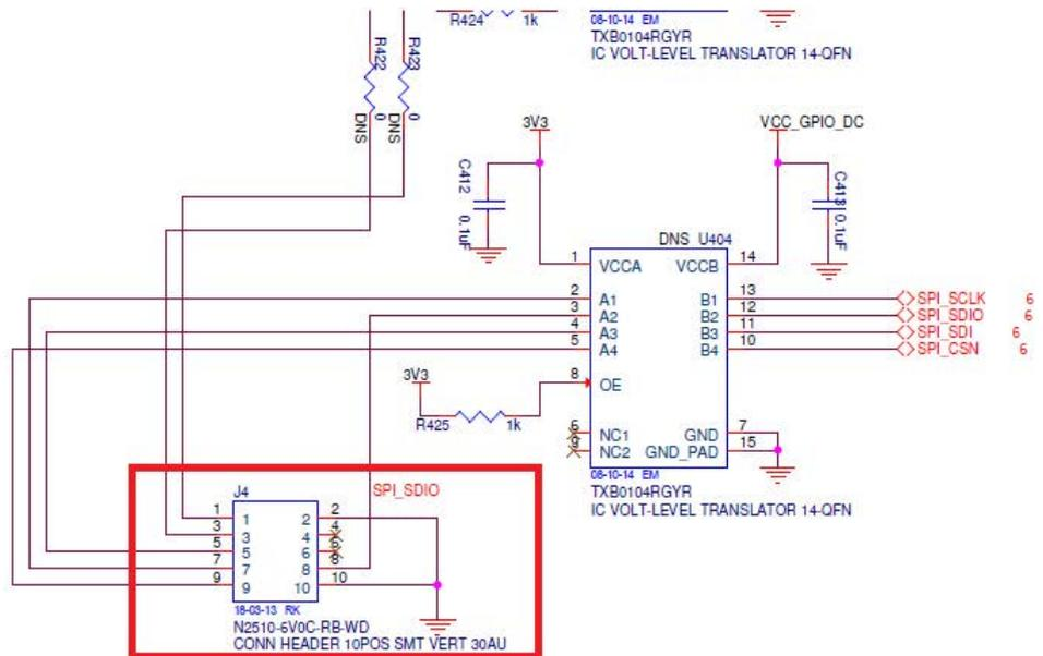
Figure 5. J4 Connector with Aardvark Color-coded Wire Connections
