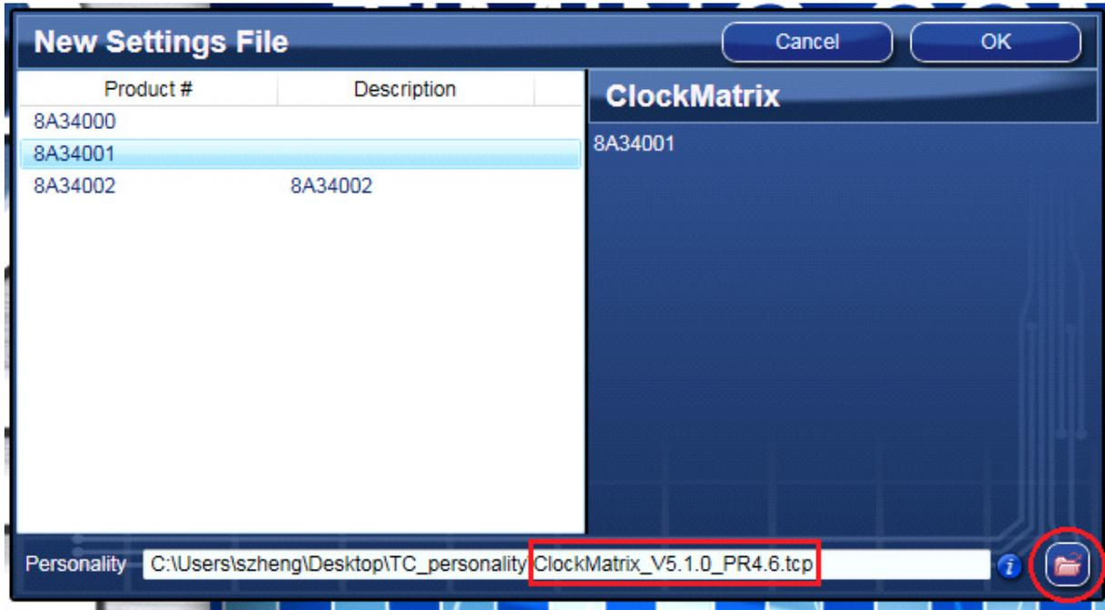
Figure 9. Selecting 8A34001 using Personality File v4.6
