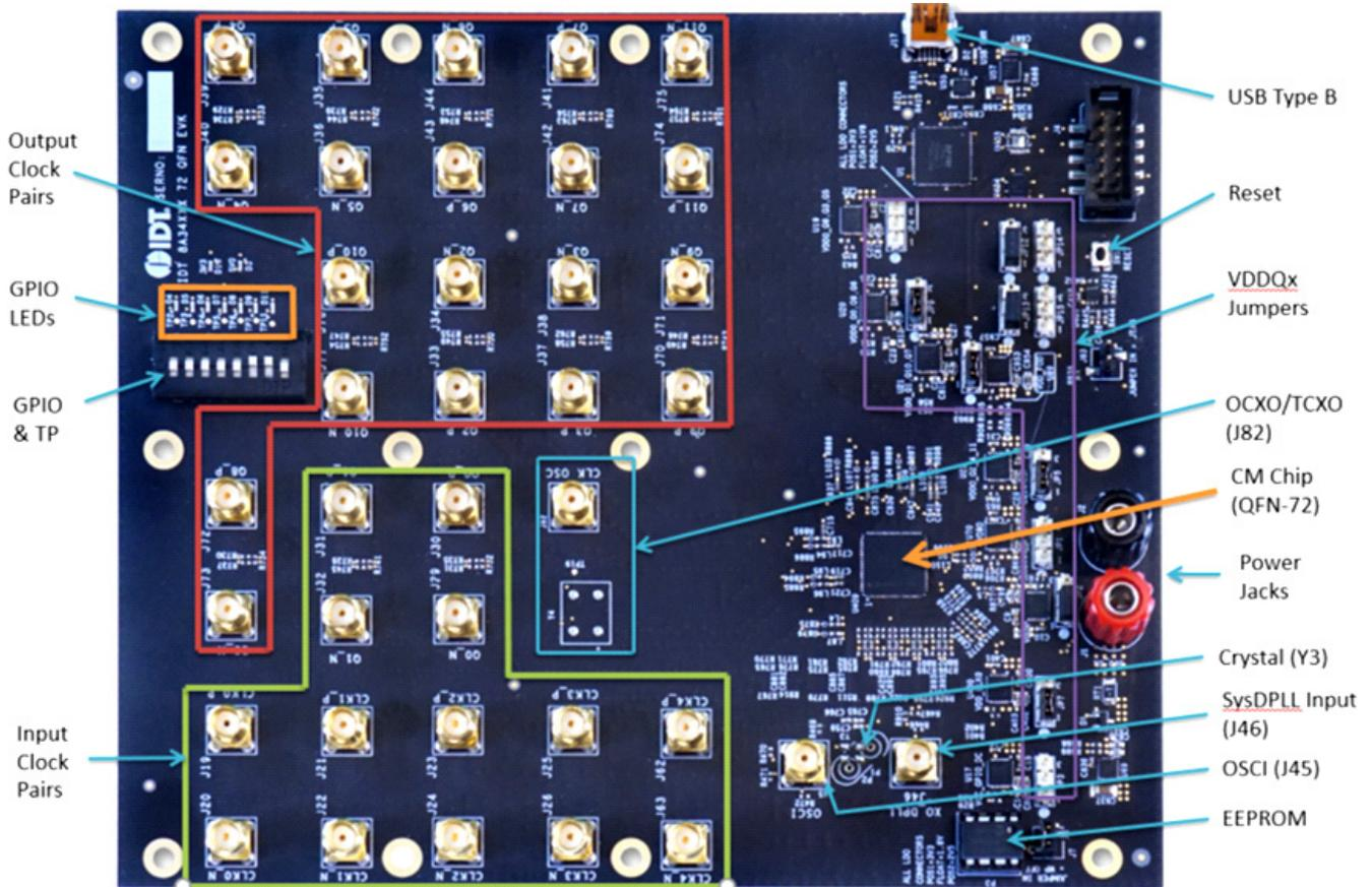
Figure 2. 8A3xxxx 72QFN Evaluation Board – Detailed
