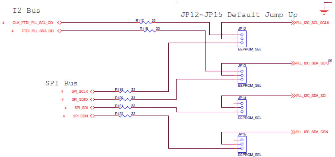
Figure 6. Schematic View of JP12 to JP15
